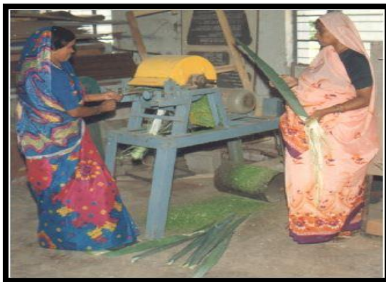
Fiber extraction using Raspador Machine
