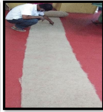
Layering of the nonwoven sheet
