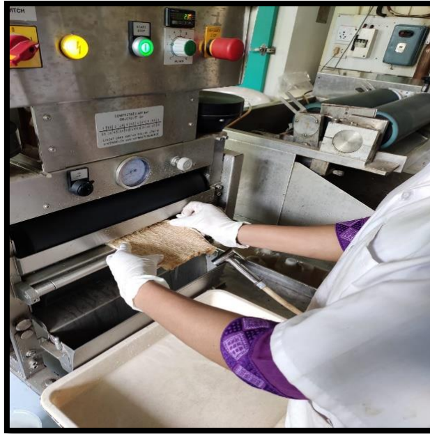
Plate 3.28: Resin application using padding mangle
