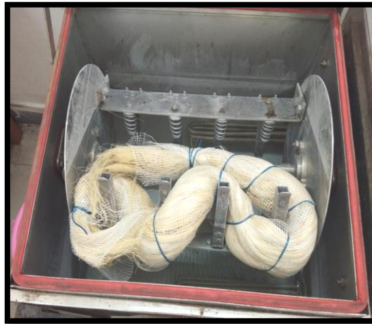
Plate 3.8: Bundle of fibers arranged on the rotor panel of launder-O-meter
