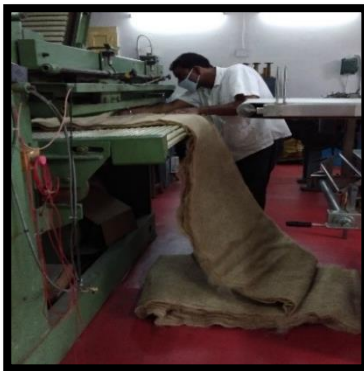
Insertion of layered sheet in needle punch machine
