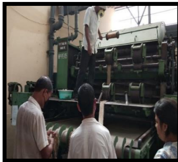
Bundled fibers converted into carded sheet on flax carding machine
