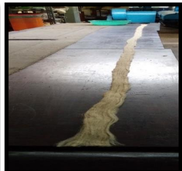
Layering of sliver for yarn preparation
