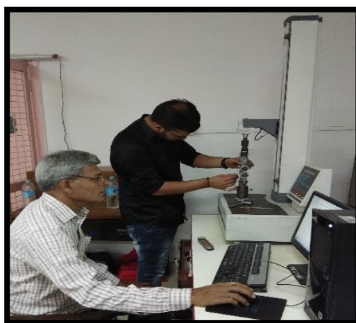
Plate 3.9: Lloyd Instron Tensile Testing Instrument
