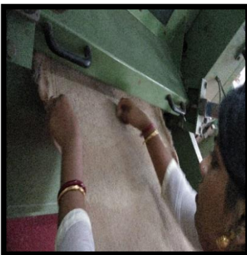
Winding of Nonwoven cloth beam
