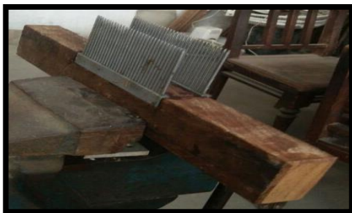
Plate 3.2: Fabricated Combing Tool
