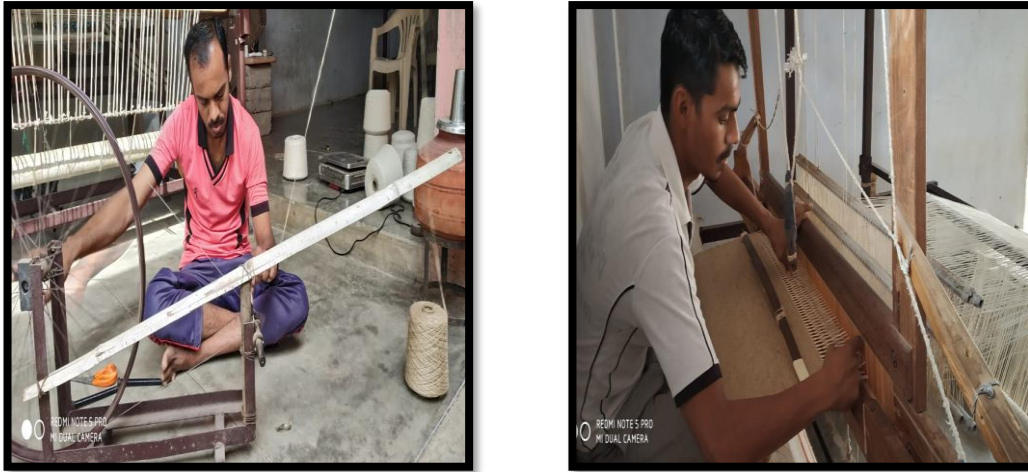
Plate 3.21: Yarn winding and fabric preparation on handloom
