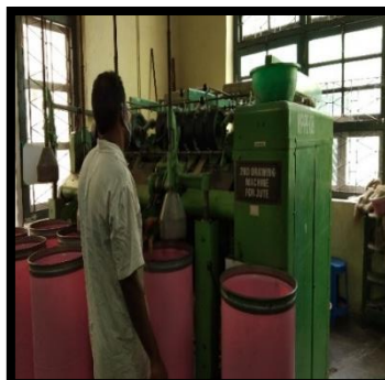
Sliver preparation on Jute drawing machine
