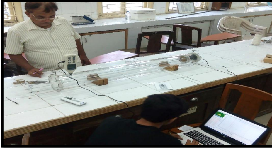
Plate 3.27: Fabricated Sound Absorbing testing instrument
