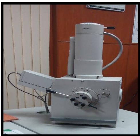
Plate 3.10: Scanning Electronic Microscopy instrument (SEM)
