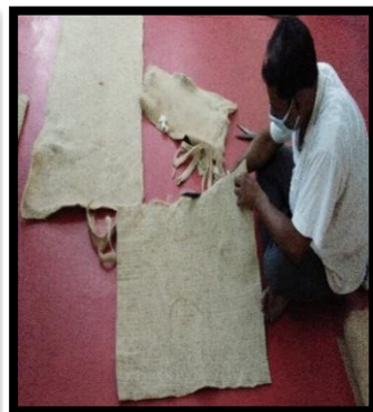
Edge finishing of Nonwoven sample
