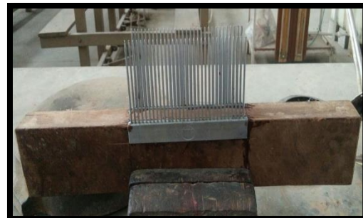
Plate 3.2: Fabricated Combing Tool
