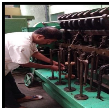
Sliver preparation on Jute drawing machine
