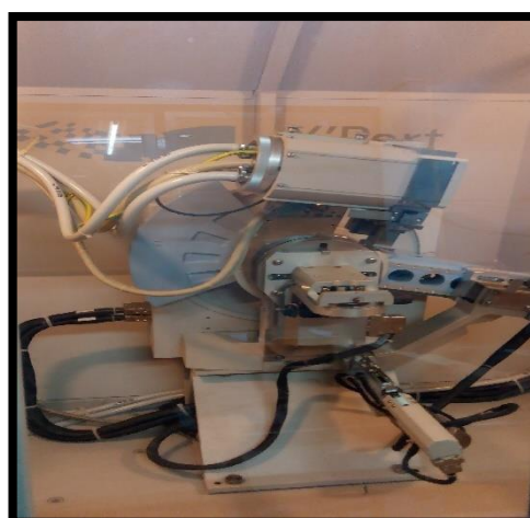
Plate 3.13: X-ray diffraction instrument (XRD)
