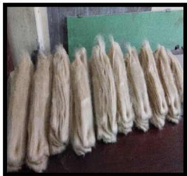
Bundles of carded fibers for converting into sliver
