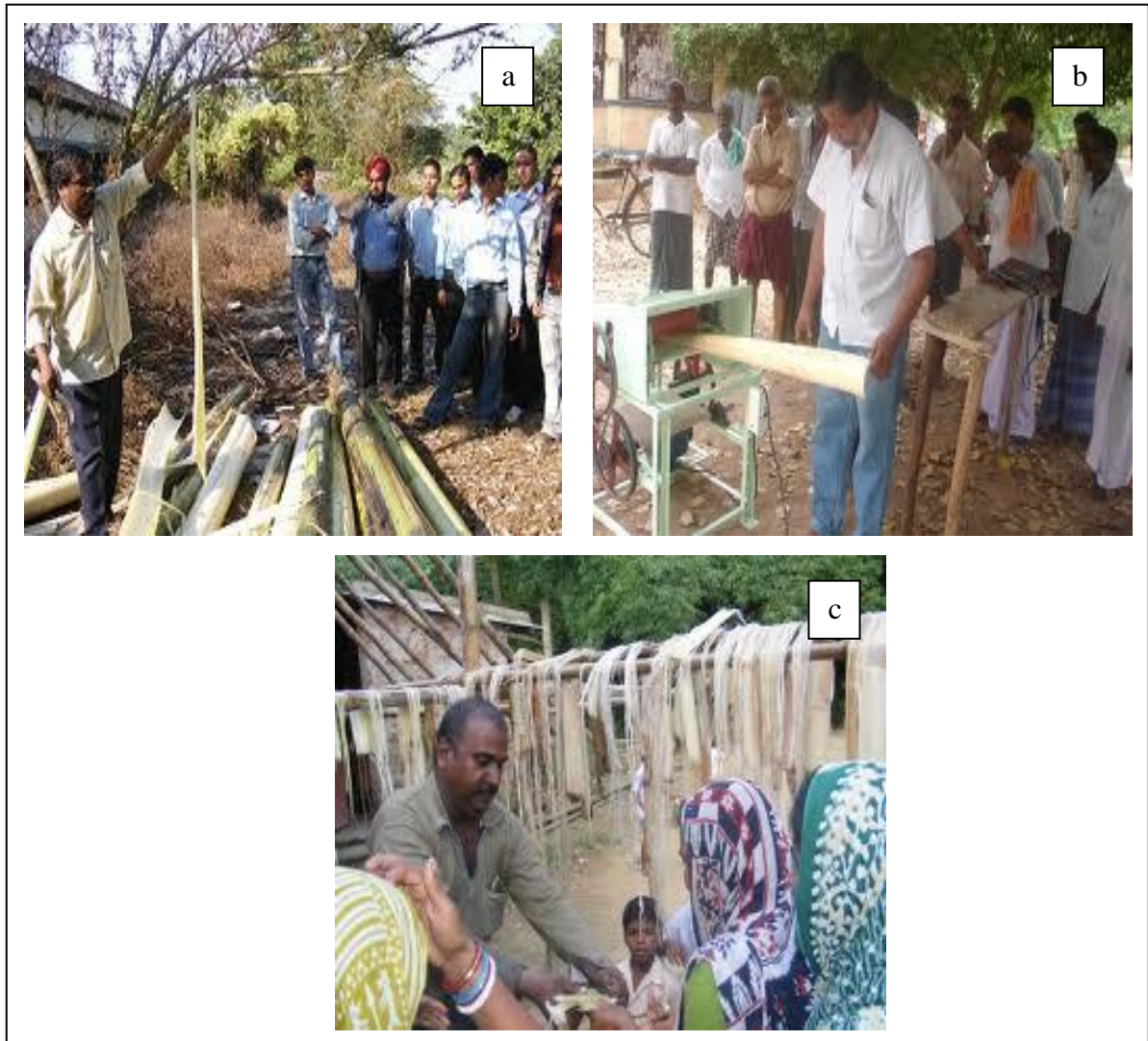
Plate 2.2: Mechanical extraction of banana fibers a) Tuxing b) Stripping c) Drying
