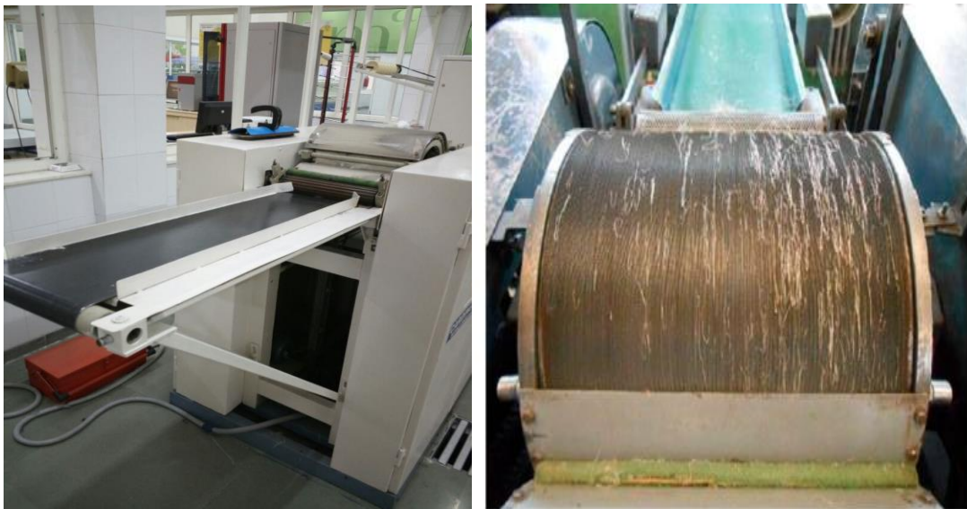
Plate 4.9: a) Carding machine b) Fibers adhere to the drum during carding process
