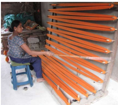
Plate 2.2: Preparation of warp yarns Source: http://en.wikipedia.org/wiki/Loom
