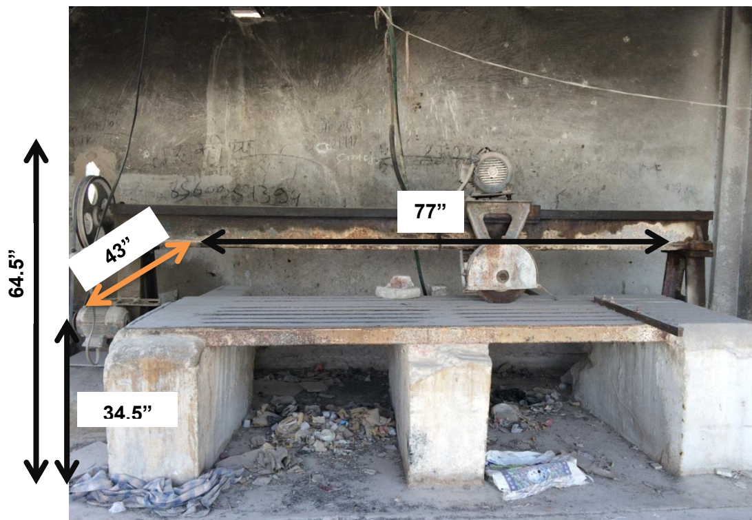
Figure 12: Dimensions of the Workstation
