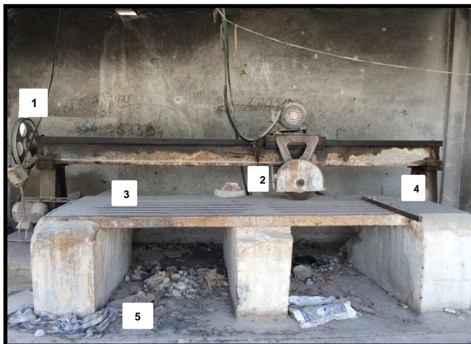
Figure 20: Marked points at which the Vibration was measured on the Marble Cutting Workstation
