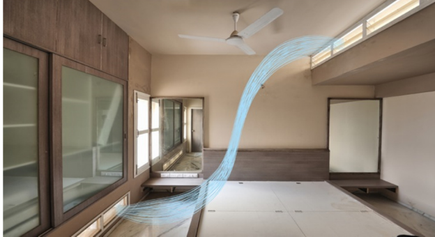
Plate 28: Openings on two directions of the room for cross ventilation
