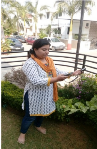
Plate 30: Measuring Daylight in the open area around the house with Light Meter
