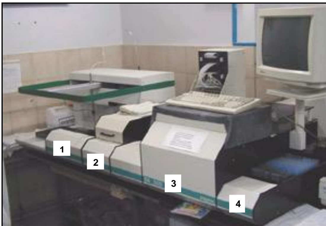
Figure 3.4: Stratec SR300 Automated Radio Immunoassay Analyzer
