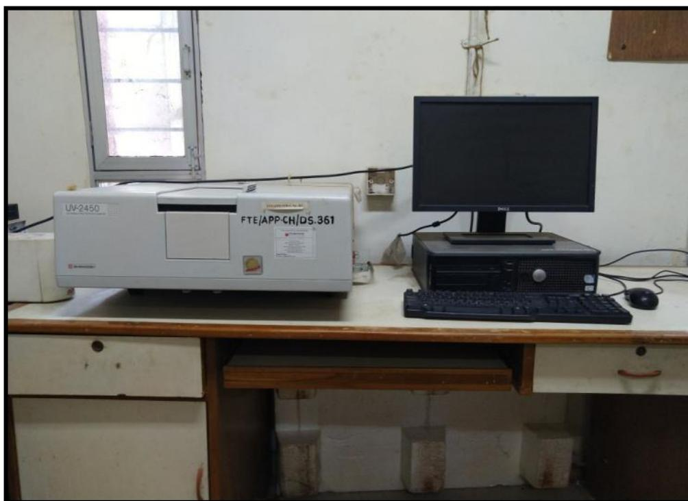
**Fig. 2.7.** UV/Vis Spectrophotometer.
