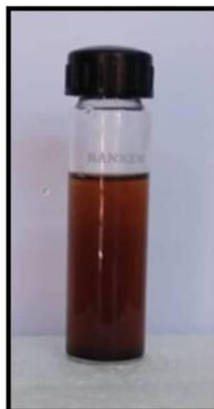
**Fig. 2.1.** An image of synthesized GO nanosheet and solution of GO.
