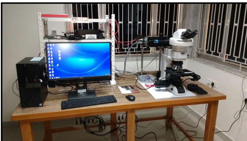
**Fig. 2.6.** Raman Spectrometer.
