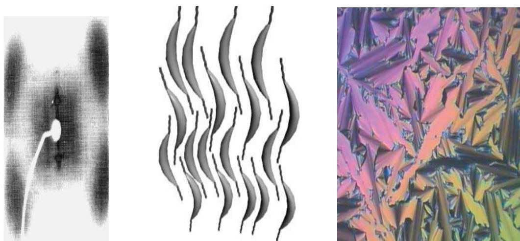
Figure 1.23: X-ray pattern and texture for B6 phase
