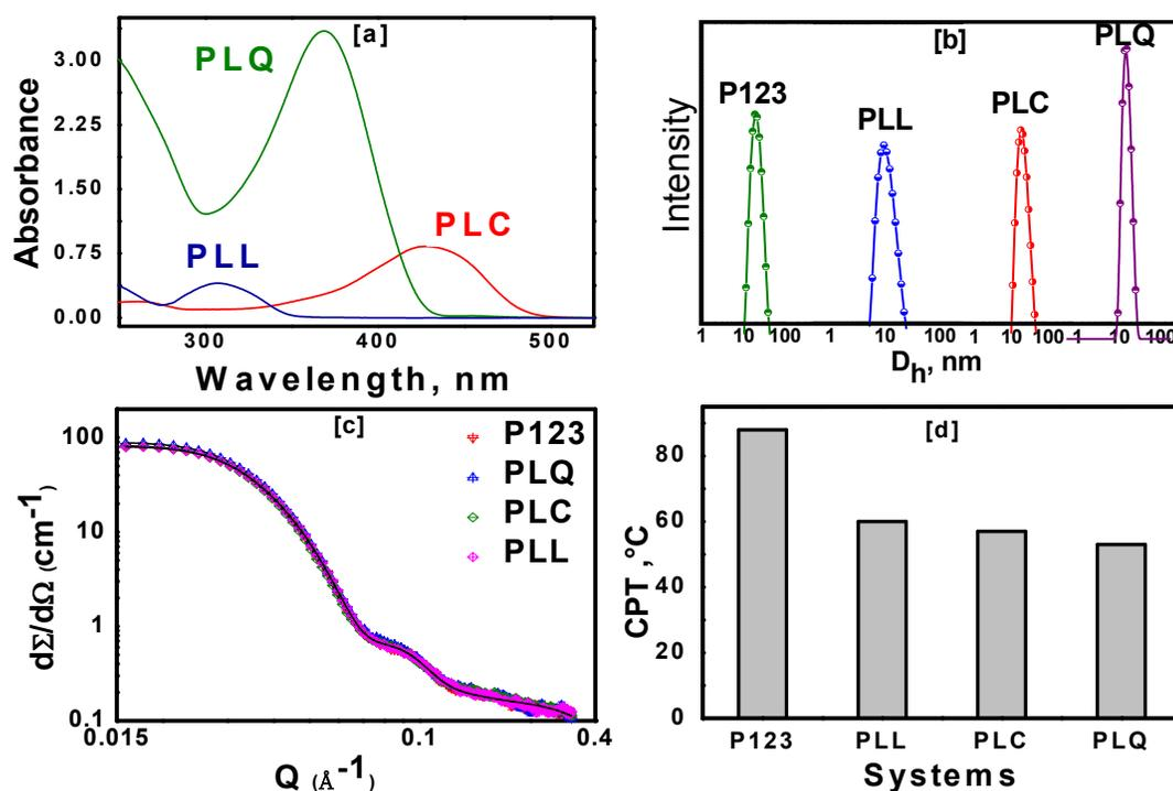
**Fig.4.7:** (a) UV-Visible absorbance spectra of PLC, PLQ and PLL in the water at room temperature (The spectra were taken with 100 times dilution of PLC and PLL and 10 times of PLQ in respective solvents. The aliphatic PluronicP123 and drugs not shown any peak in the spectrum). (b) DLS study of drug-loaded Pluronic P123 micelles at 30°C. (c) SANS study of drug-loaded Pluronic P123 micelles at 30°C. (d) CPT of 5 % Pluronic P123 in absence and presence of drugs.
