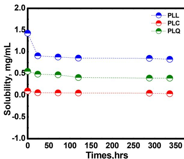
*Fig.4.10: Storage stability of drug-loaded Pluronic P123 micelles at 30°C.*
