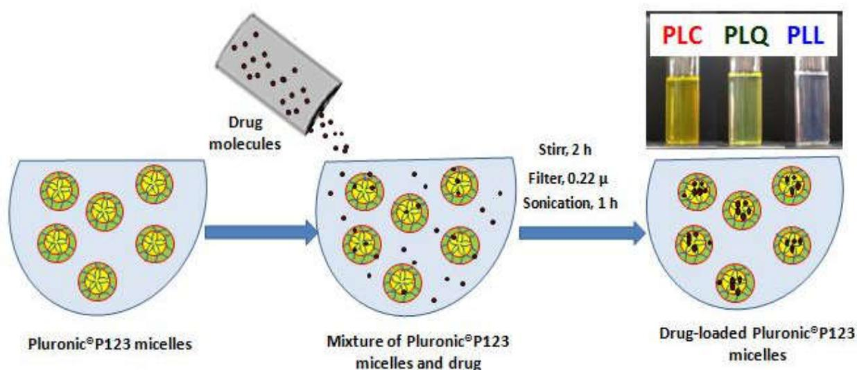
**Fig.4.3: Schematic representation of the preparation of drug-loaded Pluronic P123 micelles.**
