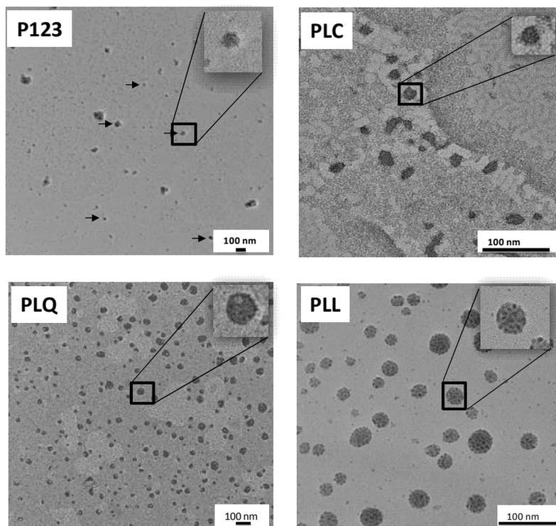
**Fig.4.8: TEM images of drug-loaded Pluronic P123 micelles at 30°C.**
