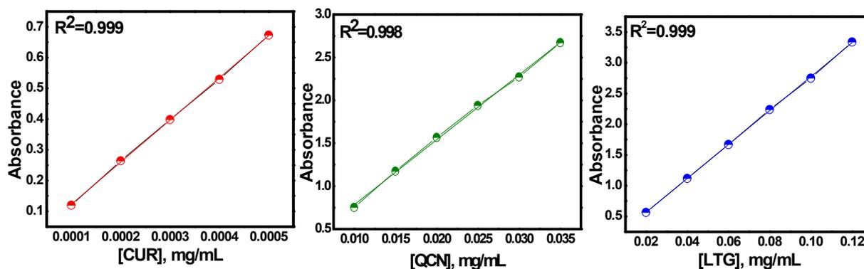
**Fig.4.2: Calibration curve of studied hydrophobic drugs (diluted with methanol/ethanol) at 30° C.**
