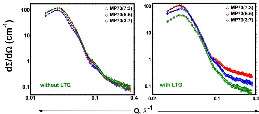
**Fig 6.7: Neutron scattering curves for 10 wt% solutions of mixed F127: P123 micellar systems with and without LTG at 37°C.**
