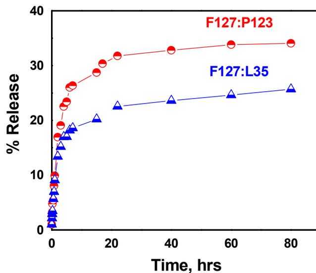
**Fig.6.10: In vitro release profile of LTG drug from mixed F127:P123 and mixed F127:L35 micellar systems at 37°C.**
