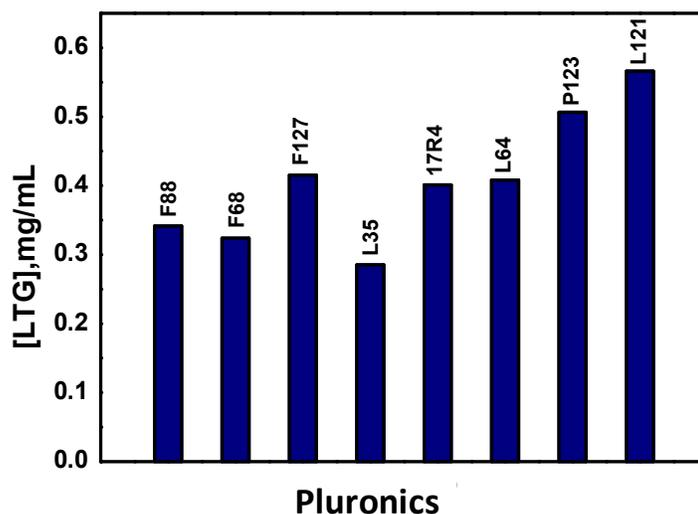
**Fig.6.2:** The solubility of LTG in 1.0 wt % aqueous solutions of Pluronic polymers at room temperature (30°C).
