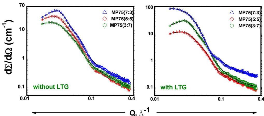
**Fig.6.8: Neutron scattering curves for 10 wt% solutions of mixed F127:L35 micellar systems with and without LTG at 37°C.**
