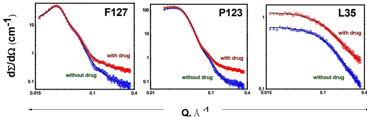
**Fig.6.6: Neutron scattering curves for 10 wt% solutions of F127, P123, and L35 in the absence and presence of LTG in  $D_2O$  at  $37^\circ C$ .**
