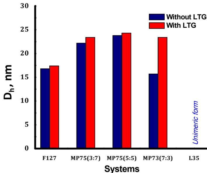
**Fig.6.5:** Average  $D_h$  values of F127, L35, and mixed F127:L35 micellar systems with and without LTG drug at 37°C.
