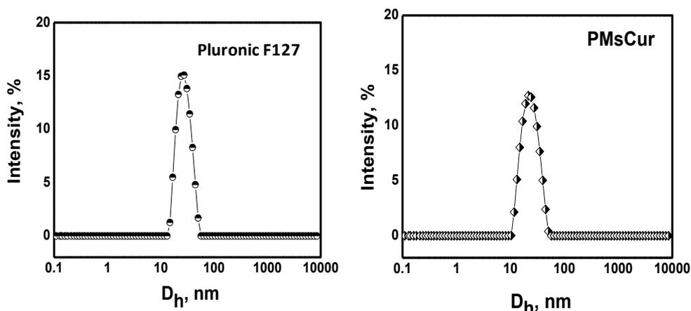
Fig.2.6: Intensity versus hydrodynamic size of 1.0wt% aqueous solution of Pluronic F127 and PMsCur in water at 37°C.
