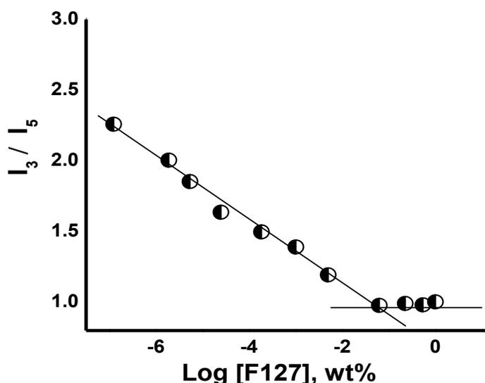
**Fig.2.3: Plot of  $I_3/I_5$  versus the log of Pluronic F127 concentration in water at 30°C.**
