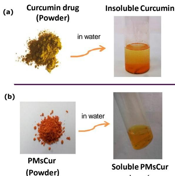
**Fig.2.5: (a) Insoluble slurry of curcumin when added in water (b) Synthesized PMsCur dispersed (soluble curcumin) in water.**
