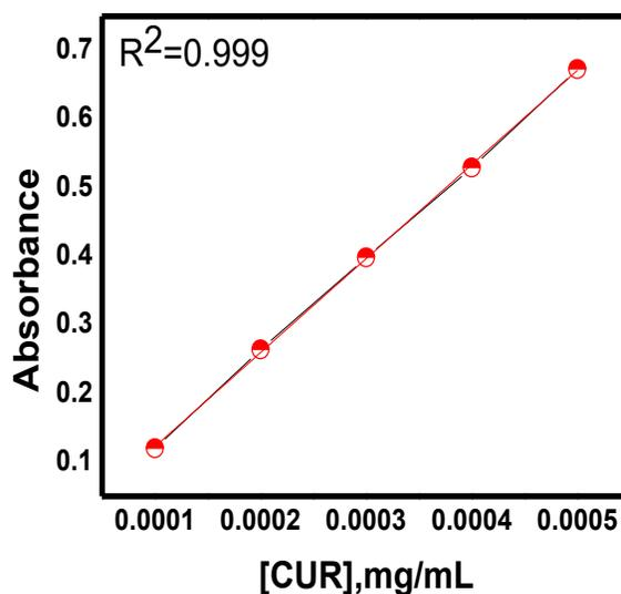
*Fig.2.2: Calibration curve of curcumin in ethanol as solvent.*
