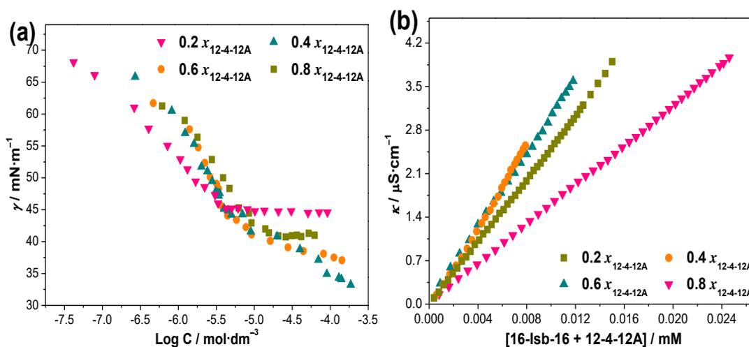
**Figure 4.** (a) Plot of surface tension ( $\gamma$ ) vs  $\text{log } C$  (logarithm of concentration) and (b) Plot of specific conductance ( $\kappa$ ) vs [surfactants], of mixed gemini surfactants (16-Isb-16 + 12-4-12A) at different mole fractions ( $x$ ) of anionic gemini (12-4-12A) in aqueous solution at 303 K.
