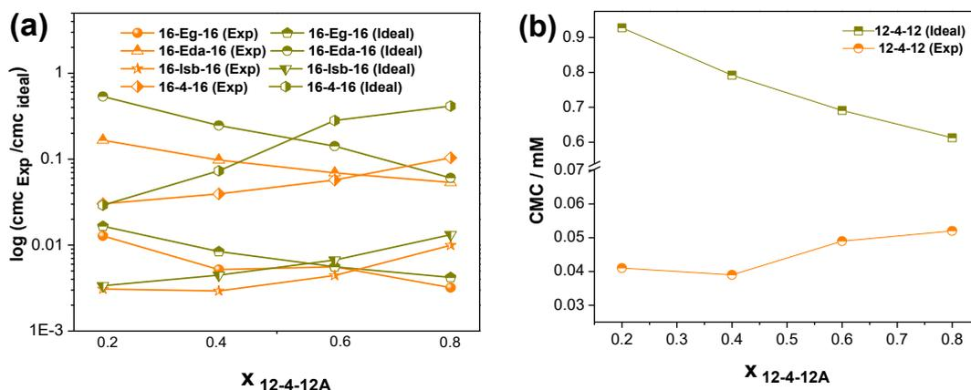
**Figure 6.** Critical micelle concentration ( $cmc$ ) by conductometry with a variation of mixed surfactant systems (cationic-anionic) with a mole fraction of anionic gemini surfactant ( $x_{12-4-12A}$ ) in aqueous solution at 303 K. The plot represents experimental and ideal values (calculated from ideal mixing model).
