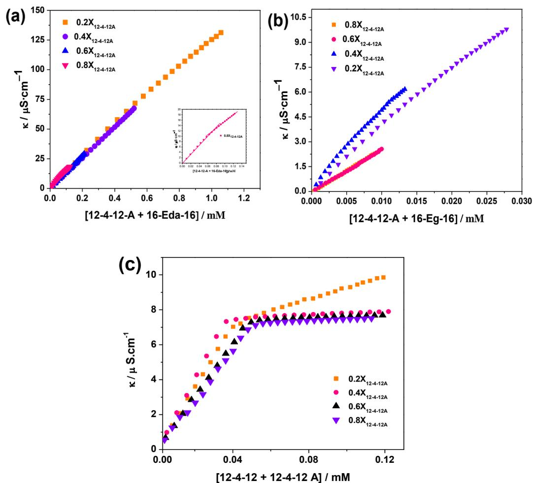
**Figure 5.** Plot of specific conductance ( $\kappa$ ) vs [surfactants], of mixed gemini at different mole fractions ( $x$ ) of anionic gemini (12-4-12A) in aqueous solution at 303 K. (a) 16-Eda-16 + 12-4-12A (b) 16-Eg-16 + 12-4-12A and (c) 12-4-12 + 12-4-12.
