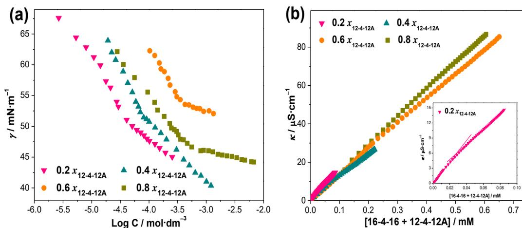
**Figure 3.** (a) Representative plot of surface tension ( $\gamma$ ) vs  $\text{log } C$  (logarithm of concentration) and (b) Plot of specific conductance ( $\kappa$ ) vs [surfactants], of mixed gemini surfactants (16-4-16 + 12-4-12A) at different mole fractions ( $x$ ) of anionic gemini (12-4-12A) in aqueous solution at 303 K.
