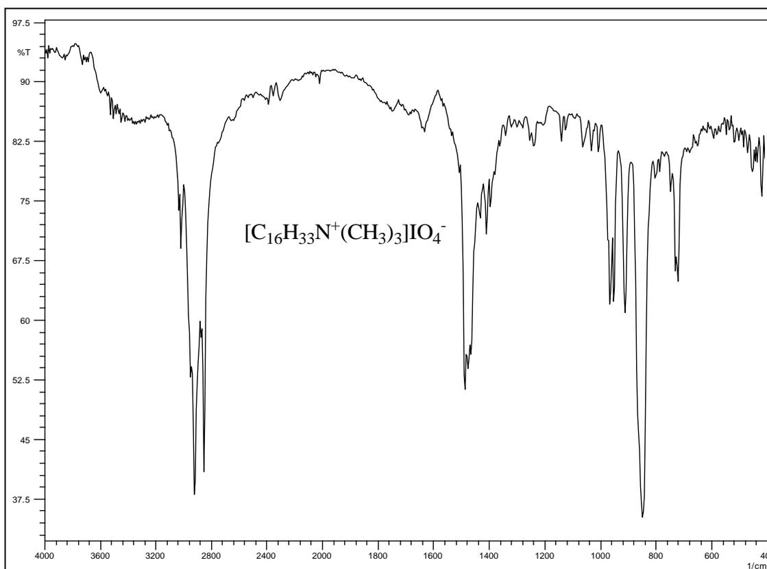
**Figure 4.5** FTIR spectrum of Cetyltrimethyl ammonium periodate (CTAPI) (15)
