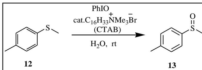
**Scheme 4.5** Oxidation of methyl *p*-tolyl sulfide (**12**) to methyl *p*-tolyl sulfoxide (**13**) using iodosobenzene (PhIO) as oxidant in the presence of a catalytic amount of (CTAB)
