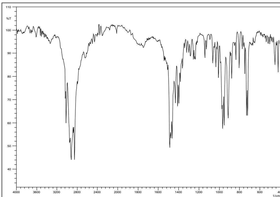
**Figure 4.4** FTIR spectrum of Cetyltrimethyl ammonium bromide (CTAB)
