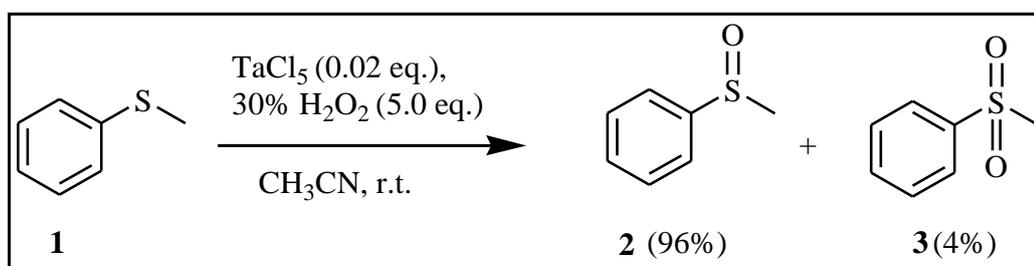
**Scheme 4.1** Oxidation of methyl phenyl sulfide (**1**) using tantalum (V) chloride as a catalyst
