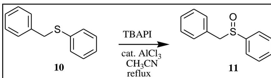
**Scheme 4.4** Oxidation of Benzyl phenyl sulfide (**10**) to Benzyl phenyl sulfoxide (**11**) using TBAPI as oxidant
