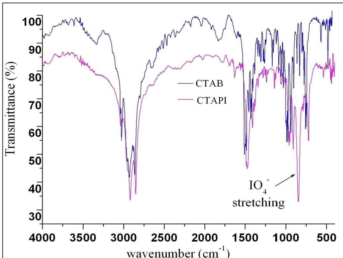
**Figure 4.3** FTIR spectra of CTAB (**14**) and CTAPI (**15**)
