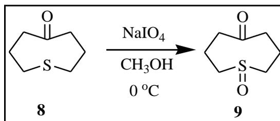
**Scheme 4.3** Oxidation of 1-thiacyclooctan-5-one (**8**) to corresponding sulfoxides (**9**) using sodium metaperiodate
