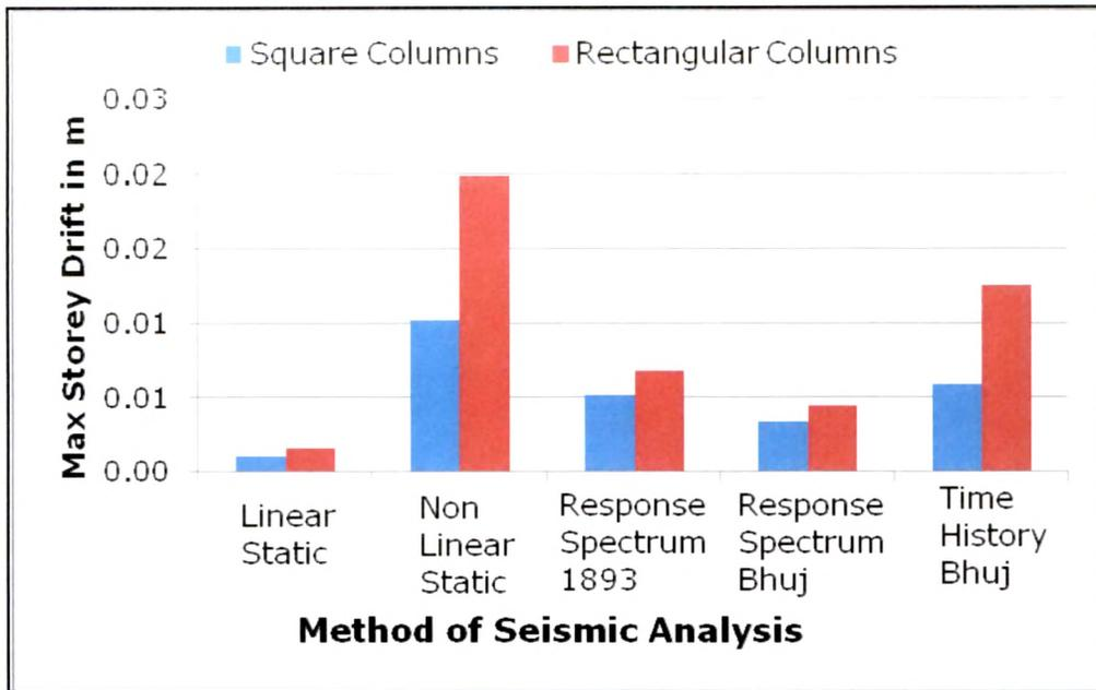
**Fig.15.6 Storey Drift Comparison for a G+7 Storey Frame**
