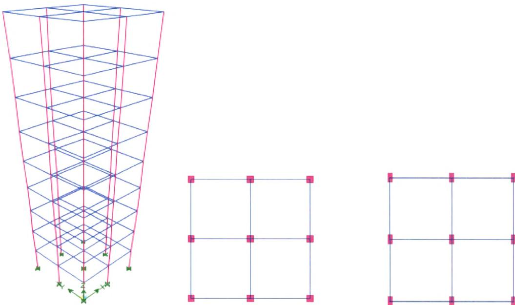
**Fig. 15.1 Typical Isometric and Plan Views of the G+7 Frame**
