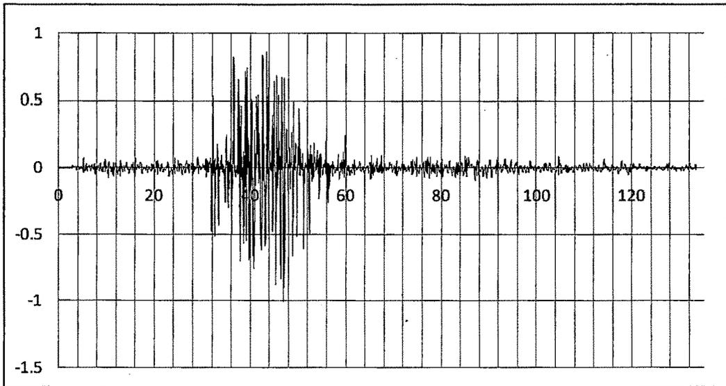
**Figure 15.2 Time versus Acceleration Record for Bhuj Earthquake**
