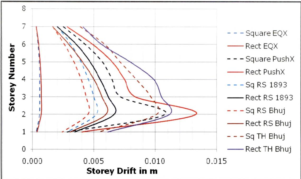
**Fig. 15.11 Storey Drift Plot for G+5 Storey Frame in X Direction**
