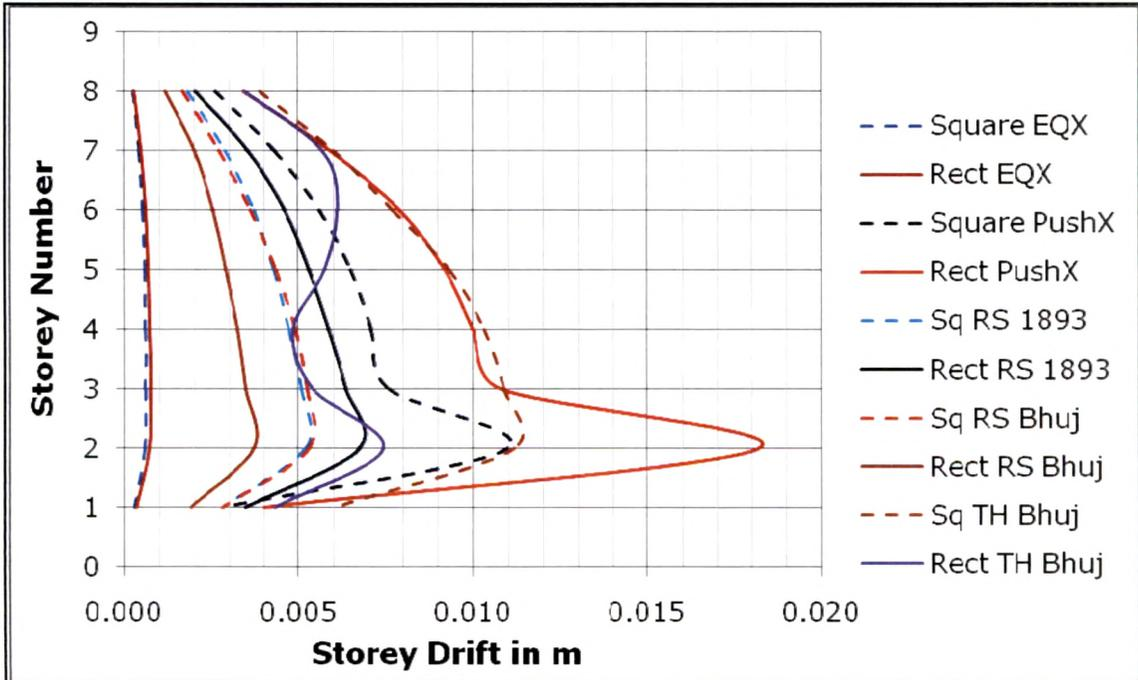
**Fig. 15.10 Storey Drift Plot for G+6 Storey Frame in X Direction**
