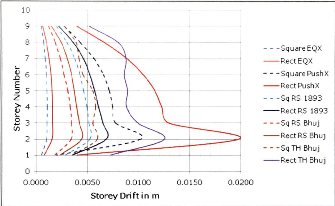
**Fig. 15.9 Storey Drift Plot for G+7 Storey Frame in X Direction**
