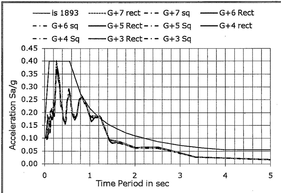
**Fig. 15.3 Response Spectra for Models for Bhuj Earthquake**
