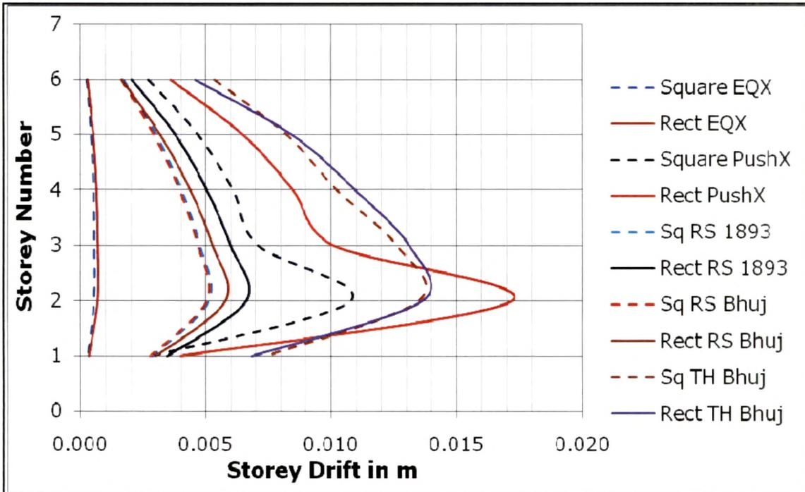
**Fig. 15.12 Storey Drift Plot for G+4 Storey Frame in X Direction**
