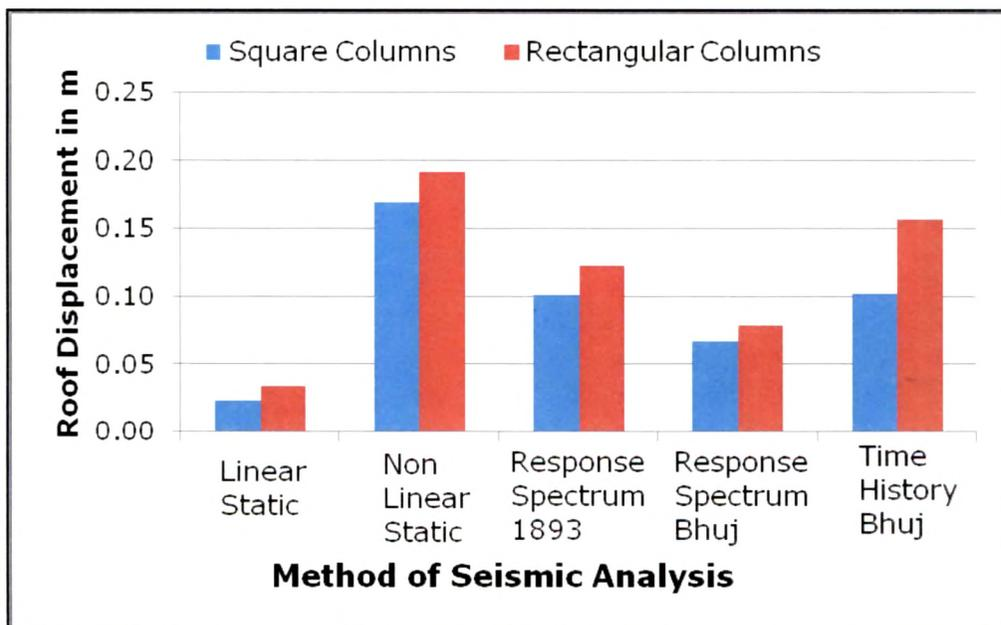
**Fig.15.5 Roof Displacement Comparison for a G+7 Storey Frame**
