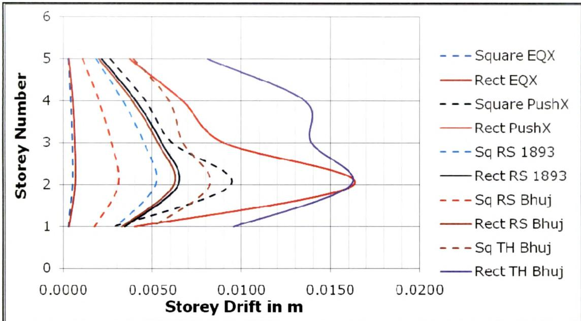
**Fig. 15.13 Storey Drift Plot for G+3 Storey Frame in X Direction**
