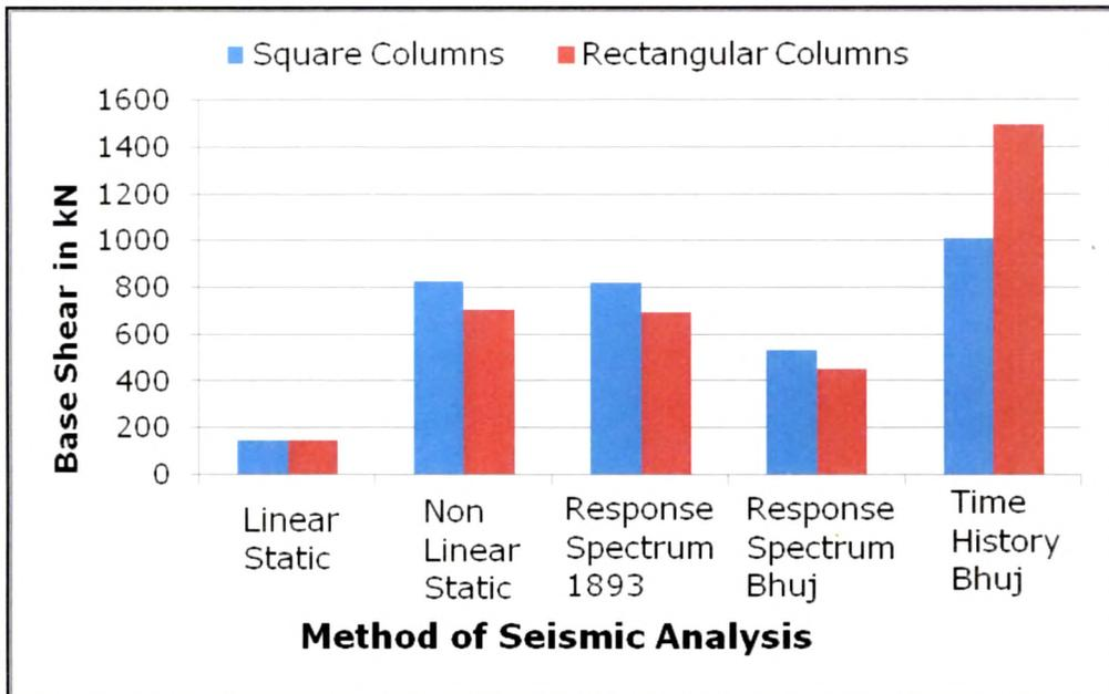
**Fig.15.4 Base Shear Comparison for a G+7 Storey RC Frame**
