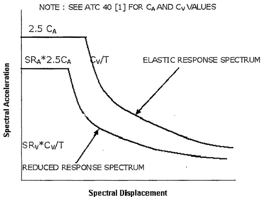
**Fig. 4.13 Reduced Response Spectrum**
