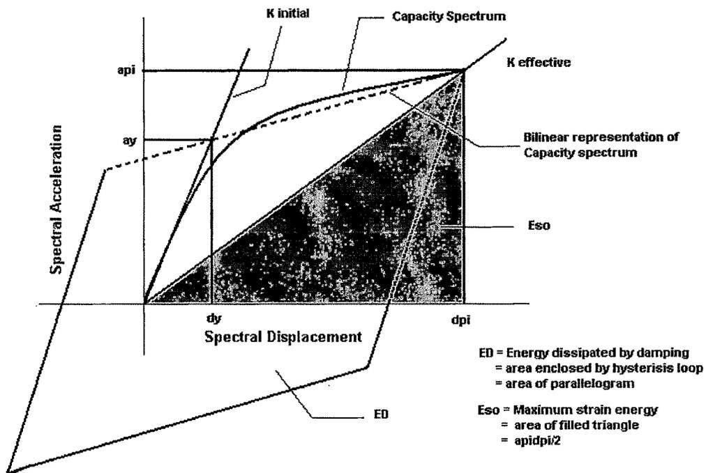
**Fig. 4.11 Derivation of Damping for Spectrum Reduction**
