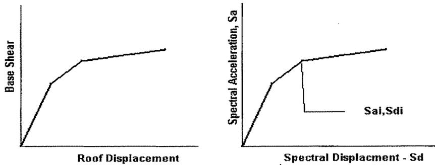
**Fig. 4.15 Converting Capacity Spectrum to ADRS Format**
