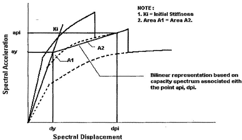
**Fig. 4.10 Bilinear Representation for Degrading System**
