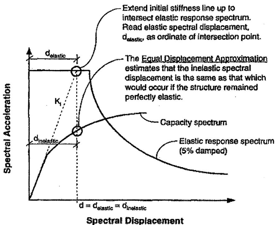
**Fig. 4.8 Equal Displacement Approximation**
