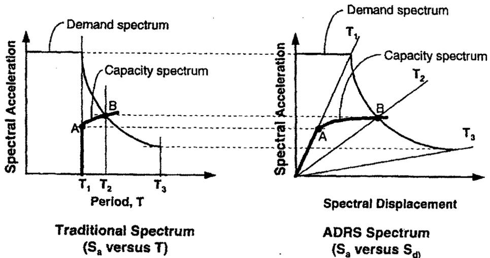
**Fig. 4.16 Capacity Spectrum Superimposed over Demand Spectrum**
