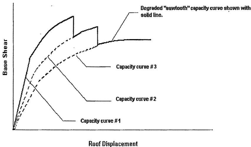
**Fig. 4.7 Capacity Curve with Global Strength Degradation**
