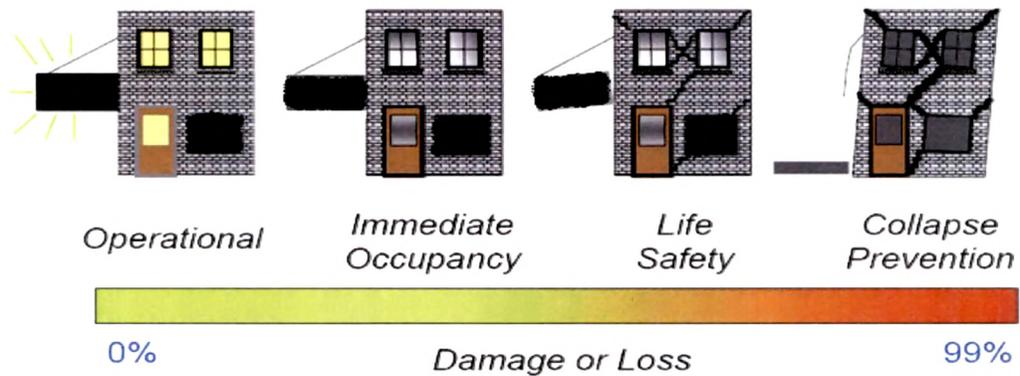
**Fig. 4.1 Standard Structural Performance Levels**
