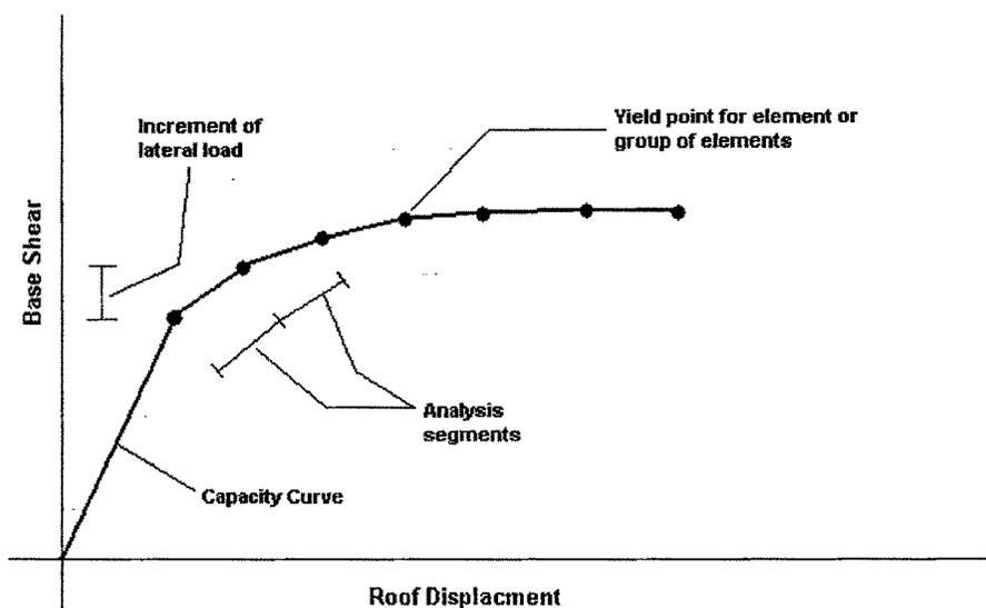
**Fig. 4.5 Capacity Curve**
