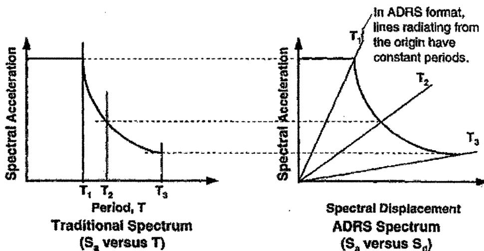
**Fig. 4.14 Converting Demand Spectra to ADRS Format**
