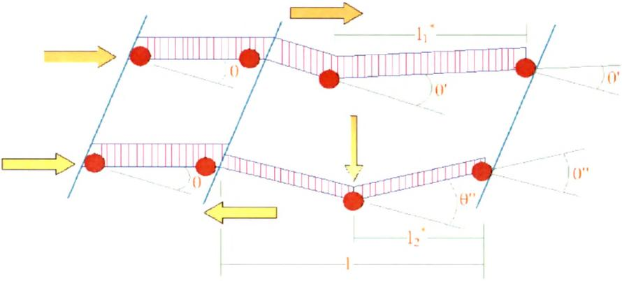
**Fig. 4.3 Plastic Hinge Pattern Dominated by Gravity Loading**
