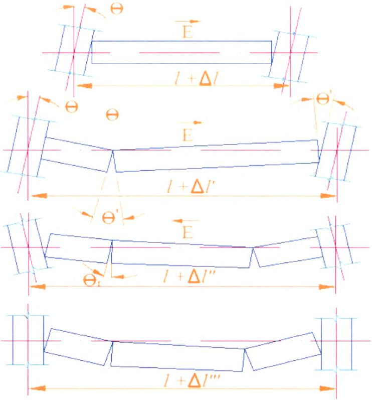
**Fig. 4.2 Plastic Hinge Pattern by Seismic Actions**
