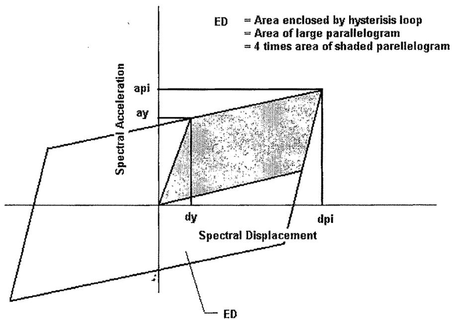
**Fig. 4.12 Derivation of Energy Dissipated by Damping,  $E_D$**
