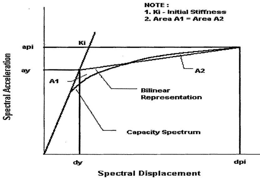
**Fig. 4.9 Bilinear Representation of Capacity Spectrum**
