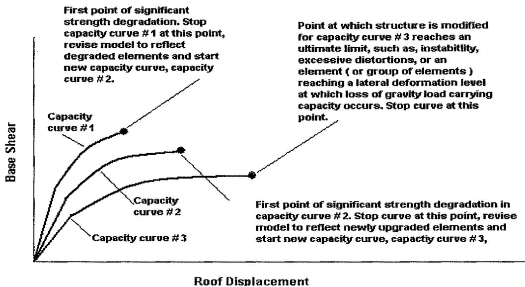
**Fig. 4.6 Multiple Capacity Curve to Model Strength Degradation**
