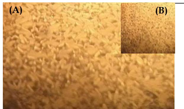
Fig. 4. (a) Optical image of doped Lanthanum sulphide complex (b) Magnified image of doped Lanthanum sulphide complex
