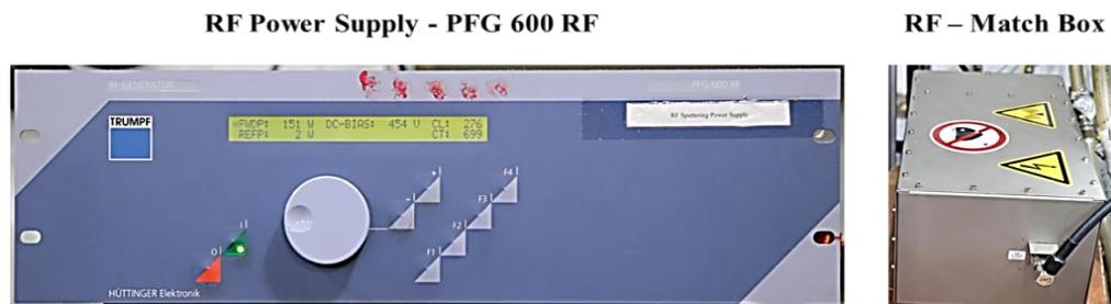
**Fig. 2.3: Photograph of Radio Frequency sputtering power supply and impedance RF Match-Box.**
