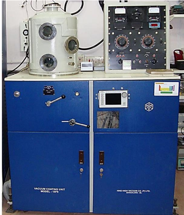
**Fig. 2.1: Photograph of Vacuum Coating Unit for multilayer deposition of thin films.**
