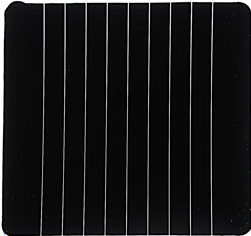
Fig 3.26: Photo (using back light) of bi-layer molybdenum thin film on 60 x 60 mm square SLG using P1 scribing process with the optimized parameter of Nd:YAG fiber laser.
