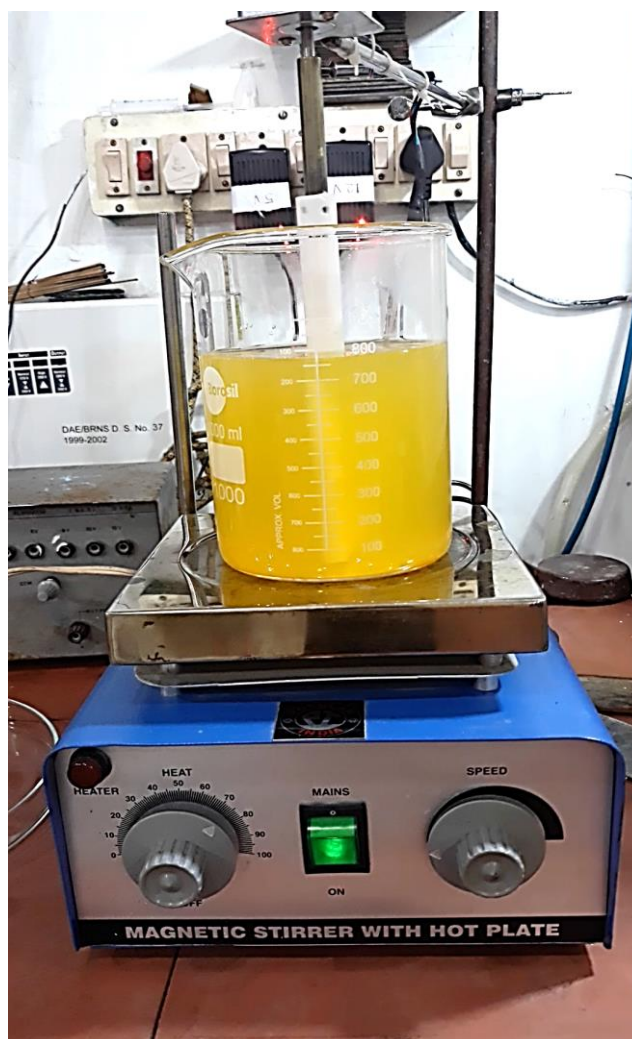
Fig. 5.1: Chemical Bath Deposition process for CdS thin film deposition.
