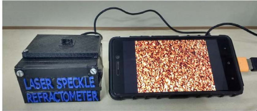
Fig 3. 18: A speckle pattern recorded by the smartphone, when attached to the webcam of the refractometer with the help of a USB OTG
