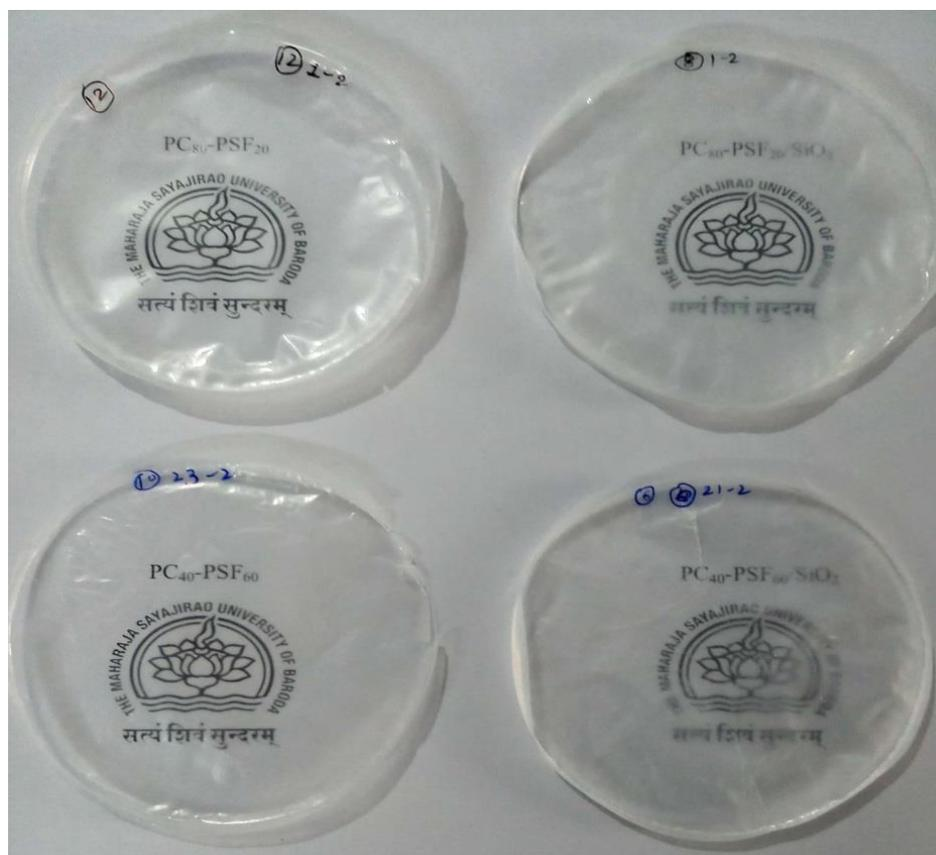
**Figure 5.6 (b)** Optical micrograph of blend and SiO<sub>2</sub> doped blend membranes.
