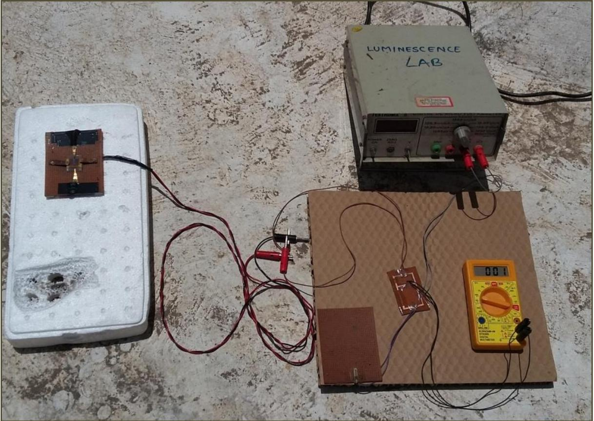
Figure 5.4: Actual view of measurement of Solar-Cell efficiency under Sunlight.
