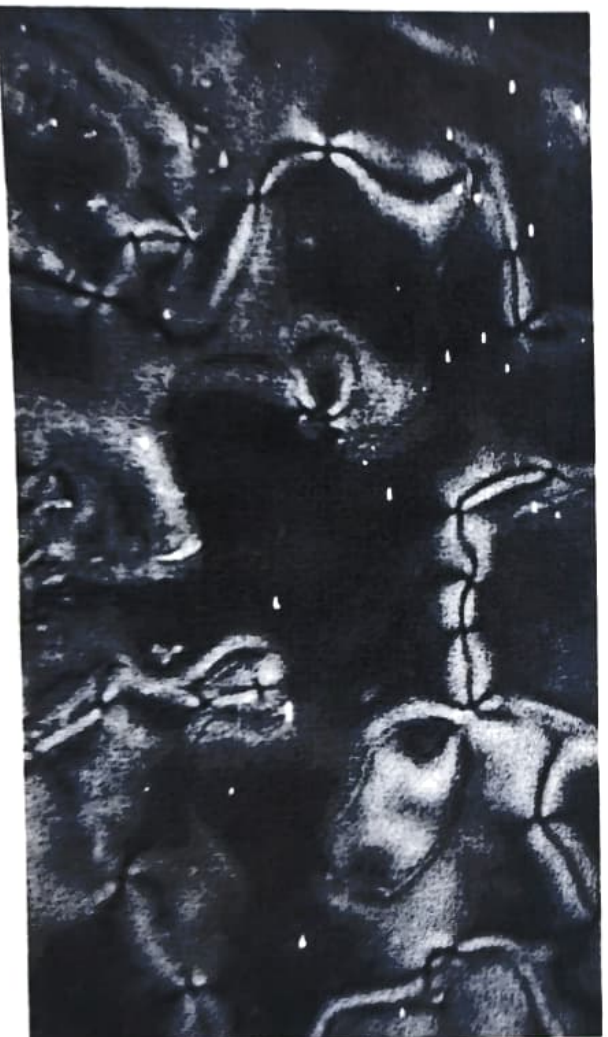
Optical polarized microphotograph of Nematic liquid crystalline phase (Thread like texture) of EP-4 on cooling at 154 °C (Paper Published)
