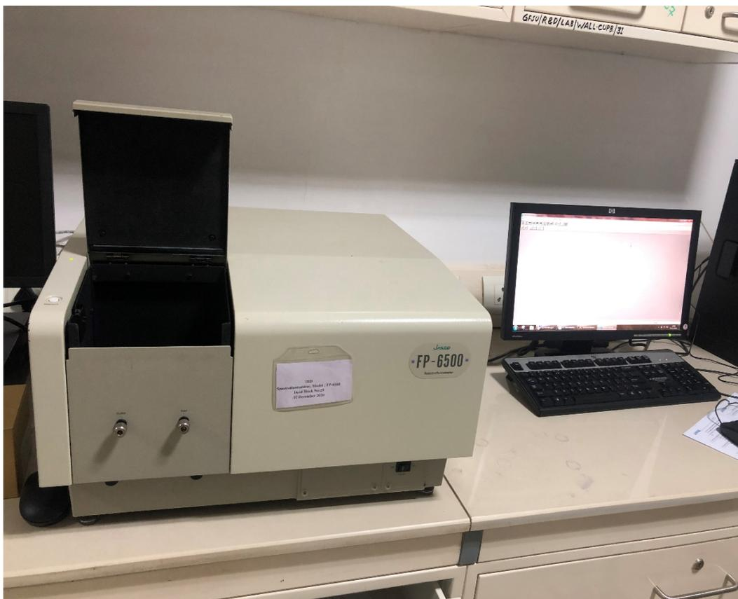
**Figure 2.11:** Actual image of the instrument JASCO FP-6500 spectrofluorometer
