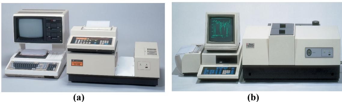
**Figure 2.6:** (a) In 1981, the IR-435, a dispersive instrument featured an integrated microcomputer and room for optional ROM memory; accurate spectrum recordings of rapid reaction processes and automatic peak detection became possible, (b) In 1984 Shimadzu's first Fourier Transform Infrared Spectrophotometer was launched [5].
