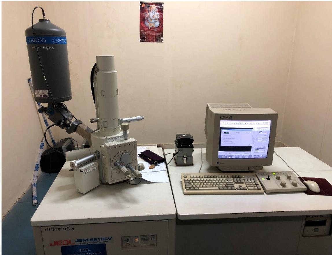
**Figure 2.4:** Actual image of Energy Dispersive X-ray Spectroscopy (EDS)
