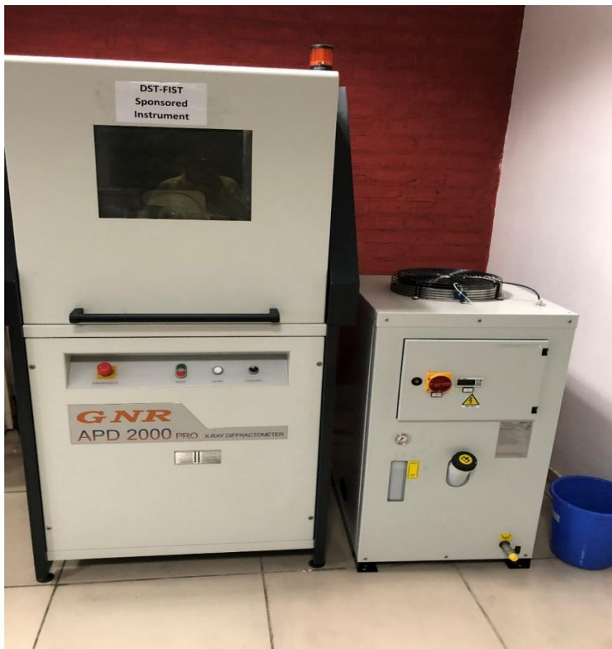
**Figure 2.3:** Actual image of the instrument GNR APD 2000 PRO XRD
