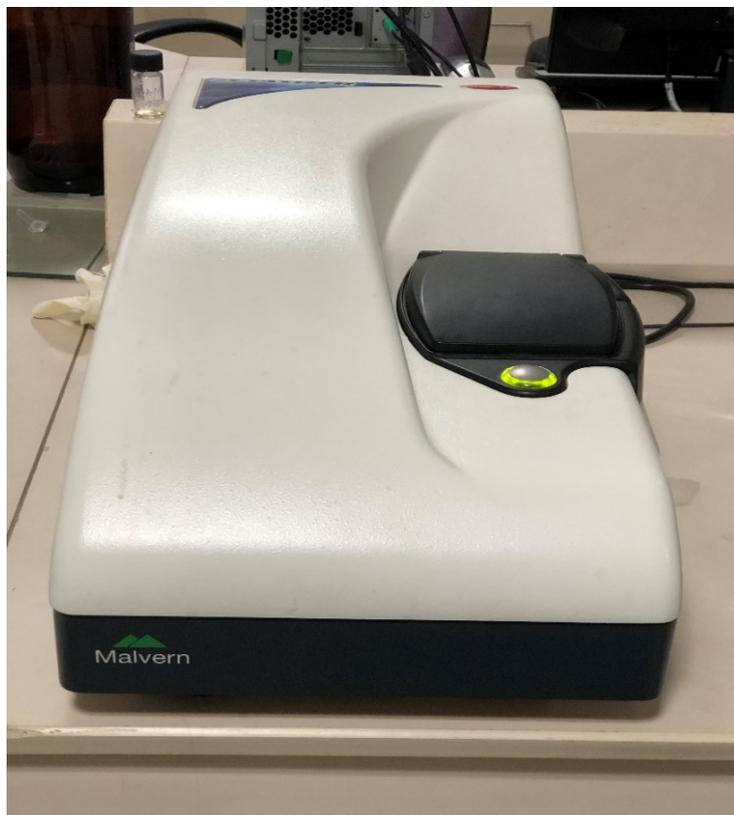
**Figure 2.5:** Actual image of Malvern Nano ZS Particle Size Analyzer
