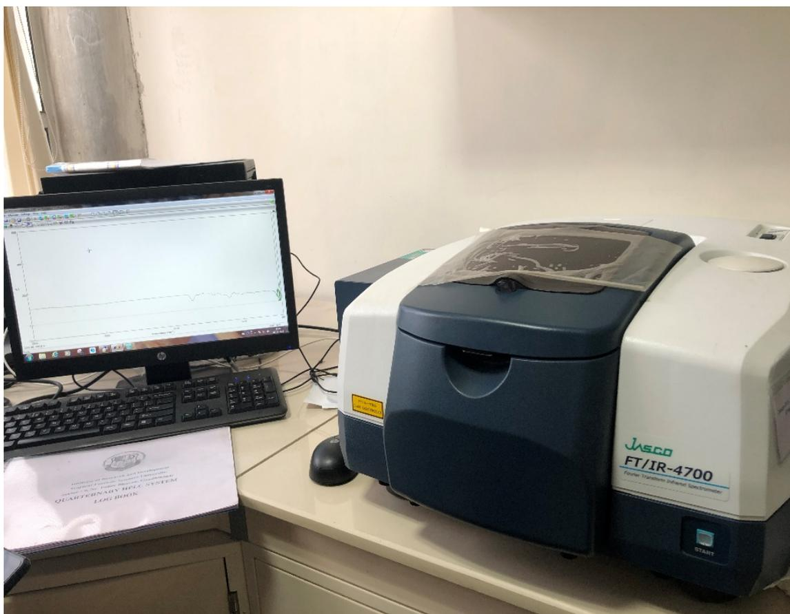
**Figure 2.8:** Actual image of the instrument JASCO FT/IR-4700 spectrometer
