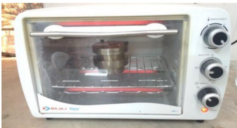
Image of stainless steel autoclave in oven used for synthesis
