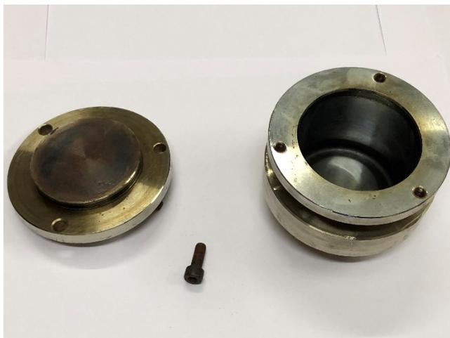
Image of stainless steel autoclave for hydrothermal technique
