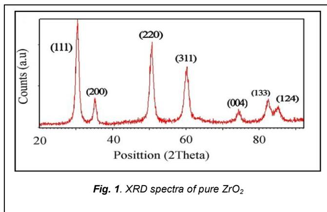
**Fig. 1.** XRD spectra of pure  $\text{ZrO}_2$
