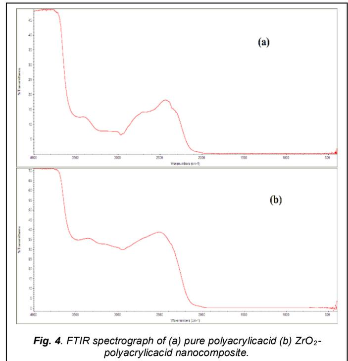
Fig. 4. FTIR spectrograph of (a) pure polyacrylicacid (b)  $ZrO_2$ -polyacrylicacid nanocomposite.
