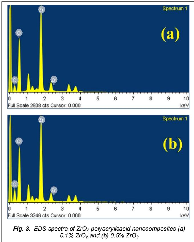
Fig. 3. EDS spectra of  $ZrO_2$ -polyacrylicacid nanocomposites (a) 0.1%  $ZrO_2$  and (b) 0.5%  $ZrO_2$
