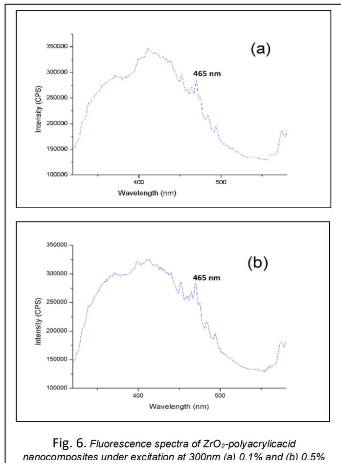
Fig. 6. Fluorescence spectra of ZrO<sub>2</sub>-polyacrylicacid nanocomposites under excitation at 300nm (a) 0.1% and (b) 0.5%
