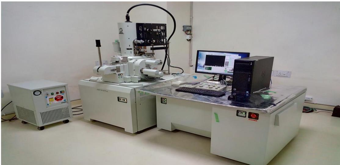
Figure 3-8: A Typical Set Up of FESEM
