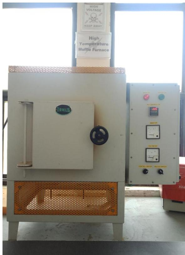
Figure 3.1: High Temperature Muffle Furnace at Department of Nanoscience and Advanced Materials, Saurashtra University, Rajkot in which samples were synthesized using Solid State reaction.
