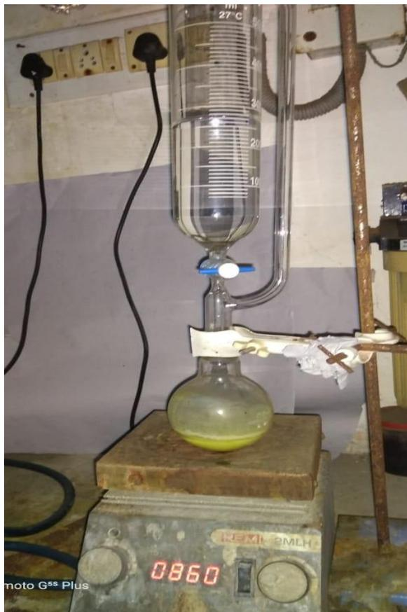
Figure 3-3: Precipitation Reaction Apparatus at M. M. Patel Science and Research Institute, Kadi Campus, Gandhinagar used to synthesize samples.
