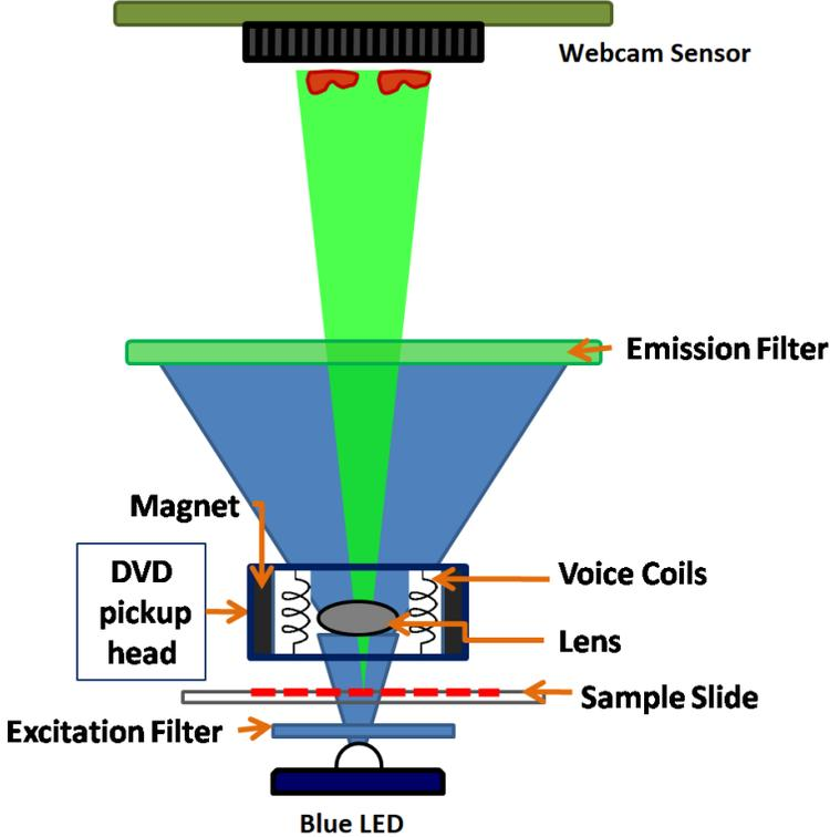
Figure 2.2.1 Schematic of developed Compact Fluorescence microscope
