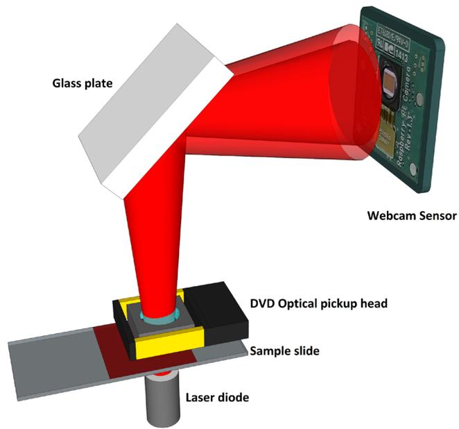
Figure 4.2.3 Schematic of Compact 3D LSDHM
