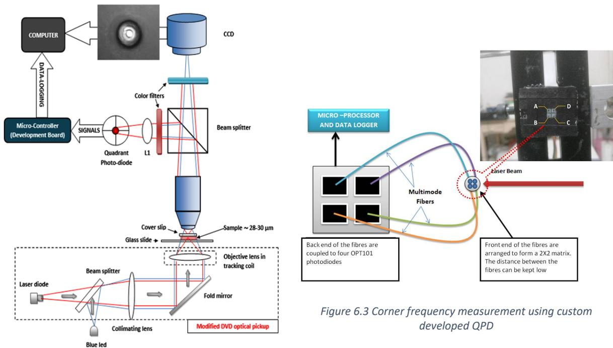
Figure 6.2 Schematic of optical trapping setup
