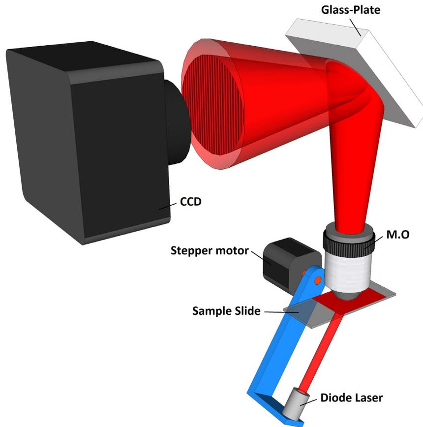
Figure 4.3.1 Schematic of Phase tomography technique using oblique illumination
