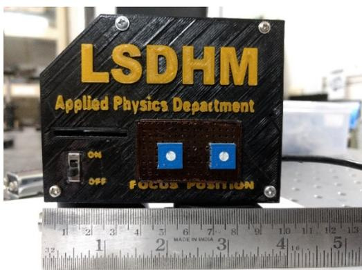
Figure 4.2.1 Developed 3D printed compact LSDHM
