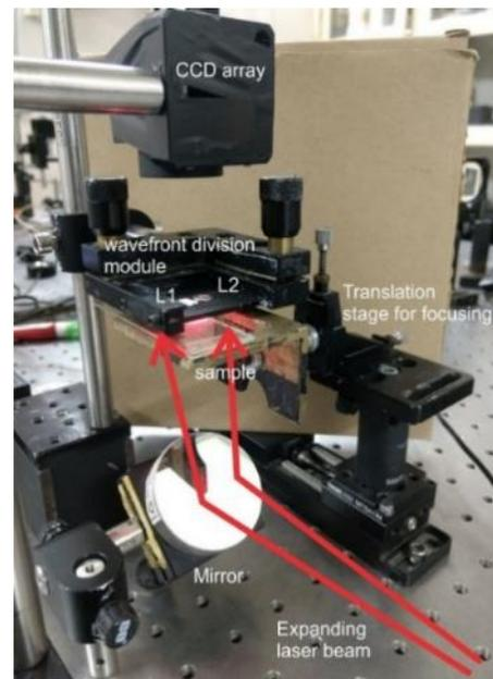
Figure 5.2 Lab Setup of WD-DHM
