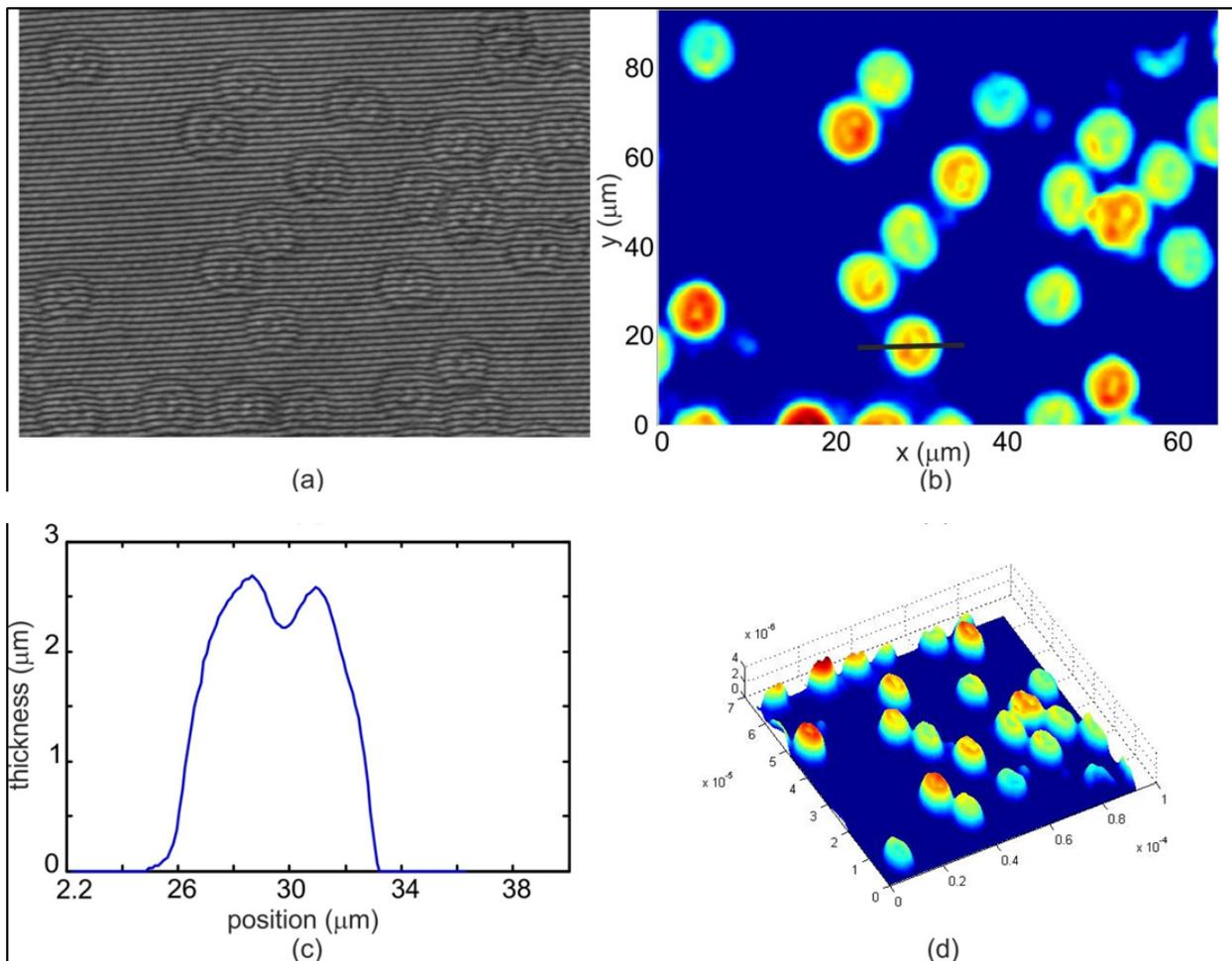
Figure 3.1.2 (a) Object Hologram, (b) Phase distribution, (c) 2D Line profile and (d) 3D profile
