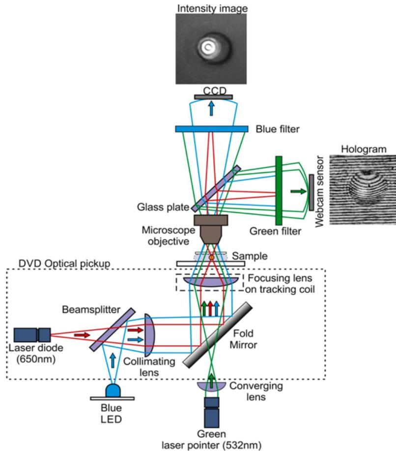
Figure 6.5 Optical trapping setup combined with LSDHM
