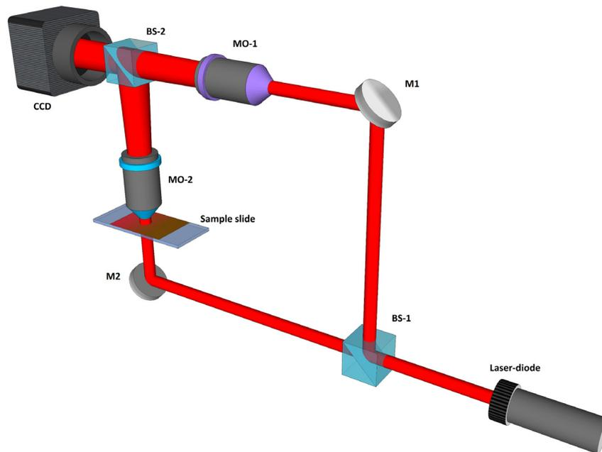
Figure 3.1.1 Schematic of the digital holographic microscope using Mach-Zehnder configuration
