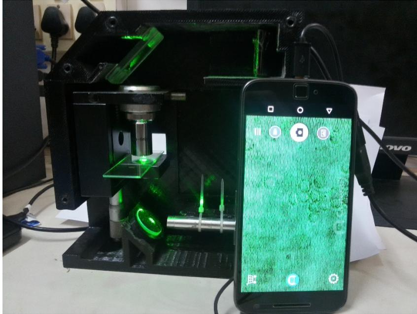
Figure 4.1.1 Developed 3D printed LSDHM Device
