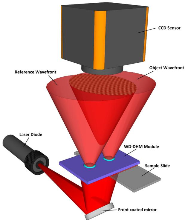
Figure 5.1 Schematic of WD-DHM
