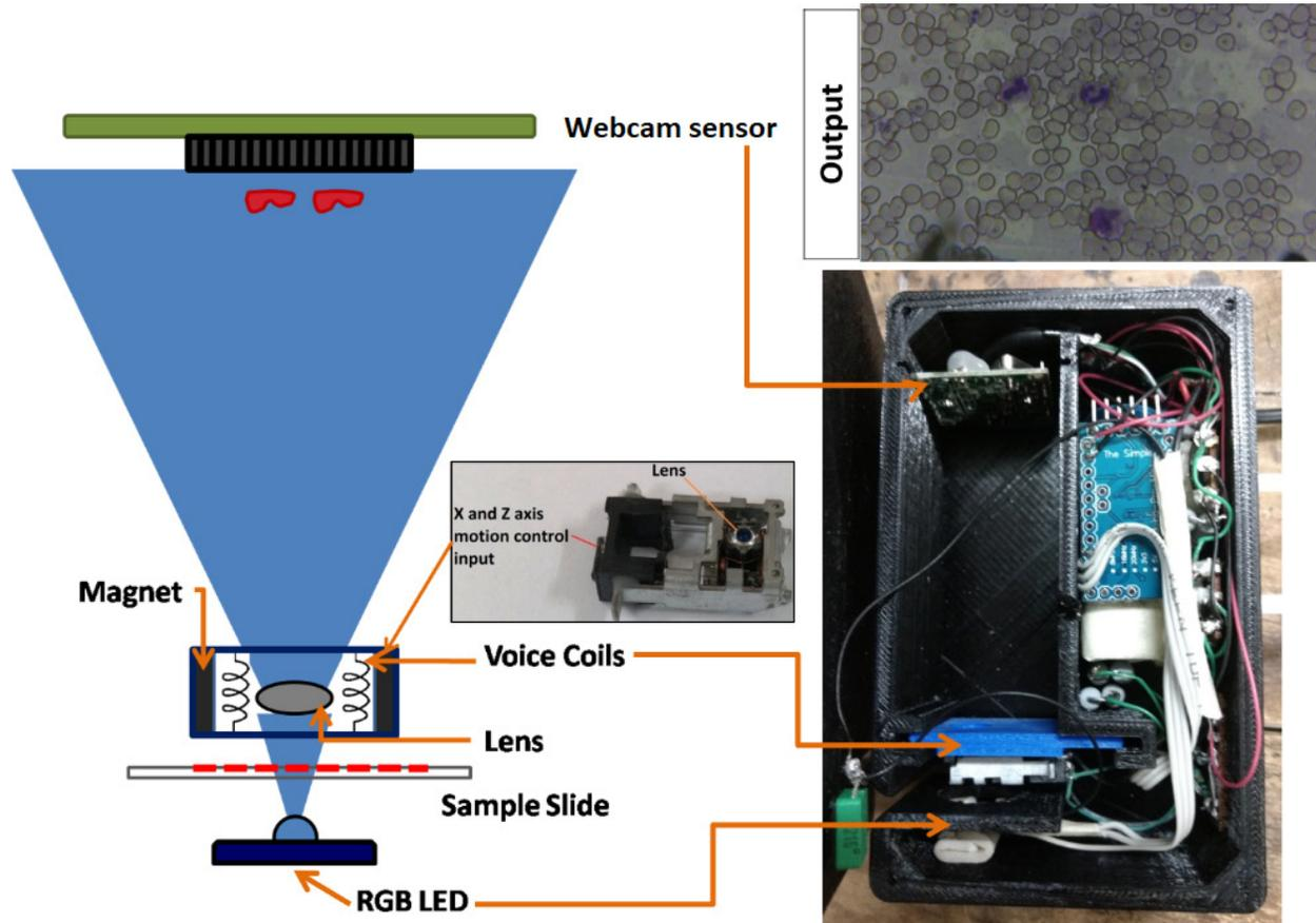
Figure 2.1.1 Working principle and inside-view of developed BFM
