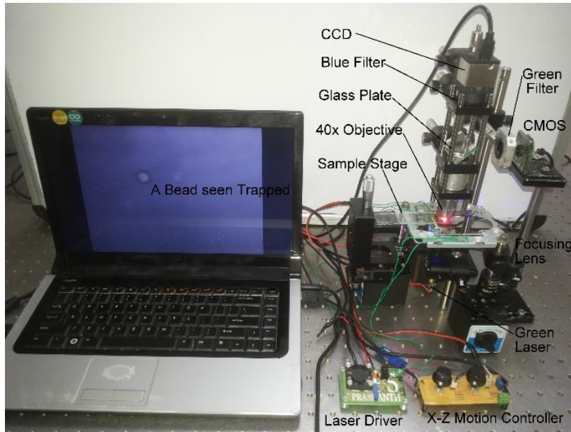
Figure 6.1 Lab Setup of optical trapping
