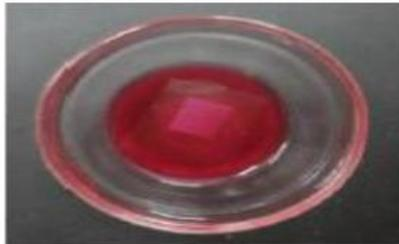
This electrode is immersed in pomegranate juice for 18 h.
