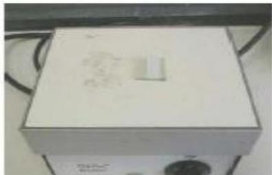
The coated conducting glass plate is sintered at 450°C for 30 min.
