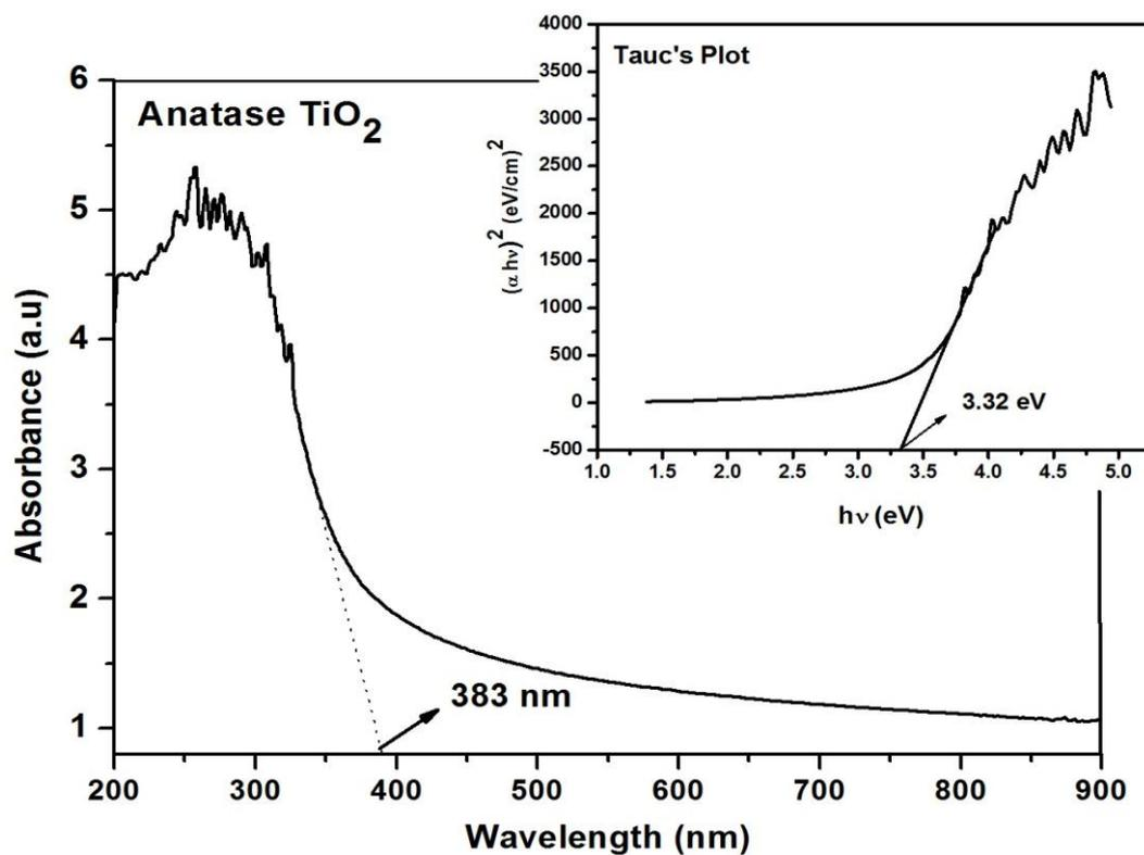
Figure 8: Absorption spectrum and Tauc's plot for Anatase TiO<sub>2</sub>
