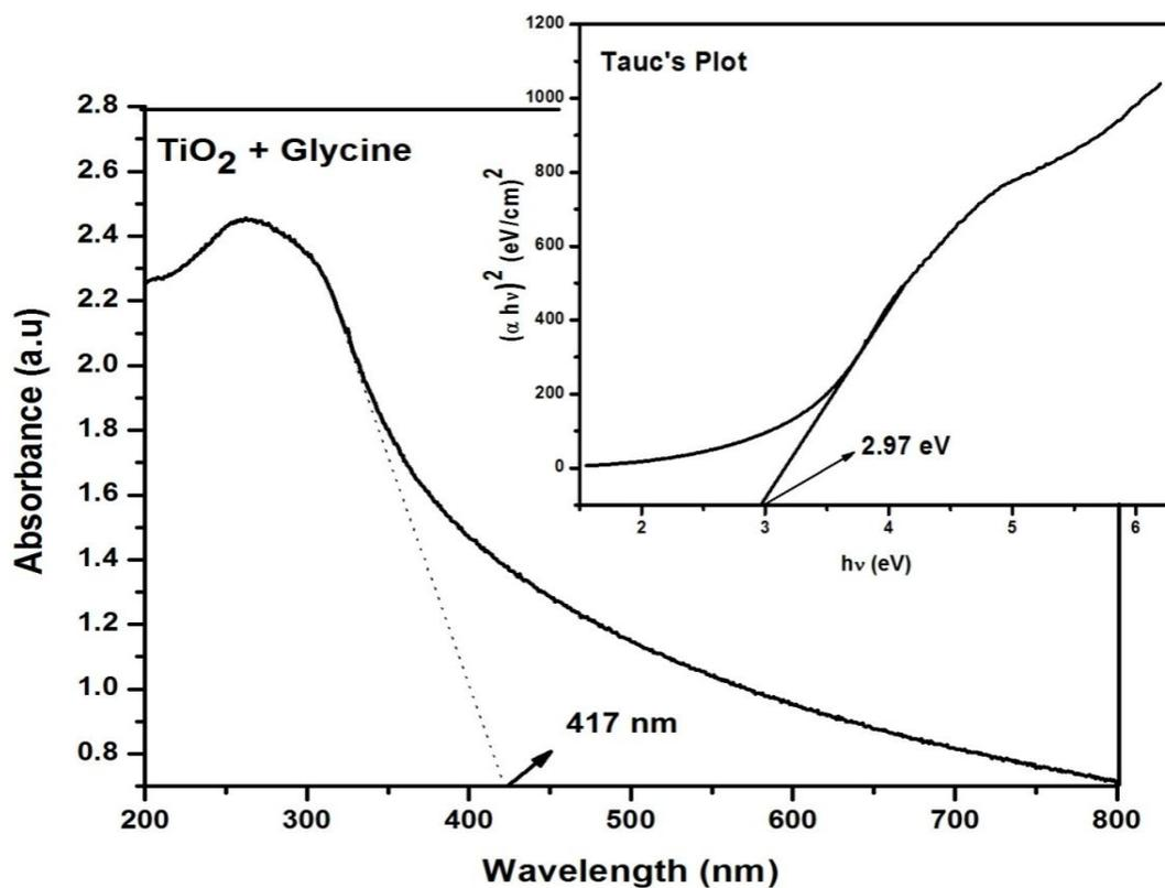
Figure 12: Absorption spectrum and Tauc's plot for  $\text{TiO}_2$  with Glycine
