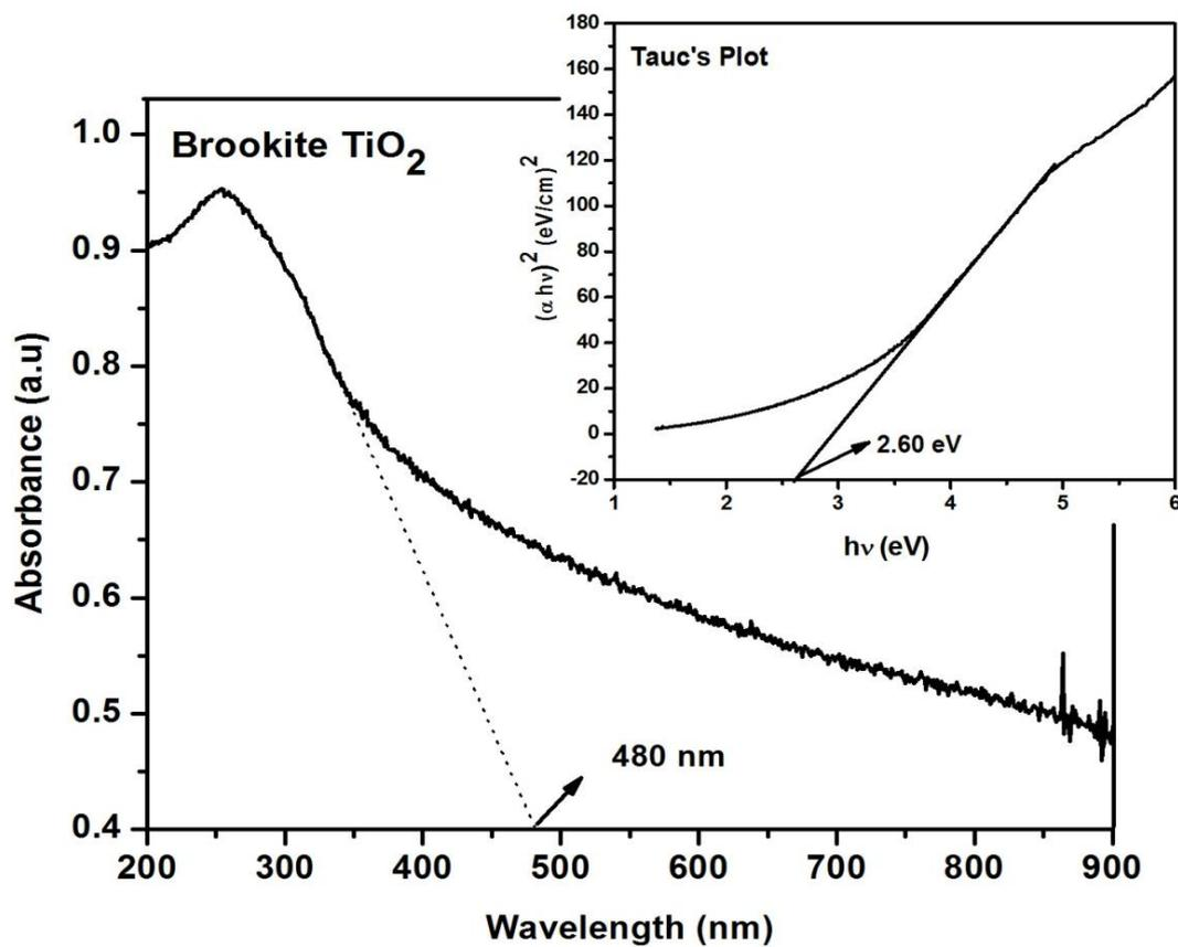
Figure 10: Absorption spectrum and Tauc's plot for Brookite TiO<sub>2</sub>
