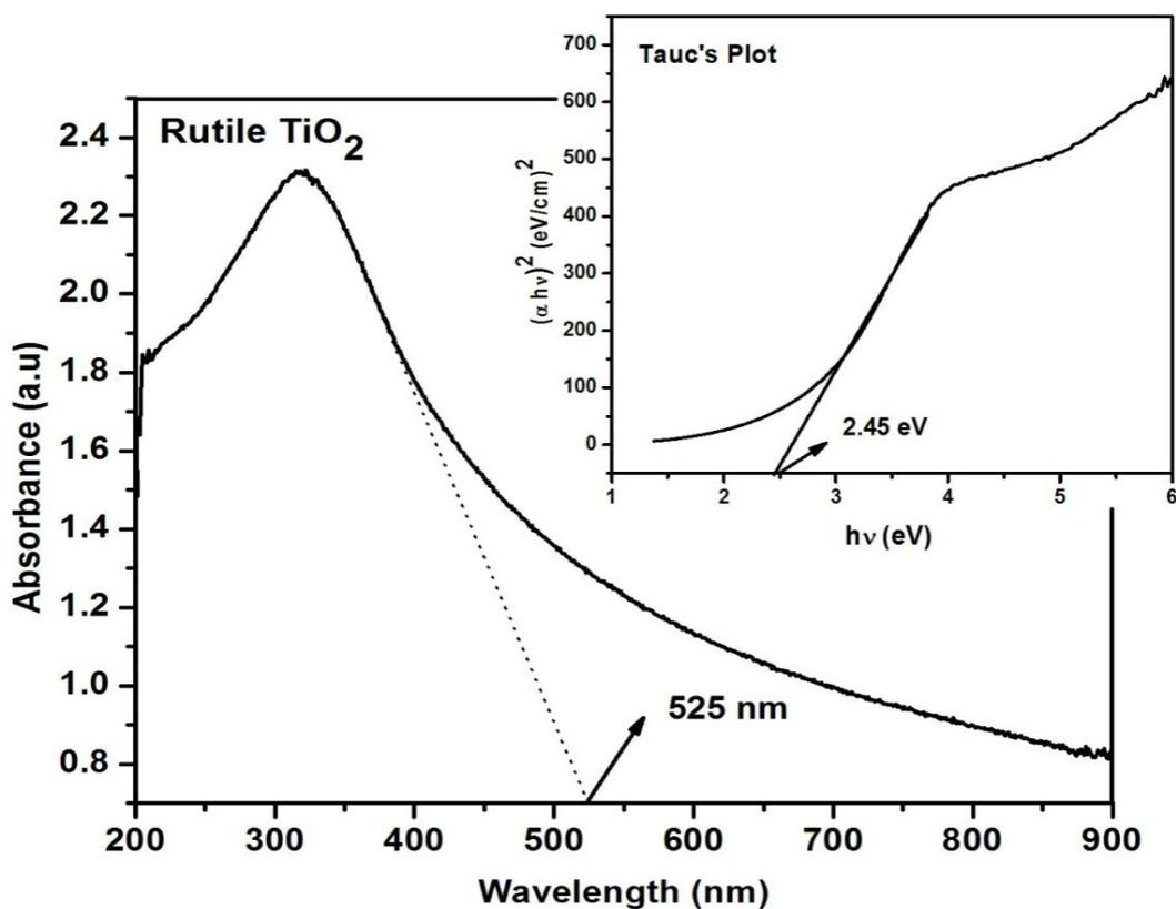
Figure 9: Absorption spectrum and Tauc's plot for Rutile TiO<sub>2</sub>
