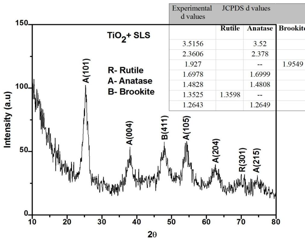
Figure 6: XRD pattern of TiO<sub>2</sub> with SLS
