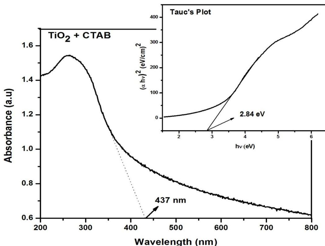
Figure 11: Absorption spectrum and Tauc's plot for TiO<sub>2</sub> with CTAB
