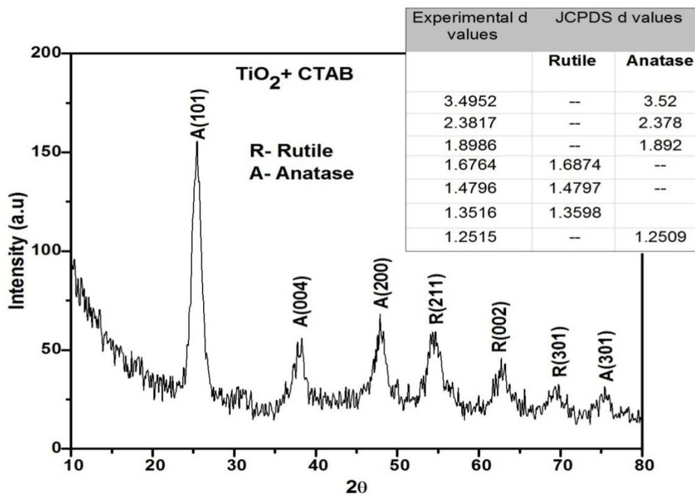
Figure 4: XRD pattern of TiO<sub>2</sub> with CTAB
