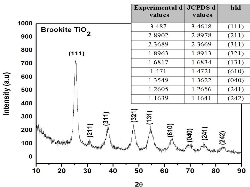
Figure 3: XRD pattern of Brookite TiO<sub>2</sub>
