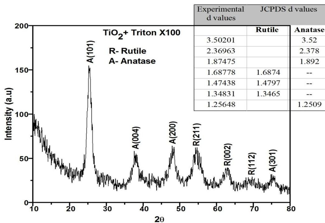
Figure 7: XRD pattern of TiO<sub>2</sub> with Triton X100
