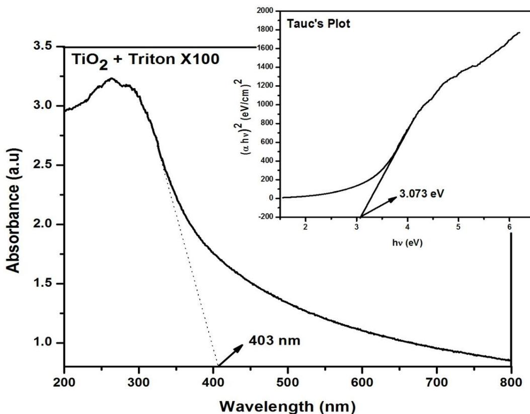
Figure 14: Absorption spectrum and Tauc's plot for  $\text{TiO}_2$  with Triton X100
