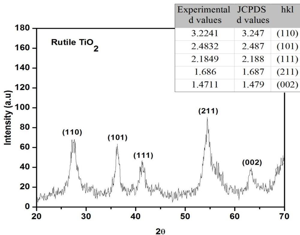
Figure 2: XRD pattern of RutileTiO<sub>2</sub>
