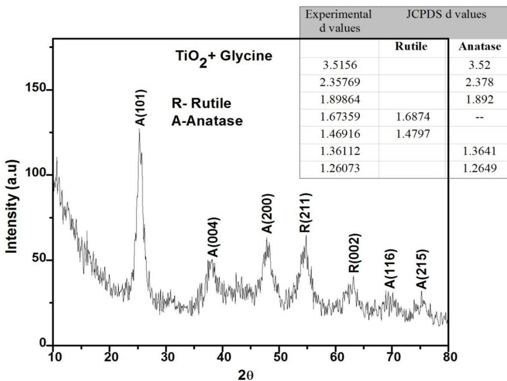
Figure 5: XRD pattern of TiO<sub>2</sub> with glycine
