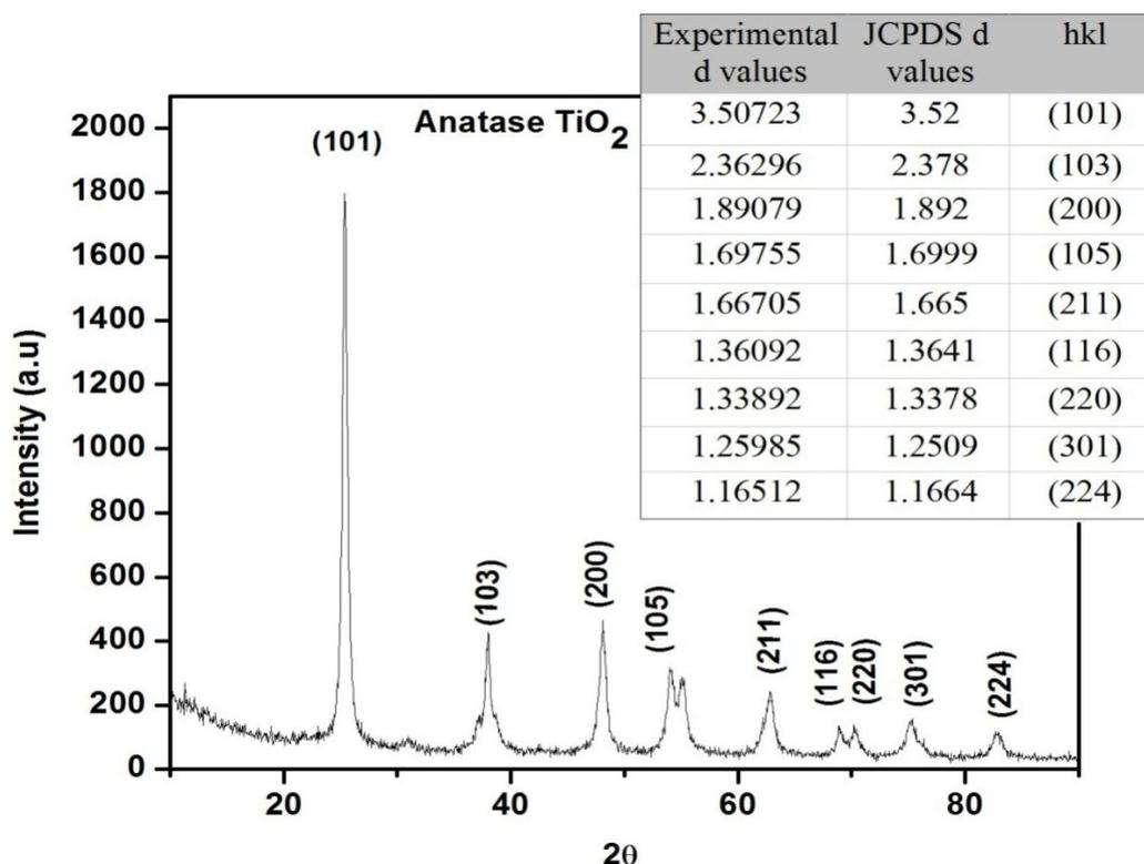
Figure 1: XRD pattern of Anatase  $\text{TiO}_2$  (Sample 1)
