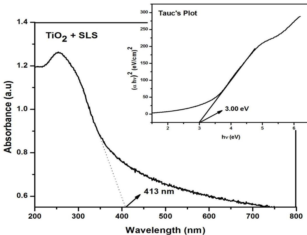
Figure 13: Absorption spectrum and Tauc's plot for  $\text{TiO}_2$  with SLS
