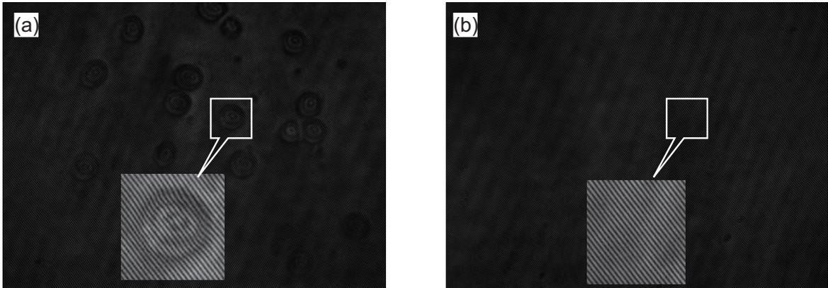
Figure 4.2: Recoded holograms in the case of red blood cells. (a) Object hologram (red blood cells). (b) Background holograms (blood plasma).
