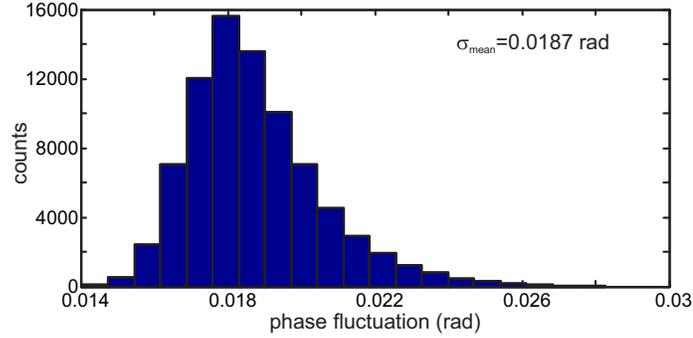
Figure 4.6: Improved temporal phase stability. Histogram of the phase fluctuation obtained for the microscope used for 3D imaging of red blood cells.
