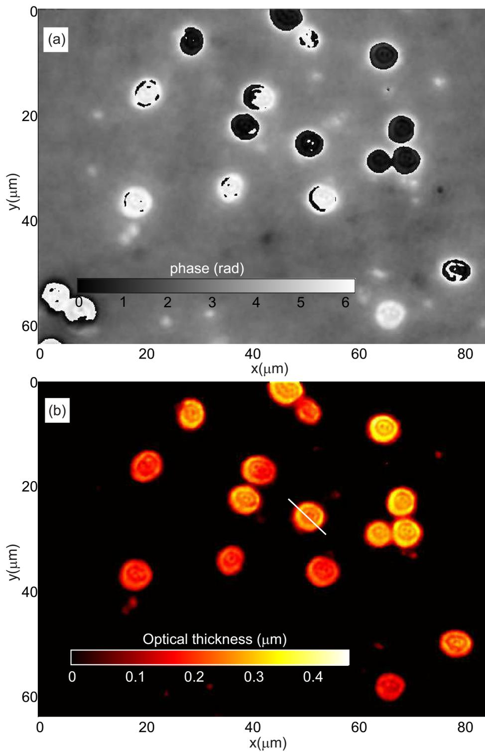
Figure 4.4: Reconstructed profile of red blood cells. (a) Wrapped phase distribution. (b) Optical thickness distribution obtained after phase unwrapping.
