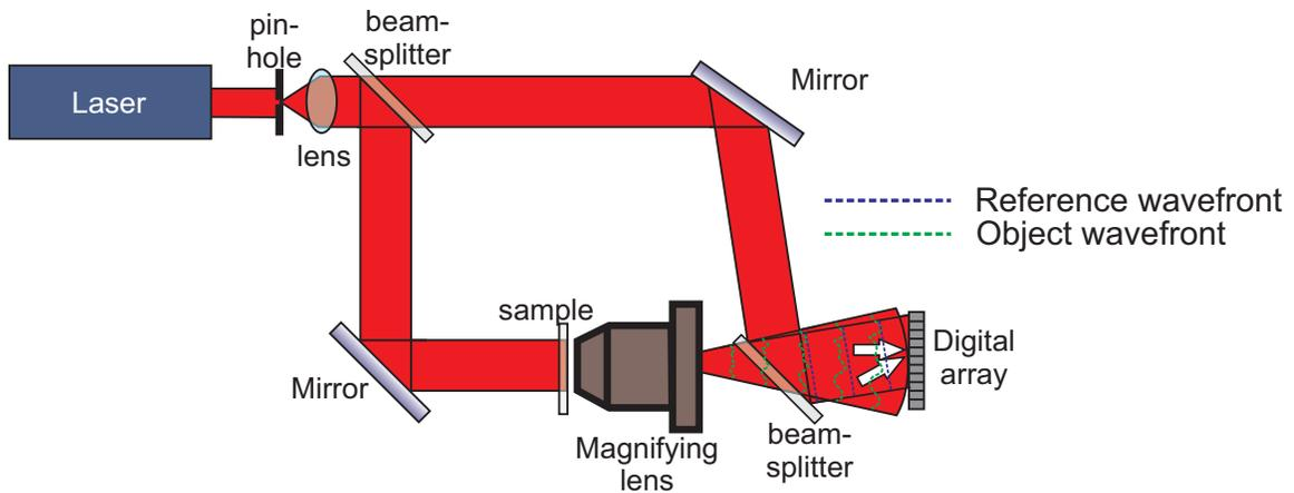
Figure 1.7: Off-axis two-beam DHIM. Detector plane is situated near the image plane of the magnifying lens making the phase retrieval possible by the use of a filtered Fourier transform.
