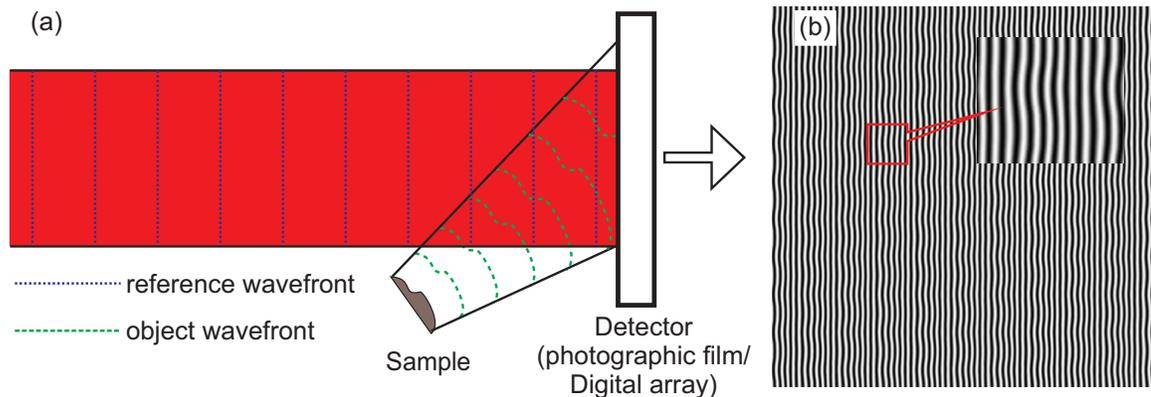
Figure 1.3: (a) Recording of off-axis holograms (b) Hologram resulting from superposition of object and reference wavefronts (object was a distribution of transparent microspheres).
