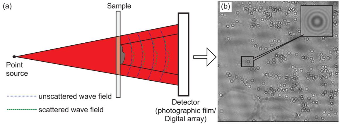
Figure 1.1: (a) Recording geometry for Gabor holograms (on-axis geometry). (b) Hologram resulting from superposition of scattered and unscattered wavefronts at the detector plane (object was a random distribution of transparent microspheres).
