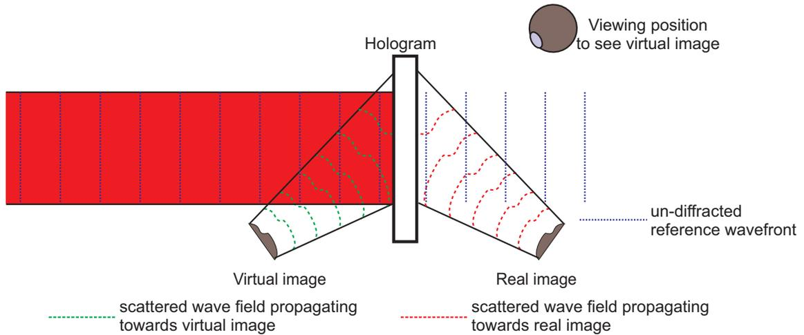
Figure 1.4: Image reconstruction from off-axis holograms
