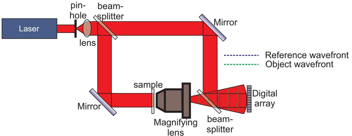
Figure 1.6: On-axis DHIM with a separate reference beam. Here also the detector plane is situated near the image plane of the magnifying lens.
