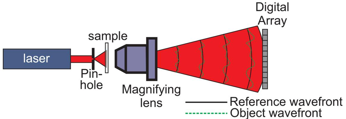
Figure 1.5: Gabor DHIM using a magnifying lens. The detector plane is situated near the image plane of the magnifying lens.
