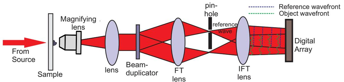
Figure 1.8: Common path Off-axis two-beam DHIM. A separate reference wave is created by spatial filtering of one of the duplicated object wavefronts.
