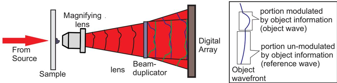
Figure 1.9: Common path off-axis self-referencing DHIM. Portion of the object wavefront un-modulated by the object information act as the reference wave field and the modulated portion act as the object wave field. Angular separation between them is introduced by the beam duplicator.
