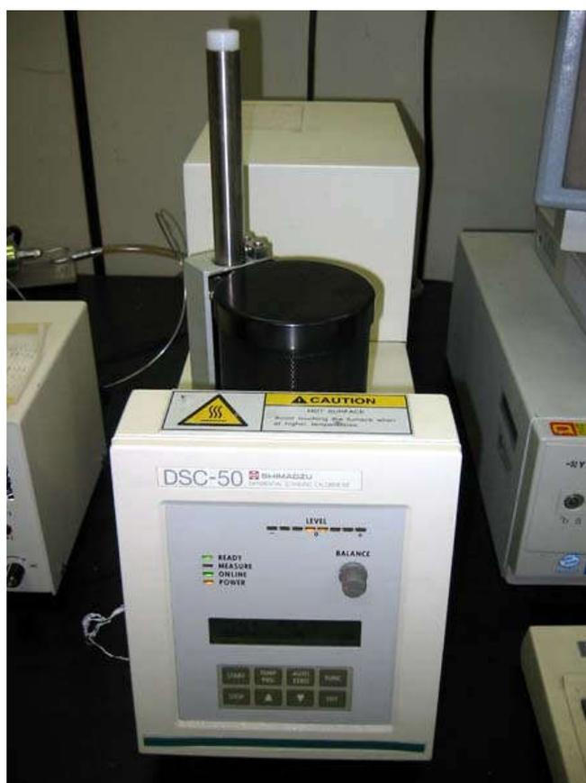
**Fig. 3.10 Shimadzu DSC-50 Differential Scanning Calorimetry**
