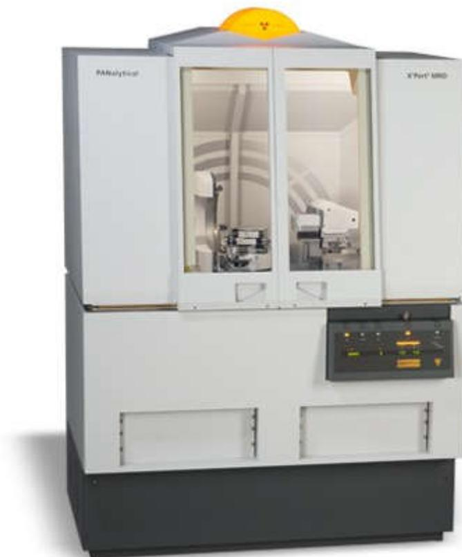
**Fig. 3.8 PANalytical X'pert Pro diffractometer [3.30]**
