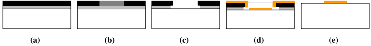
Figure 3.9: Lift-off technique: (a) overlying layer of photoresist (OiR 960), soft baked at 95 °C for 1 minute and (b) exposed to UV light ( \lambda = 365 nm) (c) developed resist with formation of undercut (d) metal deposition on sample (e) lift-off and clean.
