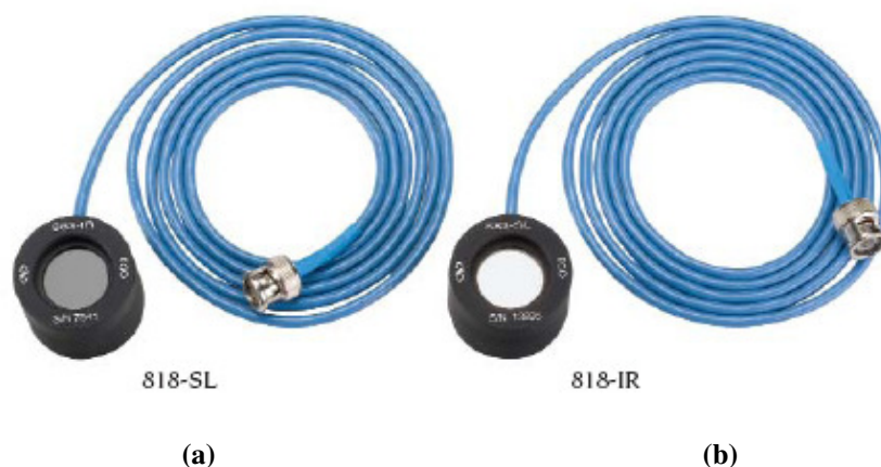
Figure 2.5: Photograph of photodetectors, (a) silicon detector (818-SL) and (b) germanium detector (818-IR), used for the experiment.
