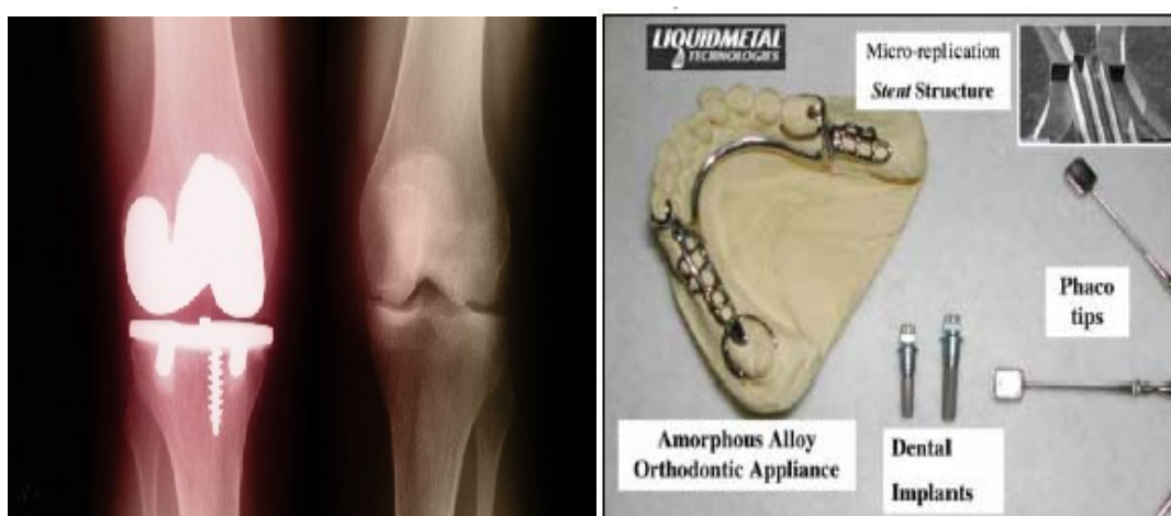
Fig. 1.6: (a) Biodegradable bone implants made of metallic glass, (b) Metallic glass hardware produced by Liquidmetal Technologies [Credit: (a) http://physicsworld.com (b) Liquidmetal Technologies].
