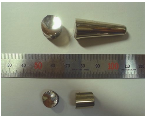
Fig. 1.3: Bulk metallic glass (Source: http://en.wikipedia.org )
