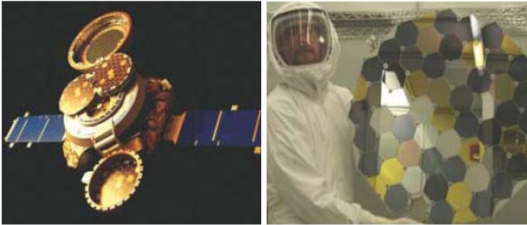
Fig. 1.8: (a) Artist's impression of the Genesis spacecraft in collection mode, opened up to collect and store samples of solar wind particles. (b) Genesis' array, held by Andy Stone of the Jet Propulsion Laboratory, showing the collector materials. [(a) Courtesy of JPL; (b) Courtesy of NASA Johnson Space Center]
