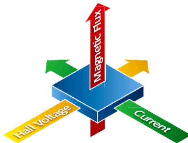
**Fig. 2.15 Illustration of Hall-effect, the hall voltage observed due to the Lorentz force.**
