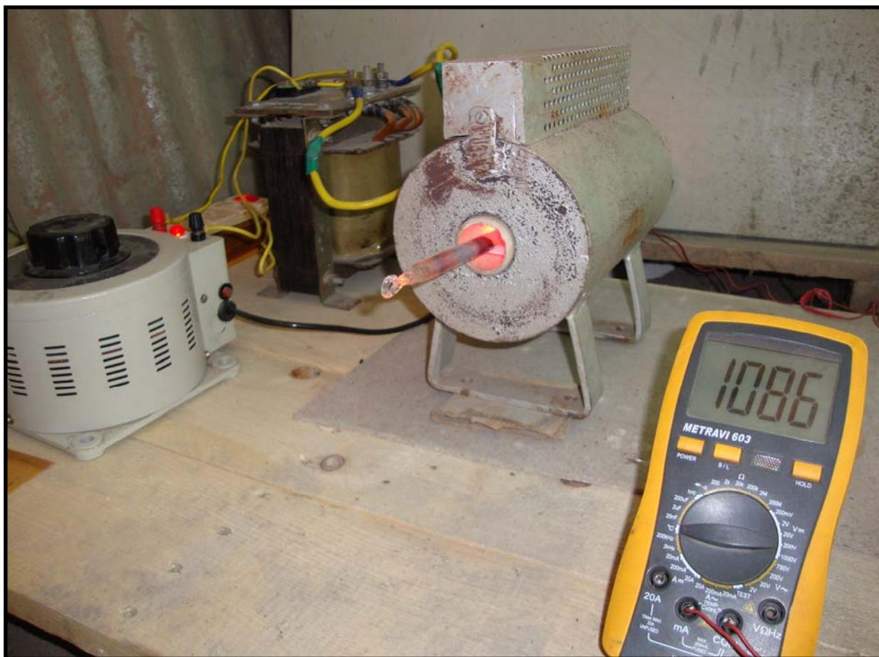
**Fig. 4.2** Photograph of experimental setup for the preparation of CIGS melt, containing the ampoule in the horizontal furnace.
