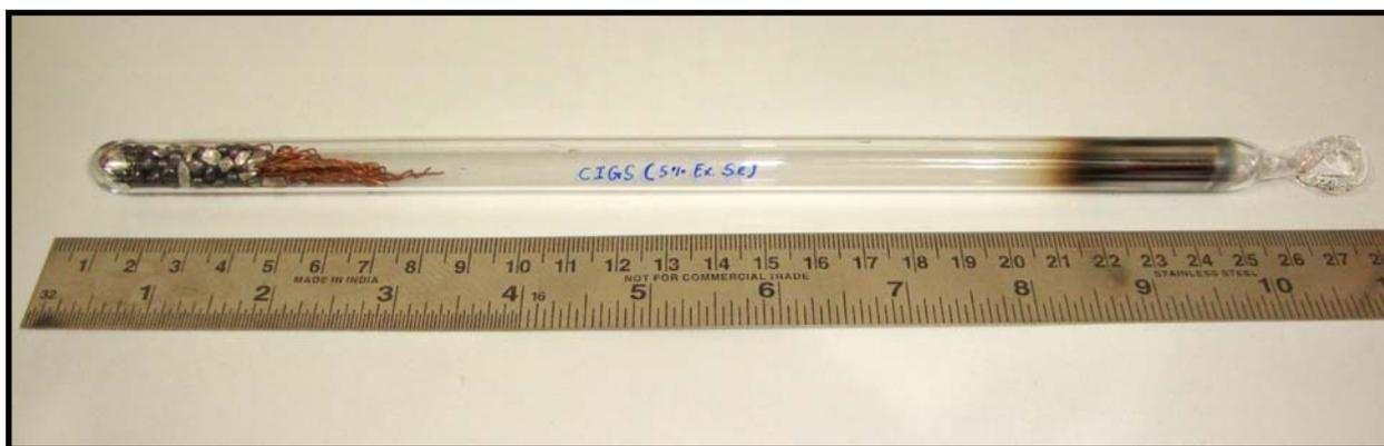
**Fig. 4.1 Vacuum sealed quartz ampoule containing constituent elements of CIGS material with 5 % excess selenium content.**
