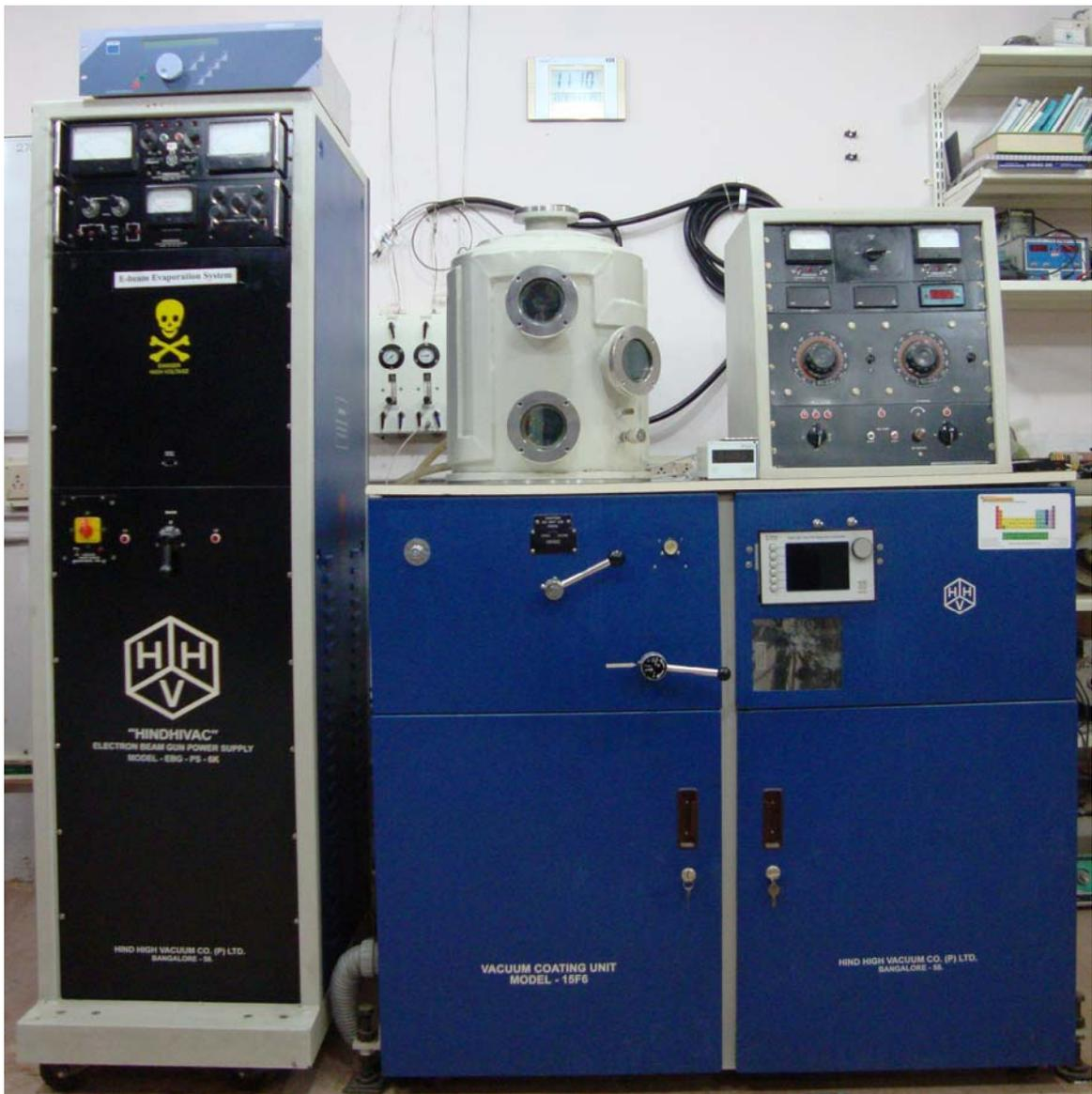
**Figure 2.5: Photograph of the High vacuum coating unit with Thermal evaporation, 2-inch diameter RF magnetron sputtering and 270 ° bend e-beam gun facility.**
