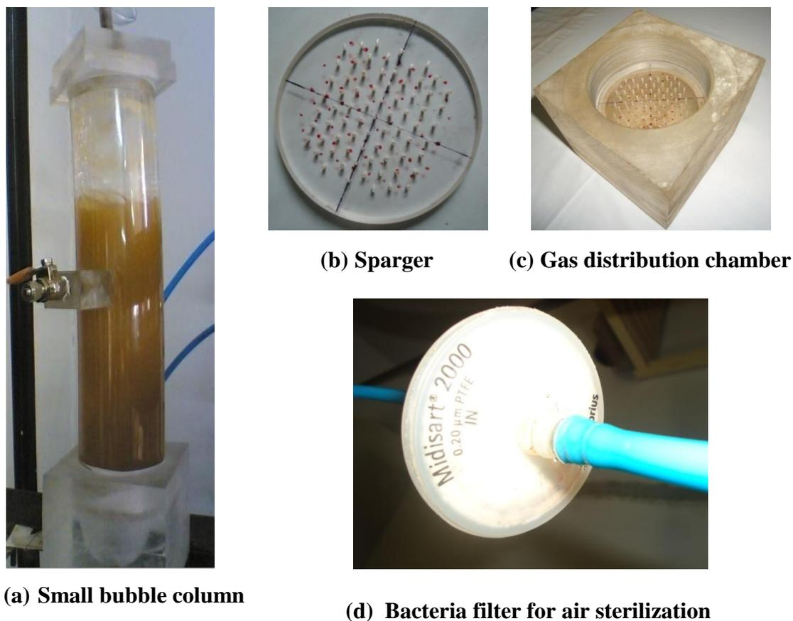
**Fig. 6.5** Snapshots of the small bubble column assembly and its parts
