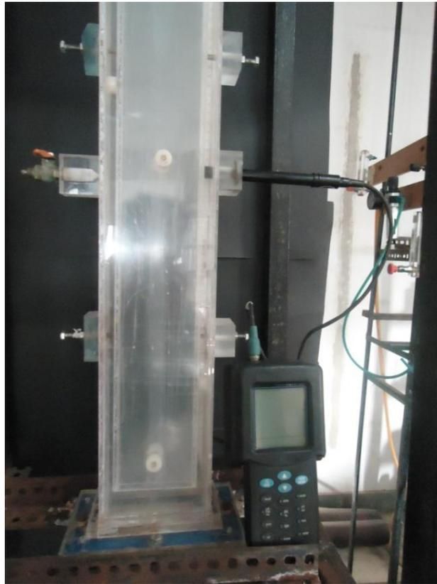
**Fig. 3.6 DO probe inserted in RDTBC and connected to DO meter**
