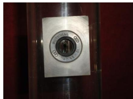
(f) Oil seal in hole for DO probe
