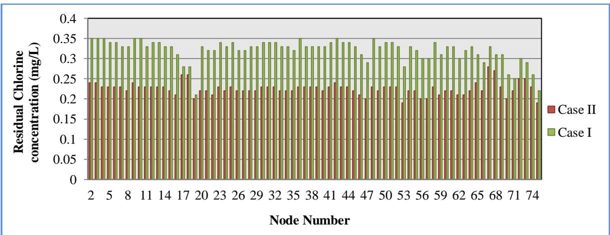
**Fig. 5.30: Variation of residual chlorine concentration at each node after 240 hours for EPS for Case Study 10**
