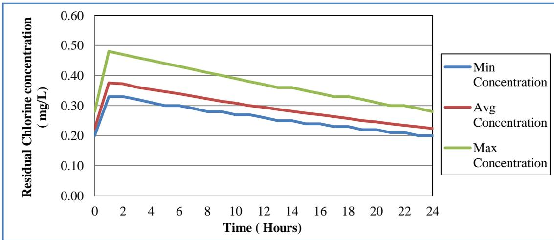
**Fig. 5.18: Minimum, average and maximum concentration of residual chlorine for all nodes (Case II) for Case Study 8**
