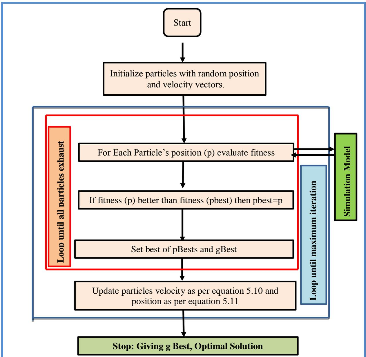
**Fig. 5.34: Coupled Simulation-Optimization Model installed in MATLAB**
