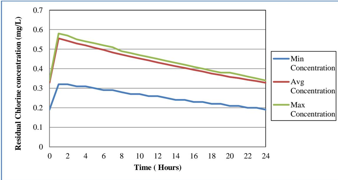
**Fig. 5.5: Minimum, average and maximum concentration of residual chlorine for all nodes (Case I) for Case Study 6**
