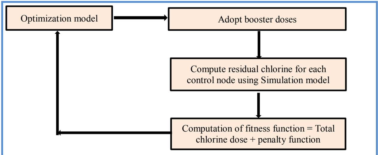
**Fig. 5.33: Simulation Model for coupling with optimization Model.**
