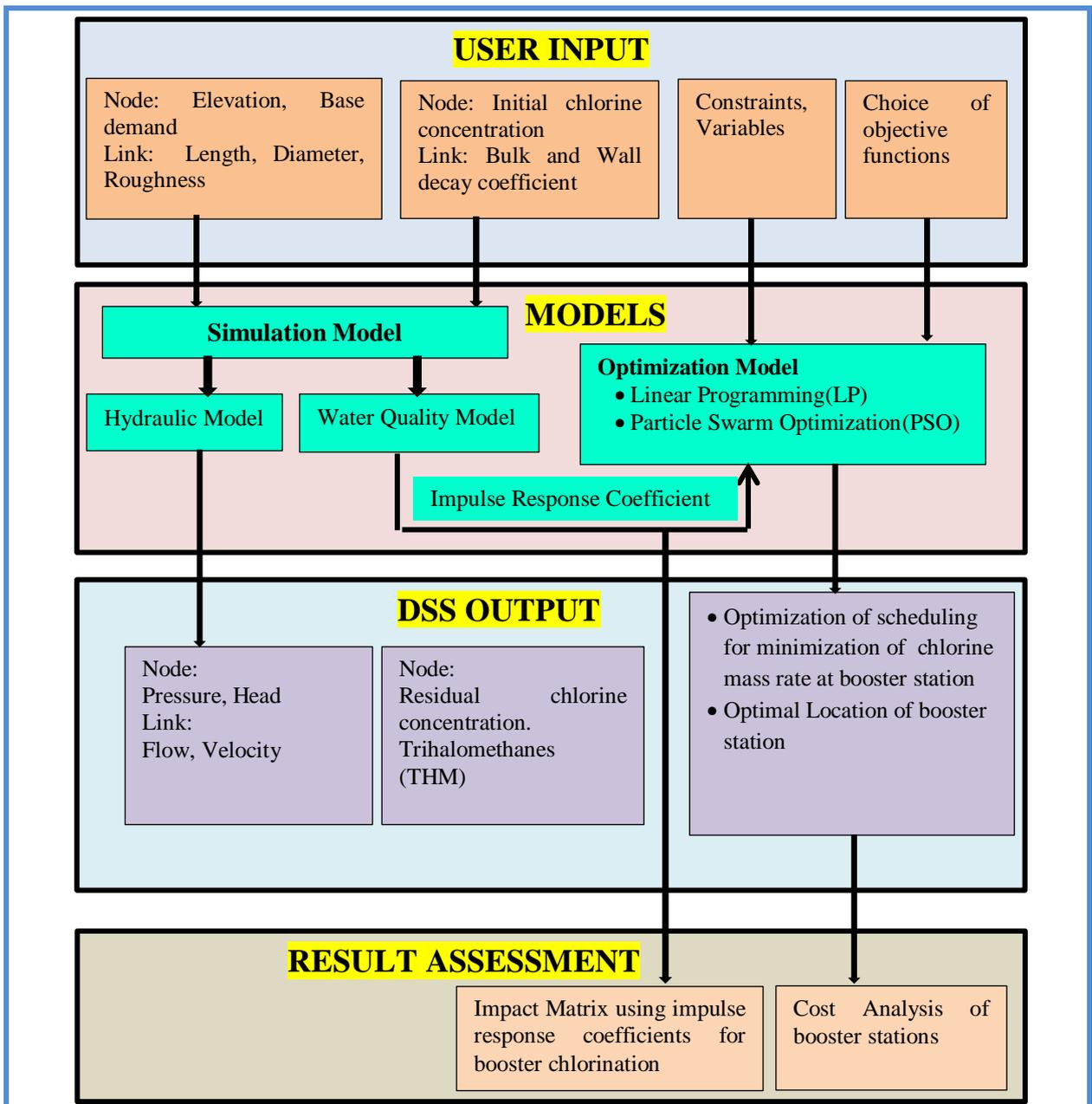
**Fig. 5.39: Decision Support Model (DSM) for management of chlorine disinfection in DWDS**
