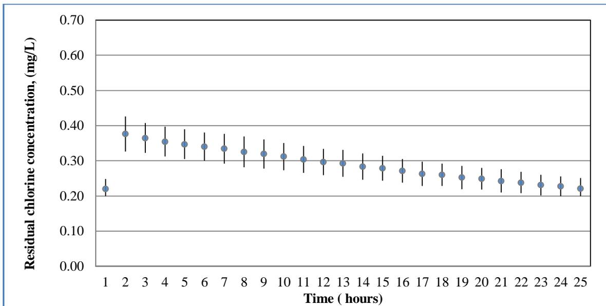
**Fig. 5.8: Average residual chlorine concentration and standard deviation for all nodes (Case II) for Case Study 6**
