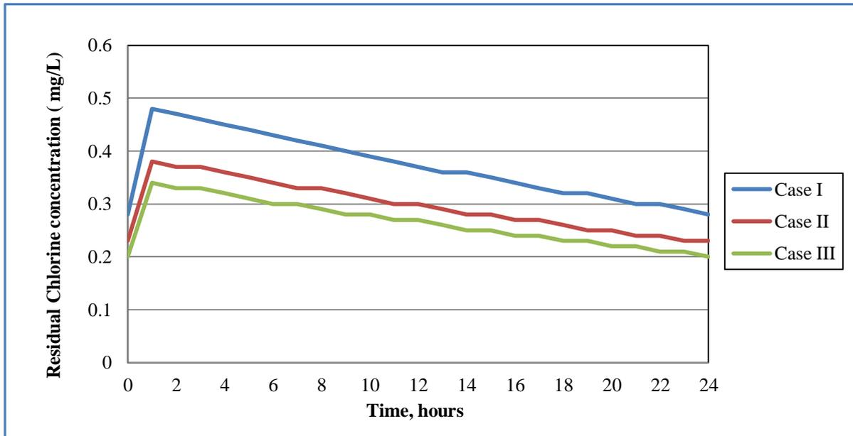
**Fig. 5.16: Tank concentration for residual chlorine (Case I, Case II and Case III) for Case Study 8**
