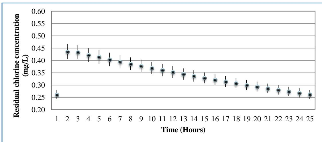
**Fig. 5.19: Average residual chlorine concentration and standard deviation for all nodes. (Case I) for Case Study 8**
