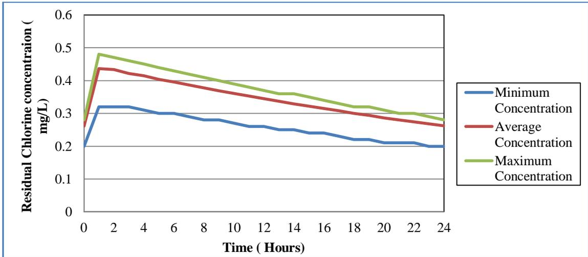
**Fig. 5.17: Minimum, average and maximum concentration of residual chlorine for all nodes (Case I) for Case Study 8**
