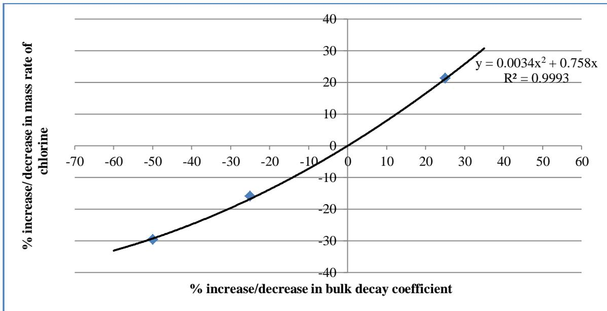
**Fig. 5.9: Percentage variation in total chlorine mass rate for % variation in bulk decay coefficient (Case Study 6).**
