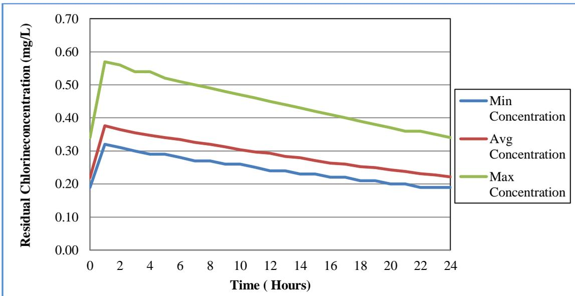
**Fig. 5.6: Minimum, average and maximum concentration of residual chlorine for all nodes (Case II) for Case Study 6**
