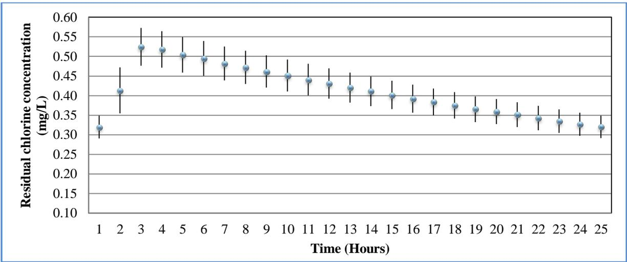
**Fig. 5.28: Average residual chlorine concentration and standard deviation for all nodes (Case I) for Case Study 10**
