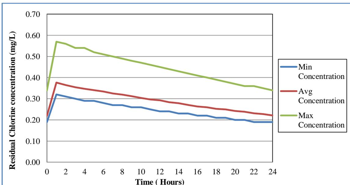
**Fig. 5.12: Minimum, average and maximum concentration of residual chlorine for all nodes. (Case II) for Case Study 7**
