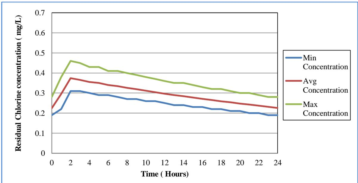
**Fig. 5.27: Minimum, average and maximum concentration of residual chlorine for all nodes (Case II) for Case Study 10**
