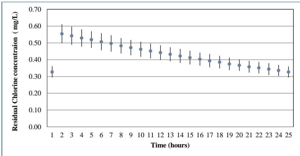
**Fig. 5.13: Average residual chlorine concentration and standard deviation for all nodes (Case I) for Case Study 7**
