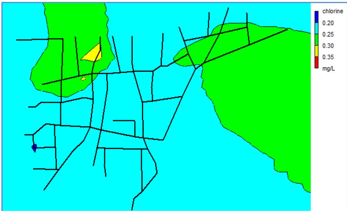
**Fig. 5.23: Contour Plot of residual chlorine for Booster Chlorination (Case III) for Case Study 8.**
