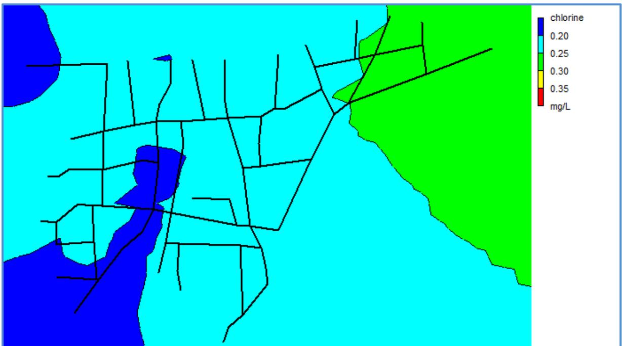
**Fig. 5.22: Contour Plot of residual chlorine for Booster Chlorination (Case II) for Case Study 8.**
