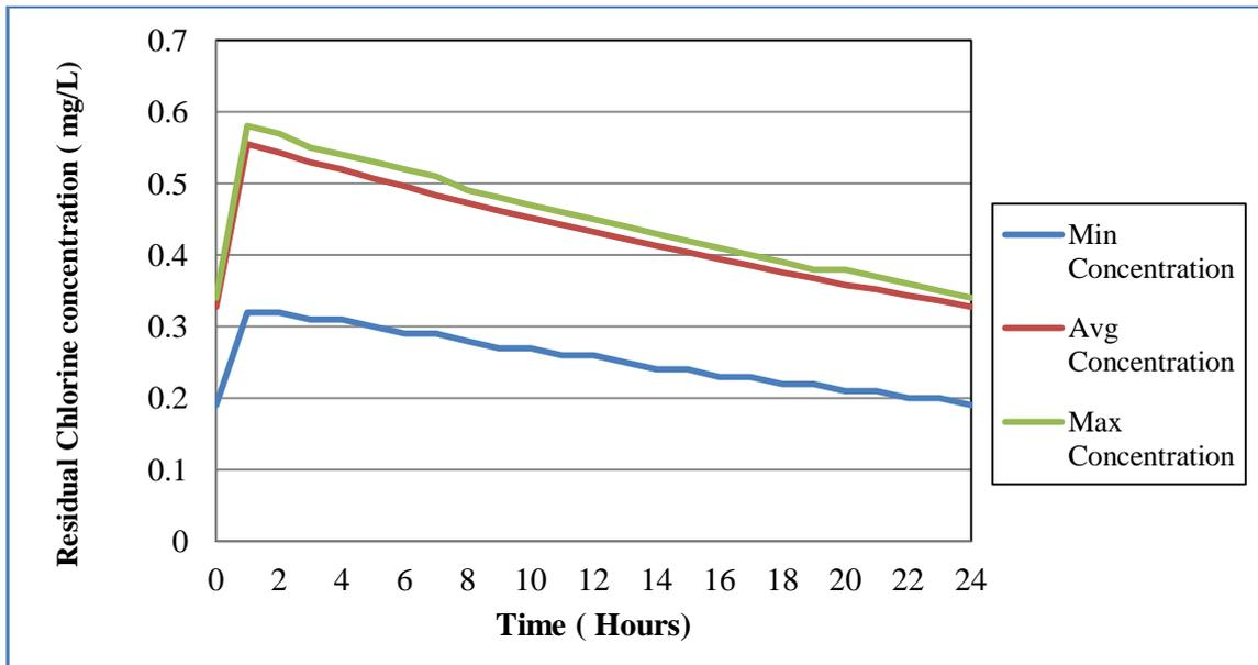
**Fig. 5.11: Minimum, average and maximum concentration of residual chlorine for all nodes (Case I) for Case Study 7**
