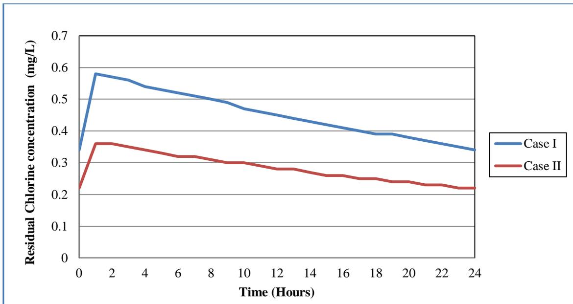
**Fig. 5.10: Tank concentration for residual chlorine (Case I and Case II) for Case Study 7**
