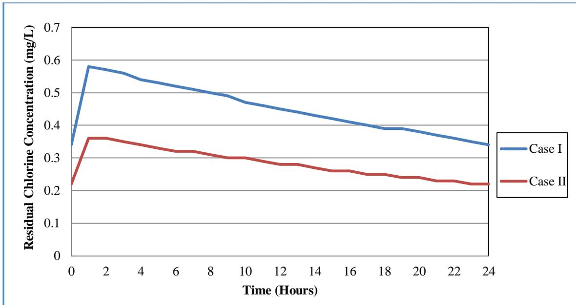
**Fig. 5.4: Tank concentration for residual chlorine (Case I and Case II) for Case Study 6**
