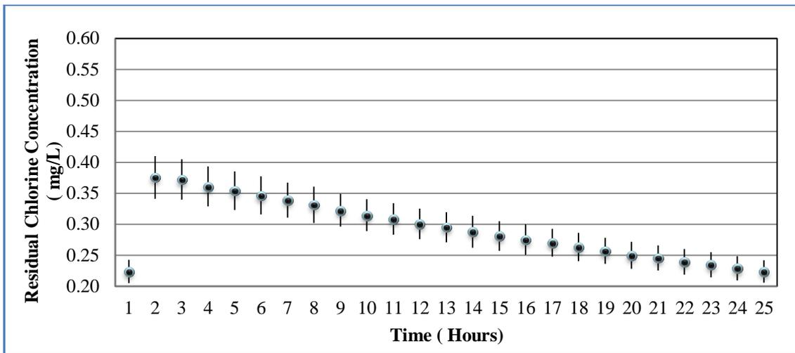
**Fig. 5.20: Average residual chlorine concentration and standard deviation for all nodes. (Case II) for Case Study 8**
