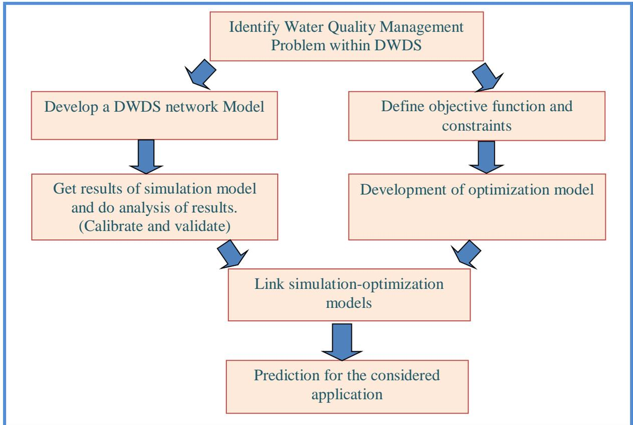
**Fig. 5.1: Steps in the development of simulation-optimization model for water quality management in DWDS.**
