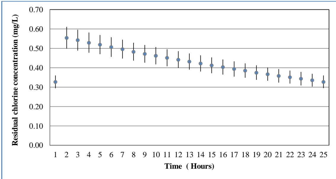
**Fig. 5.7: Average residual chlorine concentration and standard deviation for all nodes (Case I) for Case Study 6**
