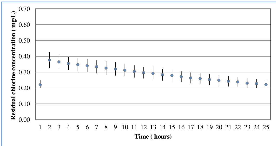
**Fig. 5.14: Average residual chlorine concentration and standard deviation for all nodes (Case II) for Case Study 7**
