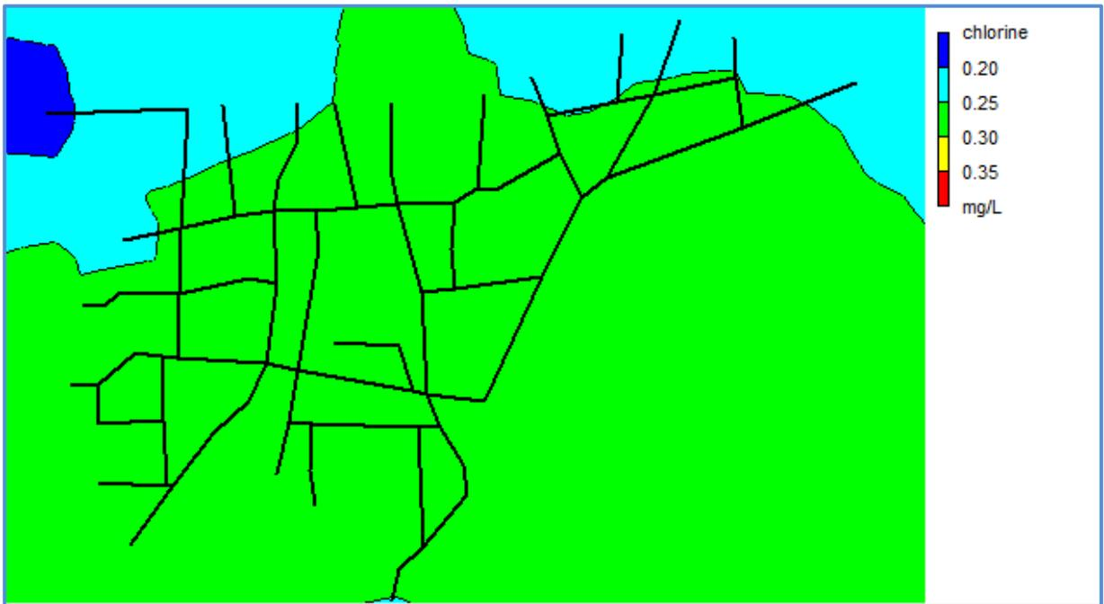
**Fig. 5.21: Contour Plot of residual chlorine for Conventional Chlorination (Case I) for Case Study 8.**
