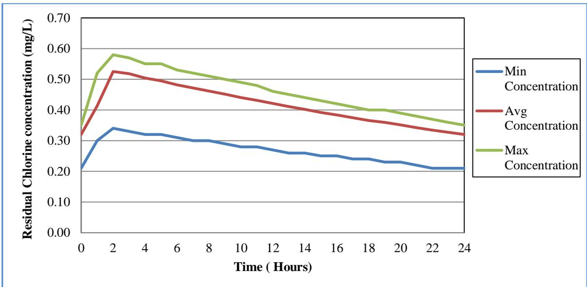
**Fig. 5.26: Minimum, average and maximum concentration of residual chlorine for all nodes (Case I) for Case Study 10**
