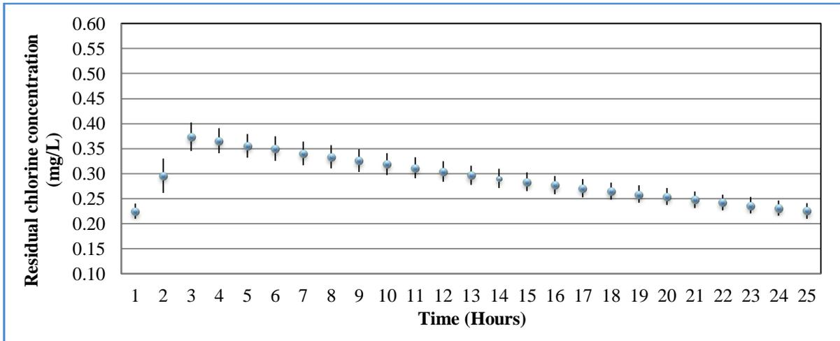
**Fig. 5.29: Average residual chlorine concentration and standard deviation for all nodes (Case II) for Case Study 10**
