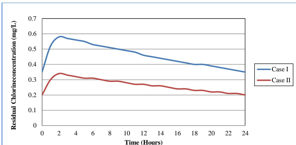
**Fig. 5.25: Tank concentration of residual chlorine (Case I and Case II) for Case Study 10**
