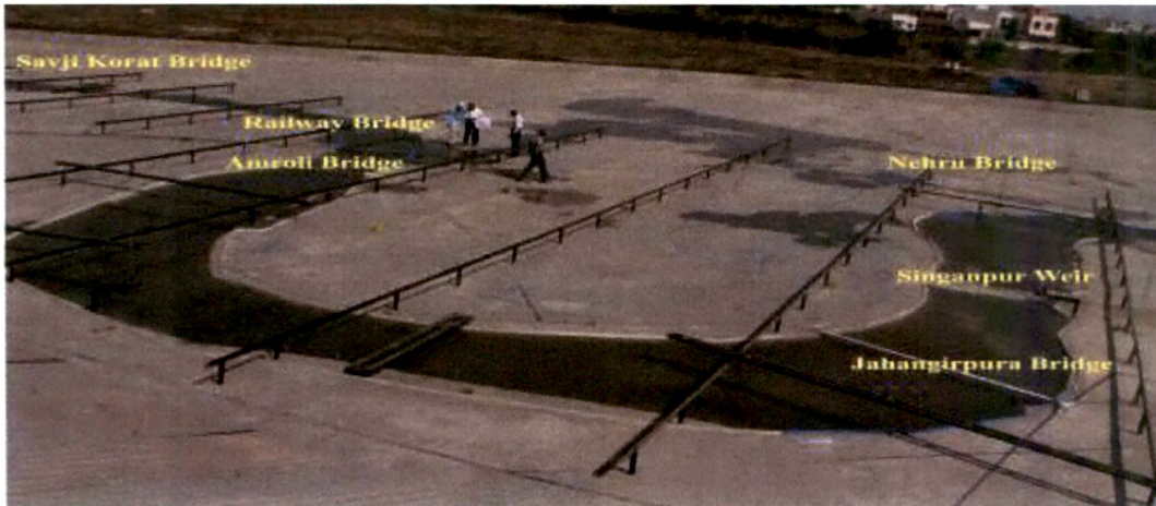
Plate.3.12 Photograph of Distorted Model at GERI, Gotri, Vadodara
