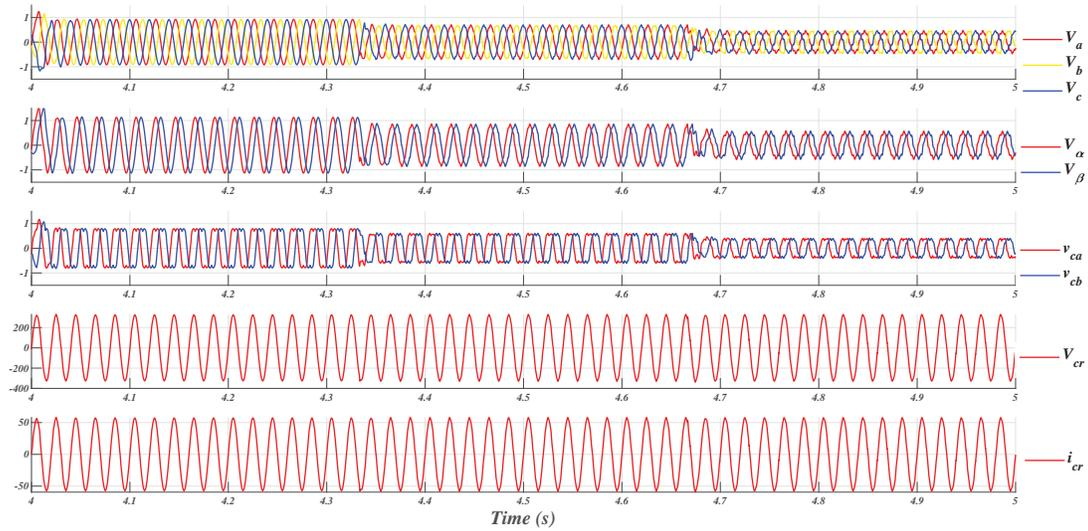
Figure 5.22: Magnified Spectrum of the Control Parameters (Instantaneous Values) of SVPWM Controlled ES, Showing  $R_1$  Load and Step Changes Applied to  $v_g$ .
