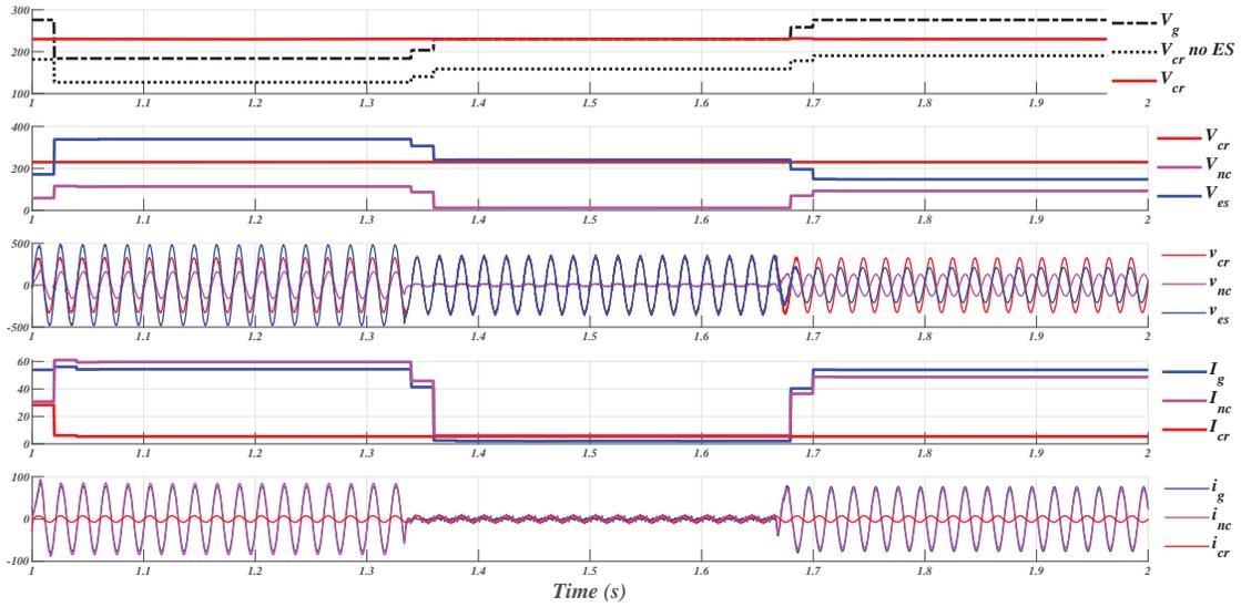
Figure 5.15: Results of *Lead-Lag* (SVPWM) Control having Step Changes in  $v_{cr}$ , for  $R_2$ - $L$  Load.
