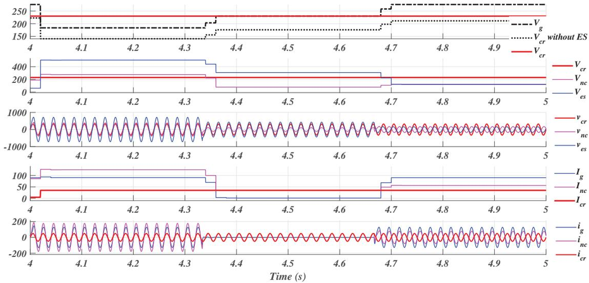
Figure 5.9: Results of *Lead-Lag* (SPWM) Control having Step Changes in  $v_{cr}$ , for  $R_1$  Load.
