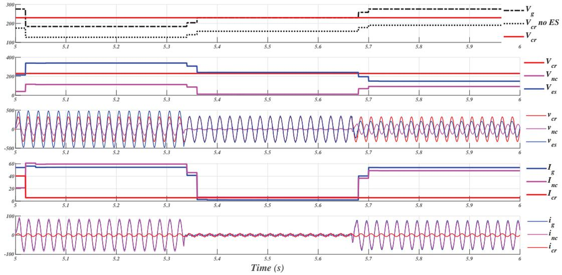
Figure 5.19: Results of *Lead-Lag* (SVPWM) Control having Step Changes in  $v_{cr}$ , for  $R_2$  Load.
