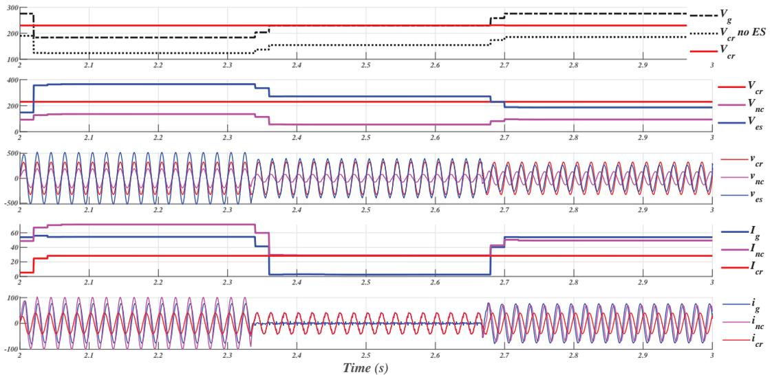
Figure 5.16: Results of *Lead-Lag* (SVPWM) Control having Step Changes in  $v_{cr}$ , for  $R_1$ - $C$  Load.
