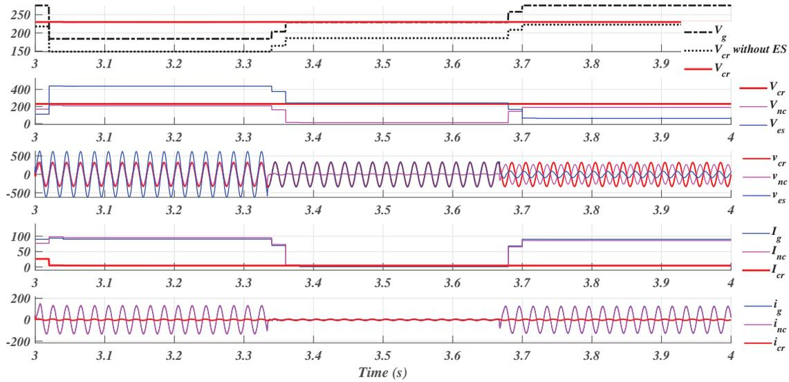
Figure 5.8: Results of *Lead-Lag* (SPWM) Control having Step Changes in  $v_{cr}$ , for  $R_2$ - $C$  Load.
