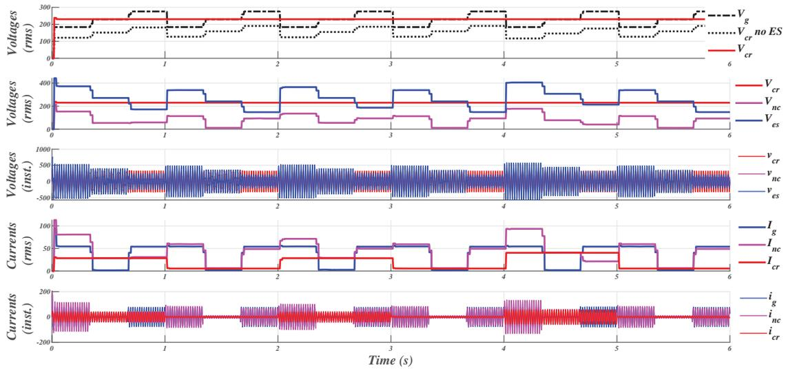
Figure 5.13: Results of *Lead-Lag* (SVPWM) Control having Step Changes Applied to  $v_g$  and Load.
