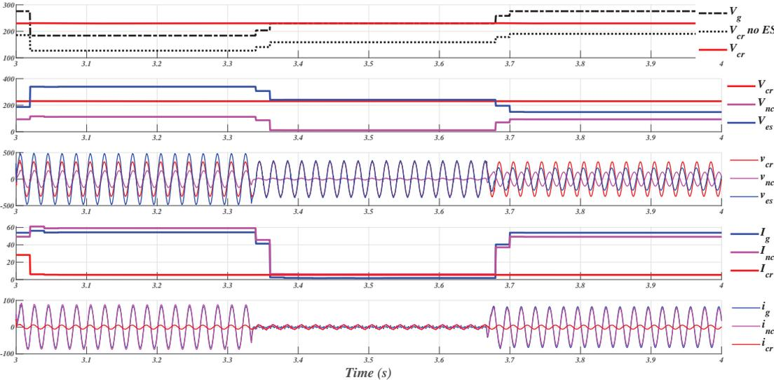
Figure 5.17: Results of *Lead-Lag* (SVPWM) Control having Step Changes in  $v_{cr}$ , for  $R_2$ - $C$  Load.
