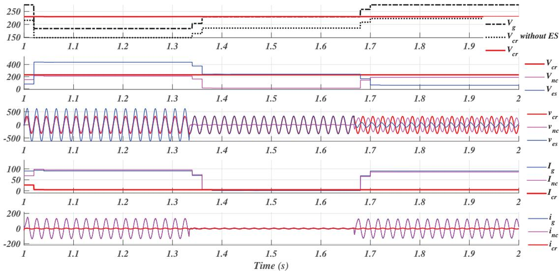
Figure 5.6: Results of *Lead-Lag* (SPWM) Control having Step Changes in  $v_{cr}$ , for  $R_2$ - $L$  Load.
