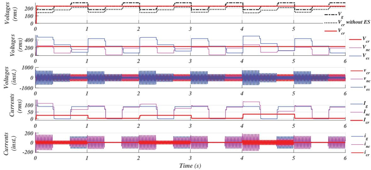
Figure 5.4: Results of *Lead-Lag* (SPWM) Control having Step Changes Applied to  $v_g$  and Load.
