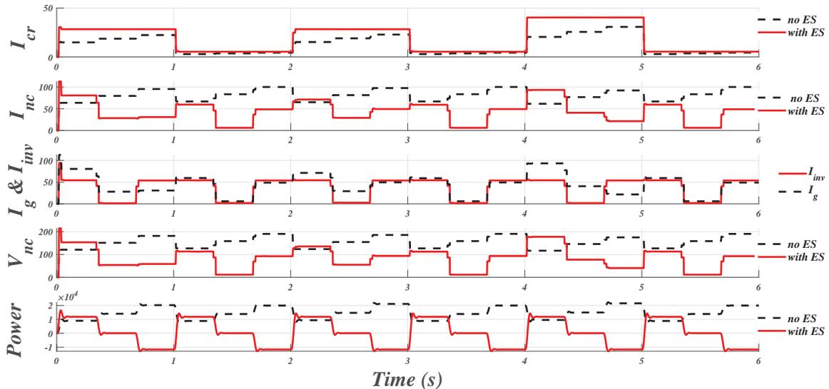
Figure 5.20: Results (RMS values) of *SVPWM* Controlled *ES*, using *Lead-Lag* Compensator, being Compared with the Scenario of Absence of *ES*, in the presence of Step Changes Applied to  $v_g$  and Load.
