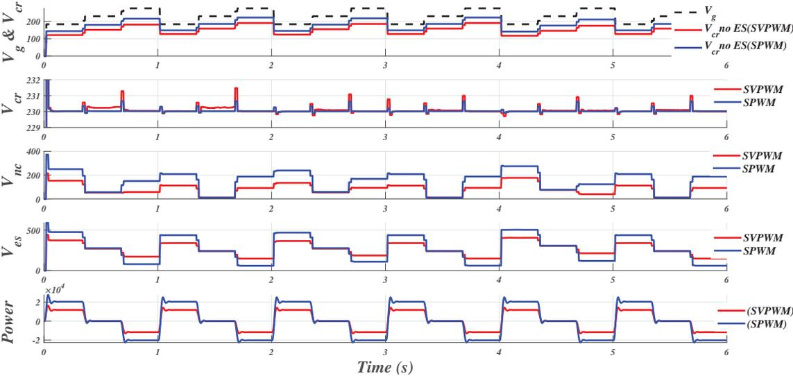
Figure 5.24: Comparative Results (RMS values of Voltages) of *SVPWM* and *SPWM* Controlled *ES*, using *Lead-Lag* Compensator, having Step Changes Applied to  $v_g$  and Load.
