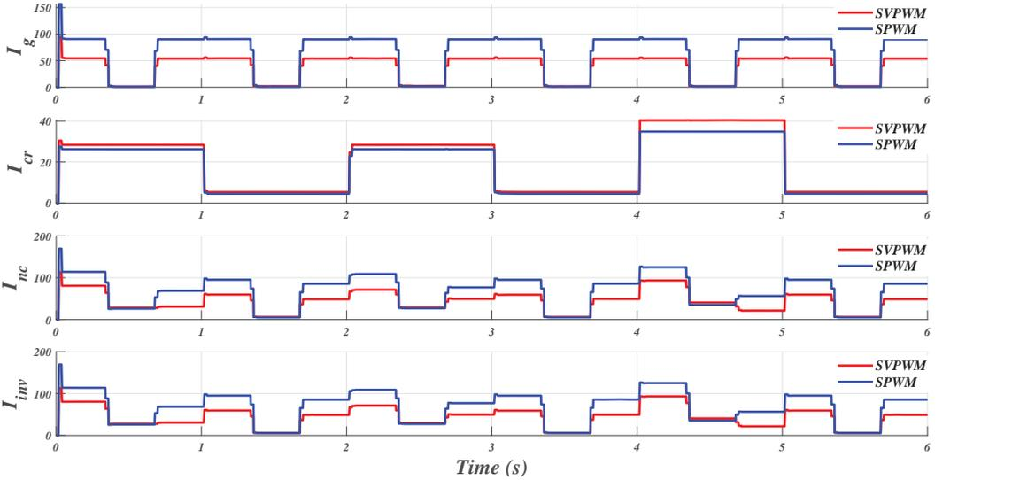
Figure 5.25: Comparative Results (RMS values of Currents and Power) of *SVPWM* and *SPWM* Controlled *ES*, using *Lead-Lag* Compensator, having Step Changes Applied to  $v_g$  and Load.
