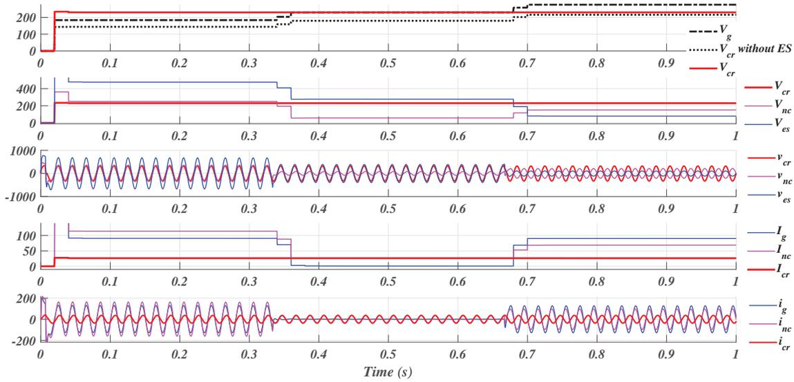
Figure 5.5: Results of *Lead-Lag* (SPWM) Control having Step Changes in  $v_{cr}$ , for  $R_1$ - $L$  Load.
