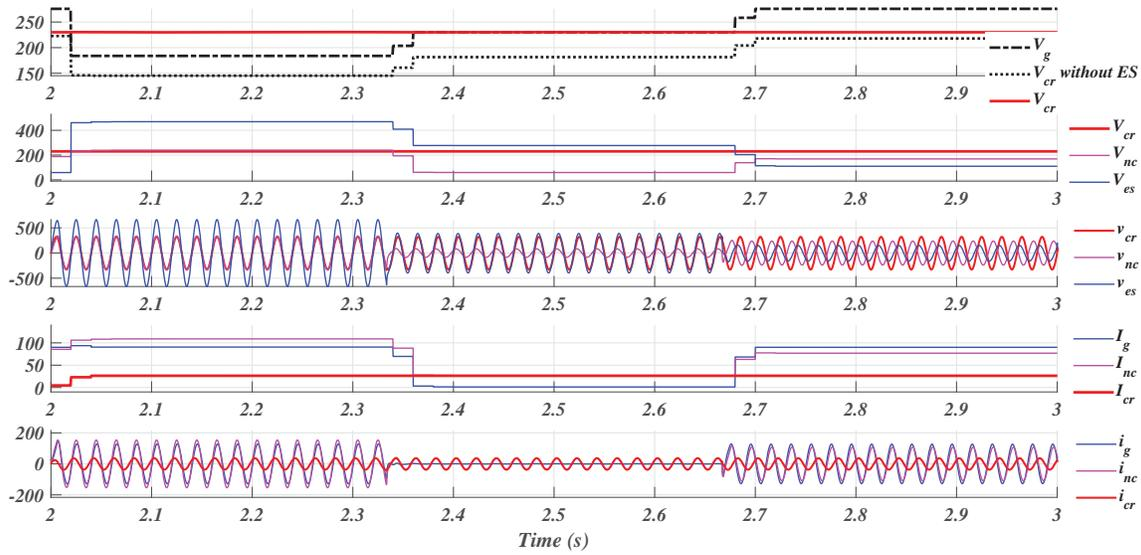
Figure 5.7: Results of *Lead-Lag* (SPWM) Control having Step Changes in  $v_{cr}$ , for  $R_1$ - $C$  Load.
