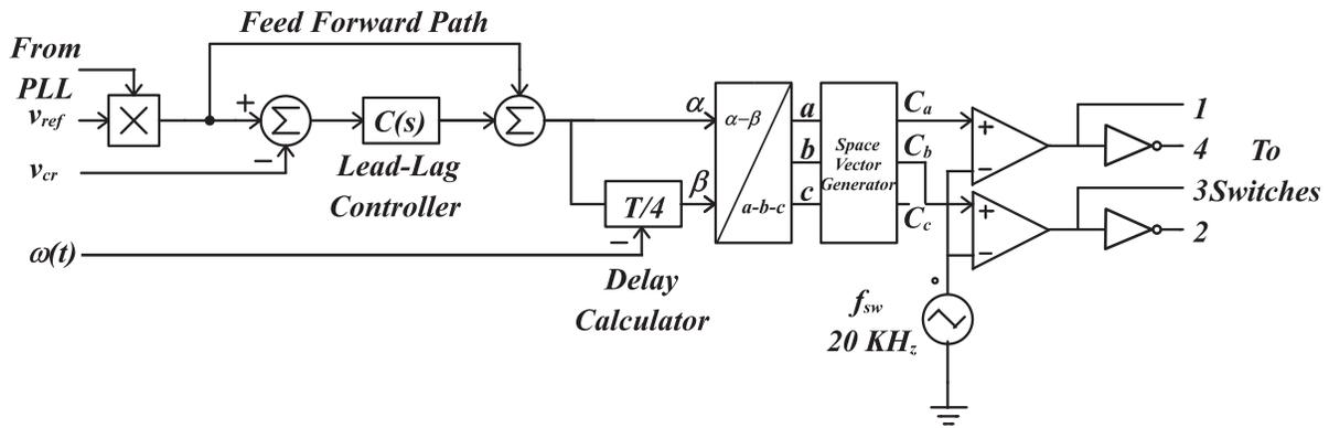
Figure 5.12: *SVPWM* Controlled *ES* using *Lead-Lag* Compensator.
