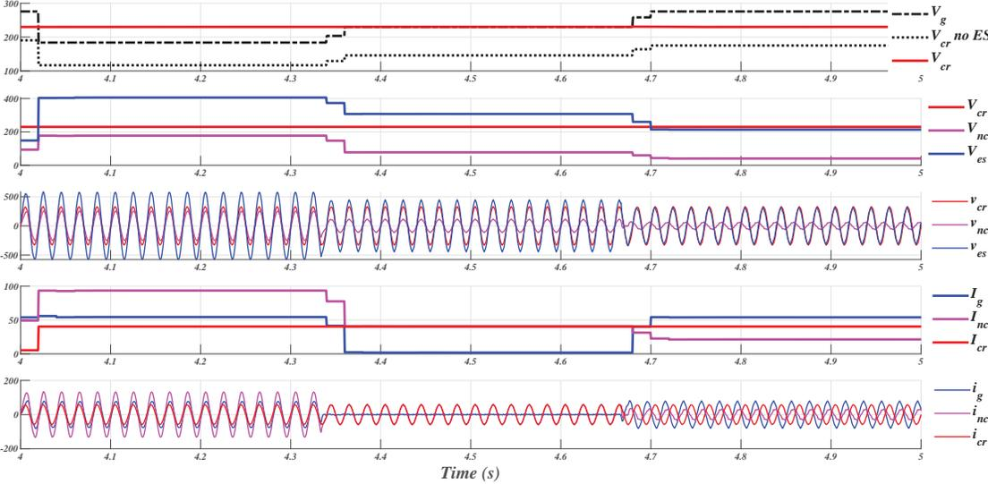
Figure 5.18: Results of *Lead-Lag* (SVPWM) Control having Step Changes in  $v_{cr}$ , for  $R_1$  Load.
