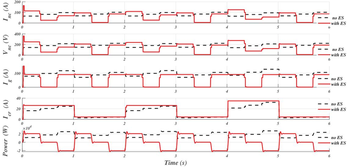
Figure 5.11: Comparison of Results of *Lead-Lag* Controlled *ES* and that with no *ES*, under the influence of Step Changes in  $v_g$  and Load.
