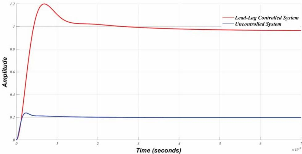
Figure 5.2: Step Response of the Uncontrolled System, and that being Controlled by a *Lead-Lag* Compensator.
