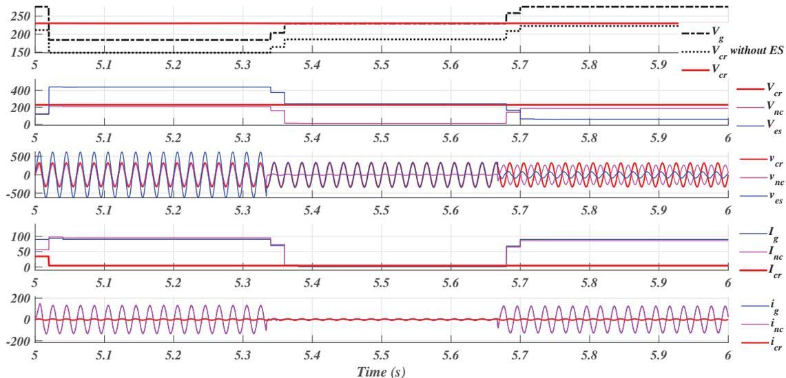
Figure 5.10: Results of *Lead-Lag* (SPWM) Control having Step Changes in  $v_{cr}$ , for  $R_2$  Load.
