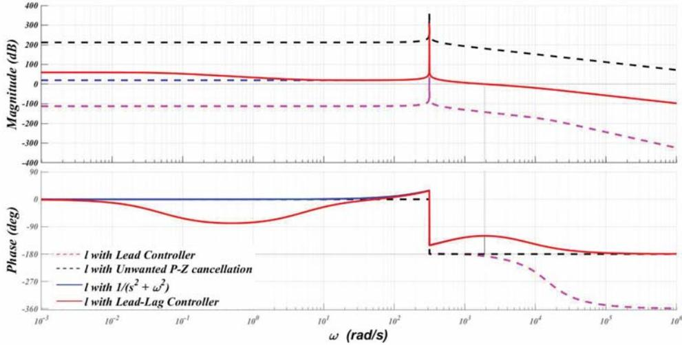
Figure 5.1: Frequency Response plot of *Lead-Lag* Controller, while Evolving through its Design.
