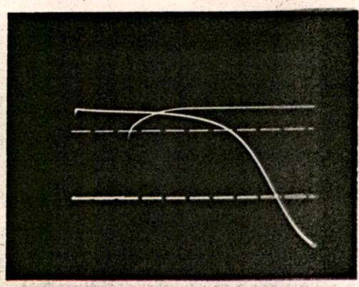
(E) SI Voltage measured across the power frequency testing transformer. (divider ratio = 1465)
