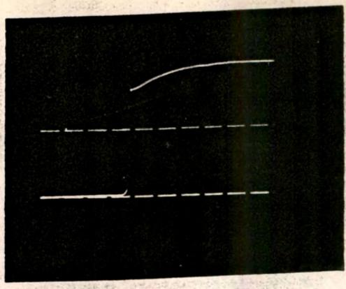
(B) SI Voltage measured at the power frequency terminal of the rod-rod gap. (Divider ratio = 1465)
