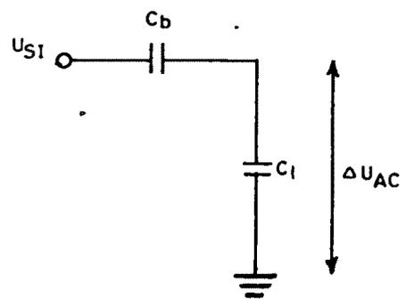
Equivalent circuit for calculating  $\Delta U_{AC}$
