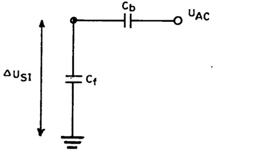
Equivalent circuit for calculating  $\Delta U_{SI}$
