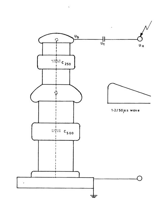
Figure - A1: Circuit for measurement of self capacitance of Transfomer
