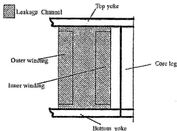
Figure 2.11: Leakage flux path
