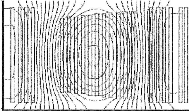
Figure 2.8: Generated Axial and Radial Fluxes in a Shell Type Transformer
