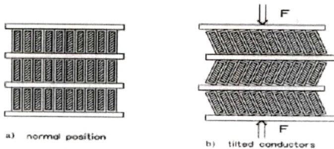
Figure 2.10: Axial forces due to radial field
