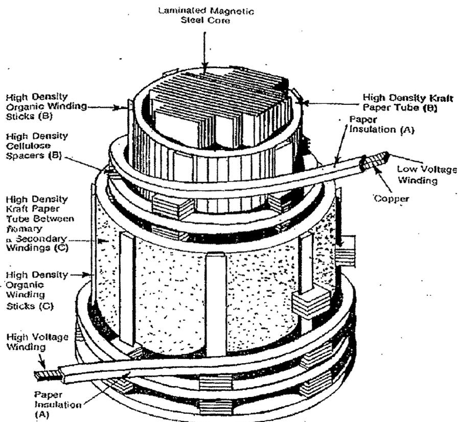
Figure 2.15: Internal layout of Transformer insulation system
