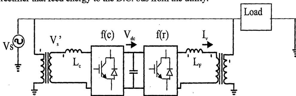
Fig 3.4 Circuit representing DC bus fed by Inverter
