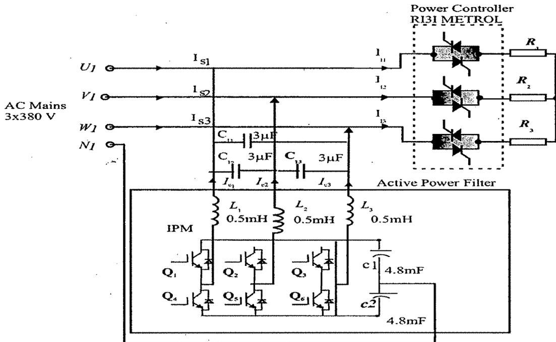
Fig 3.9 Three-Phase Active Power Filter Test Circuit
