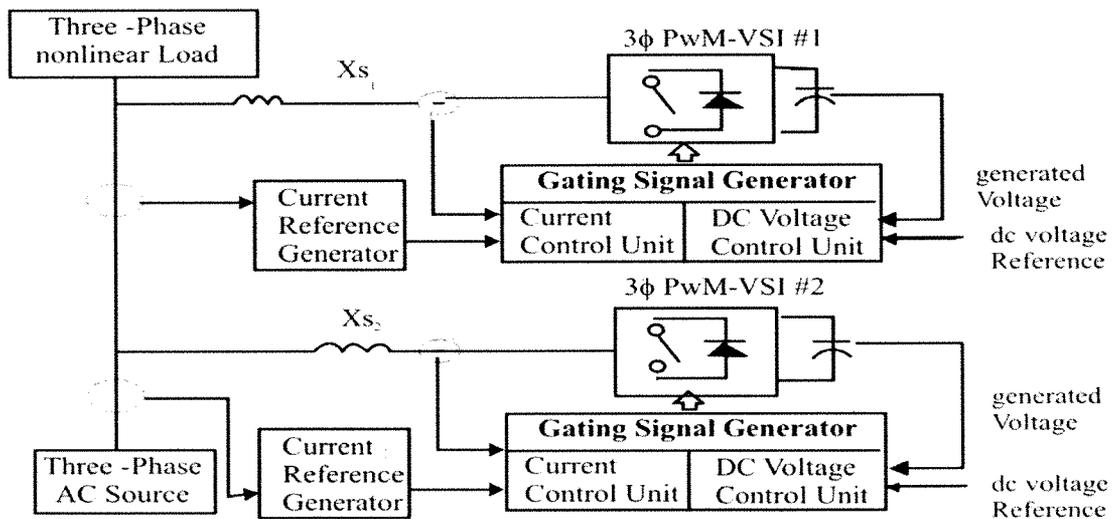
**Fig 3.25 APF Configuration: TWO VSI in Cascade**
