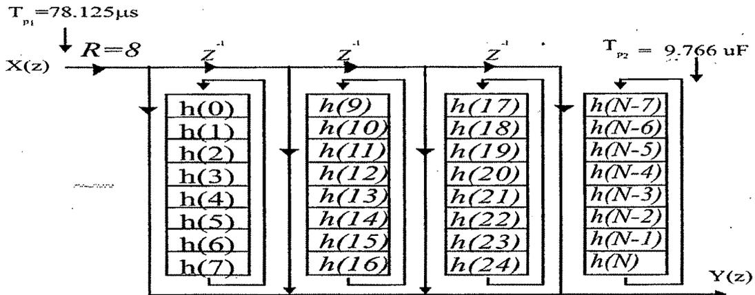
Fig 3.32 Poly phase Interpolator
