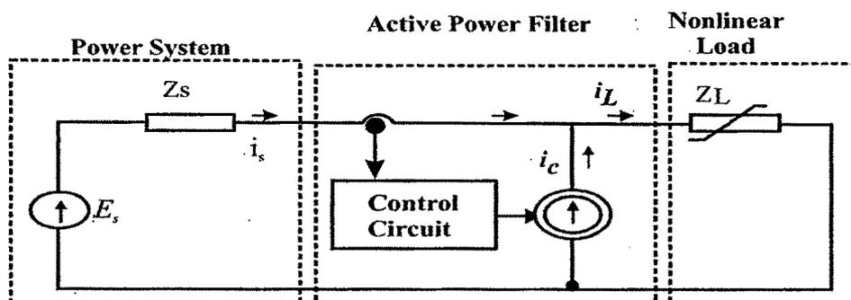
Fig 3.30 (b) Harmonic Compensation Circuit with current-fed APF with feedback
