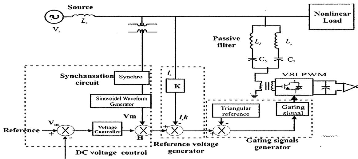
**Fig 3.11 Hybrid APF: Topology & Associated Control Scheme**
