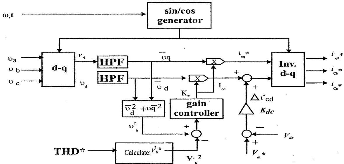
Fig 3.14: Control Block Diagram of APF
