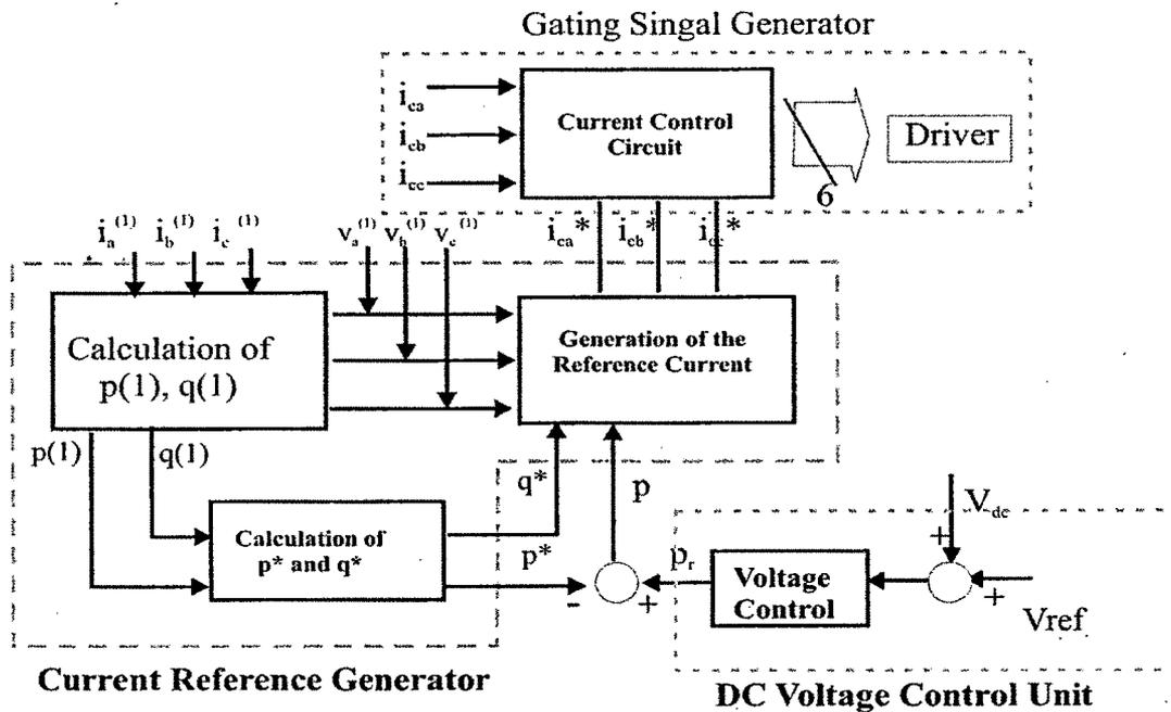
Fig 3.26 Block Diagram of APF Control System
