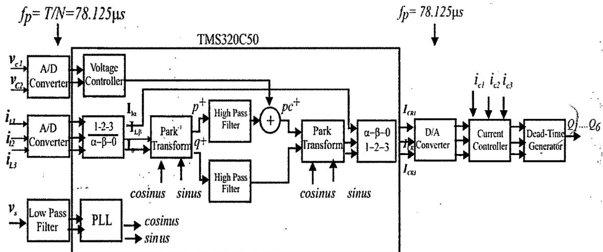
Fig. 3.8 Simplified Block Diagram for the APF Control Algorithm
