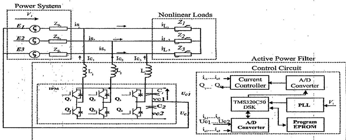
Fig 3.7 Simplified Block diagram of Active Power Compensation Circuit
