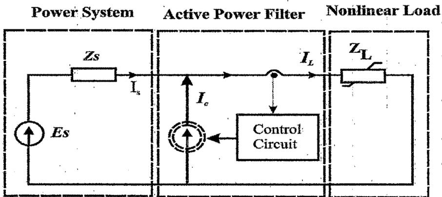
Fig 3.6 Harmonic Compensation circuit with current-fed APF
