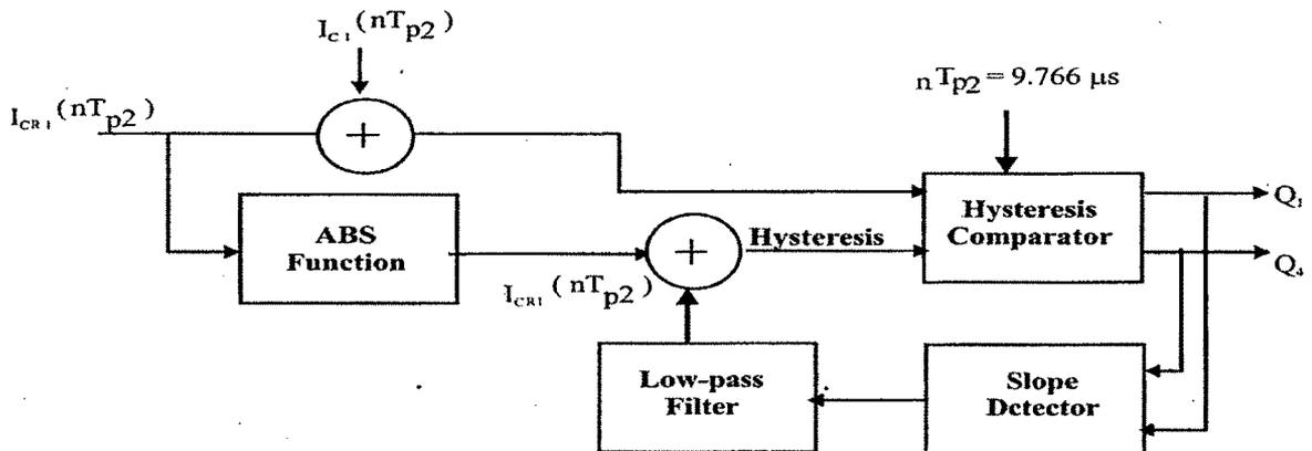
Fig 3.33 Hysteresis Current Controller Algorithm
