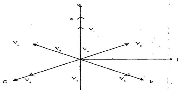
Fig 3.28 Regions of Inverter Output Voltage
