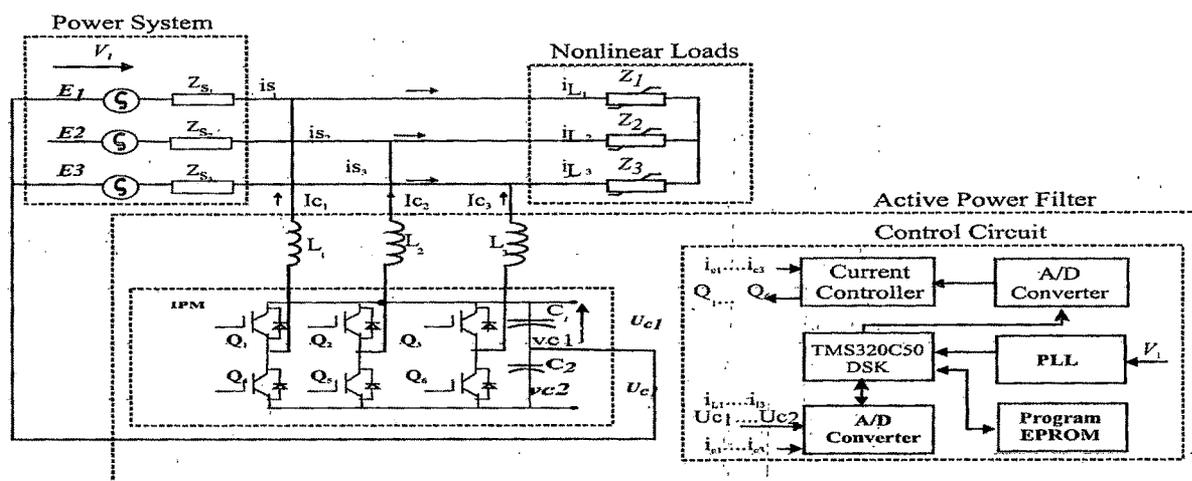
Fig 3.31 Simplified Block Schematic of Current-Fed APF
