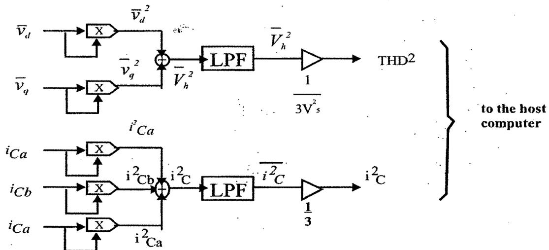
Fig 3.18: Voltage THD and Compensation Current Calculations
