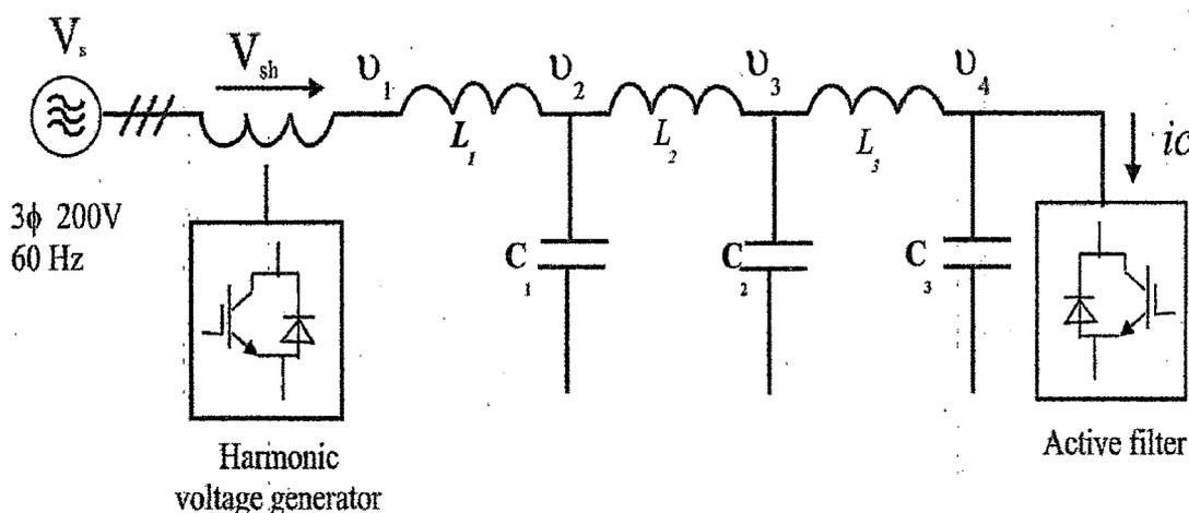
Fig 3.12: Three Phase distribution line Simulator
