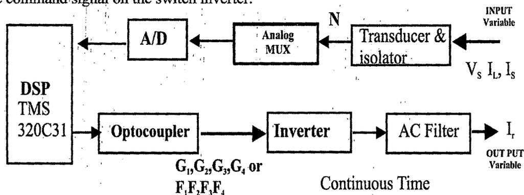
Fig 3.5 Block Diagram of Hardware setup for DSP Based APF
