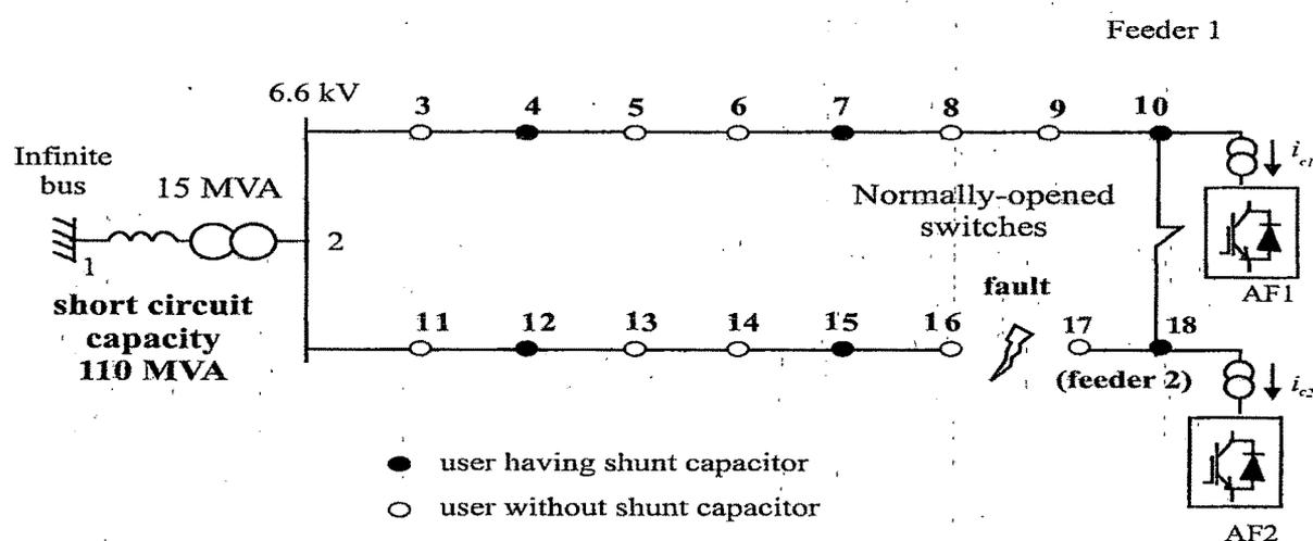
**Fig 3.17 A feeder Arrangement under a fault Condition**
