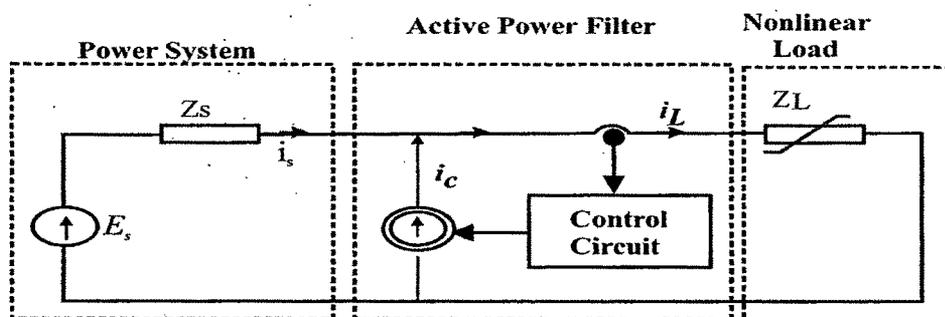
Fig 3.30 (a) Harmonic Compensation Circuit with current-fed APF without feedback (with unity gain)
