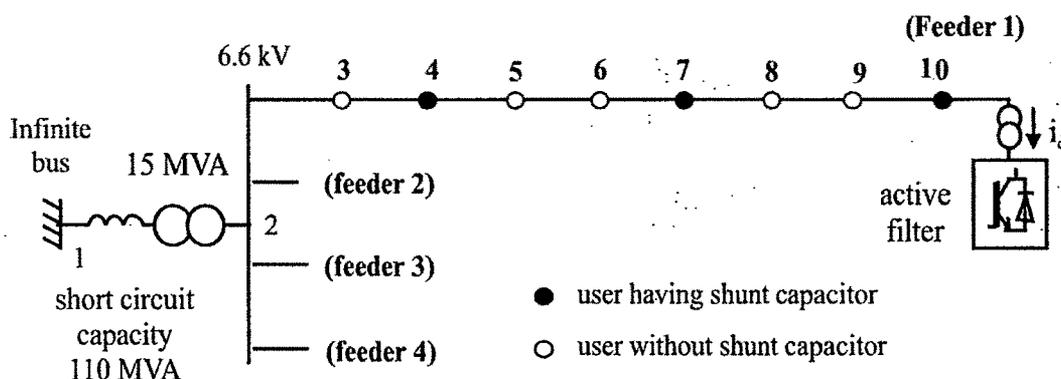
**Fig 3.16 A radial Power Distribution system**
