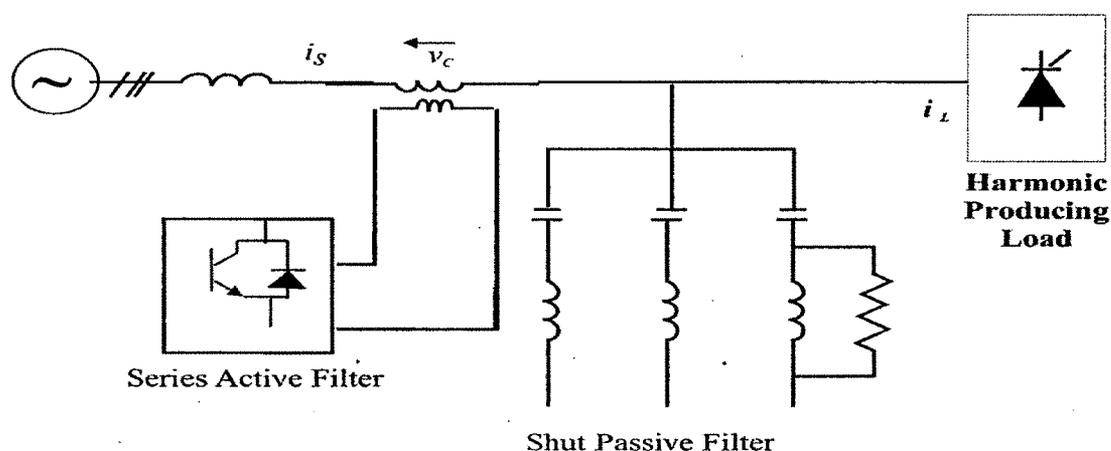
**Fig 3.1: Combination of Series Active and Passive Filters**
