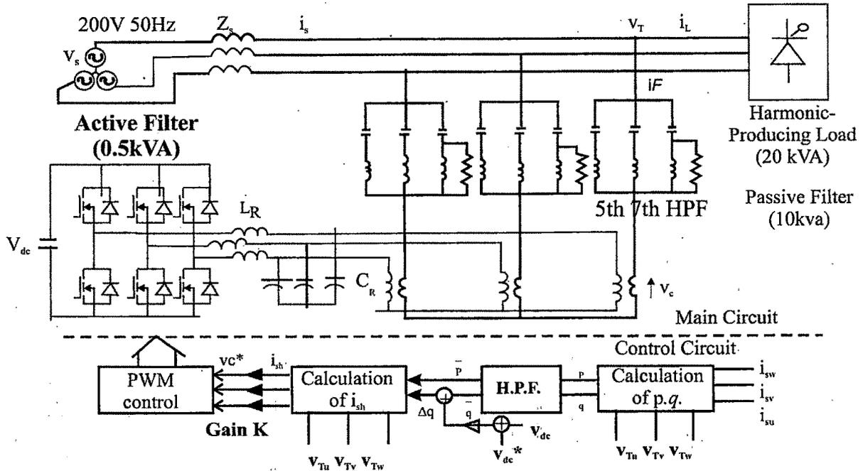
**Fig 3.2 Hybrid Series Configuration**
