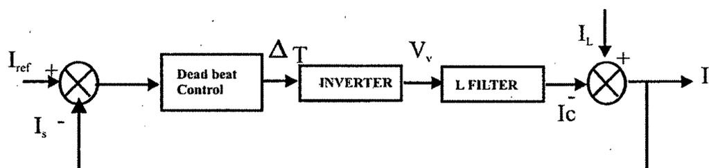
**Fig 3.3 Control Diagram of Shunt APF**
