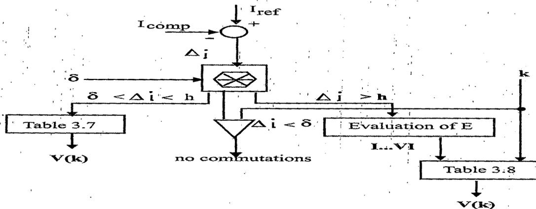
Fig 3.29 Current Control Scheme
