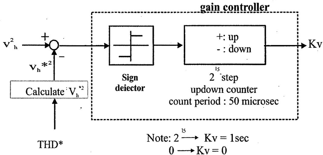
Fig 3.15: Software Implementation of Automatic Gain Adjustment
