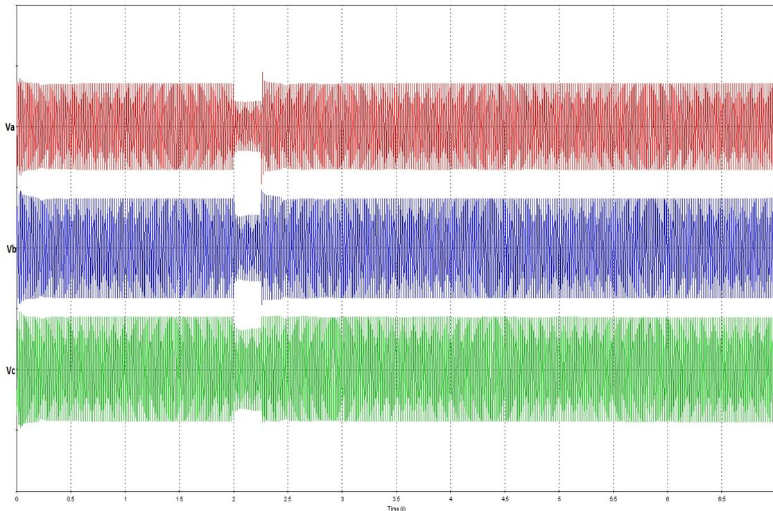
Figure 7.36: Wind Turbine Voltage during Fault
