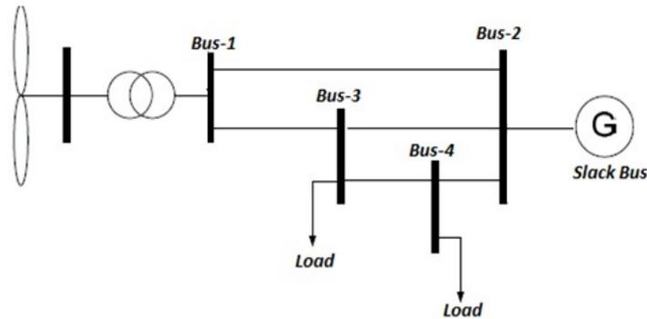
Figure 7.24: 4-Bus EPRI Test System
