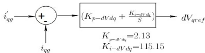
Figure 7.20: PI controller for  $dV_{qRef}$
