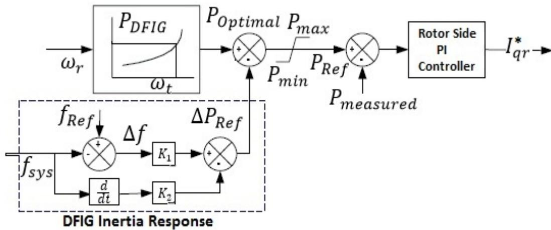
Figure 7.2: Primary Frequency Control
