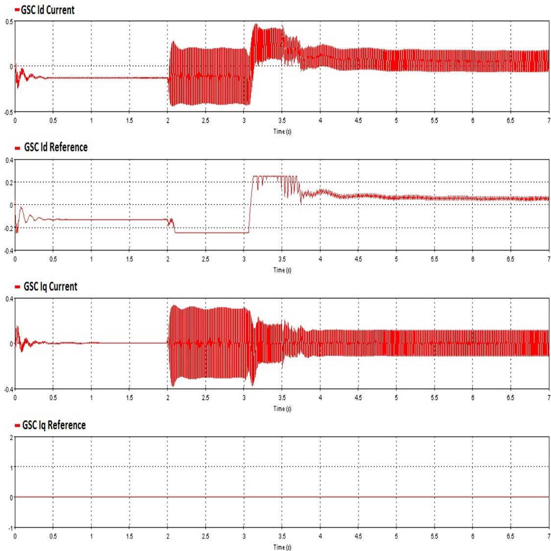
Figure 7.39: Grid Side Converter - Outer Loop Currents
