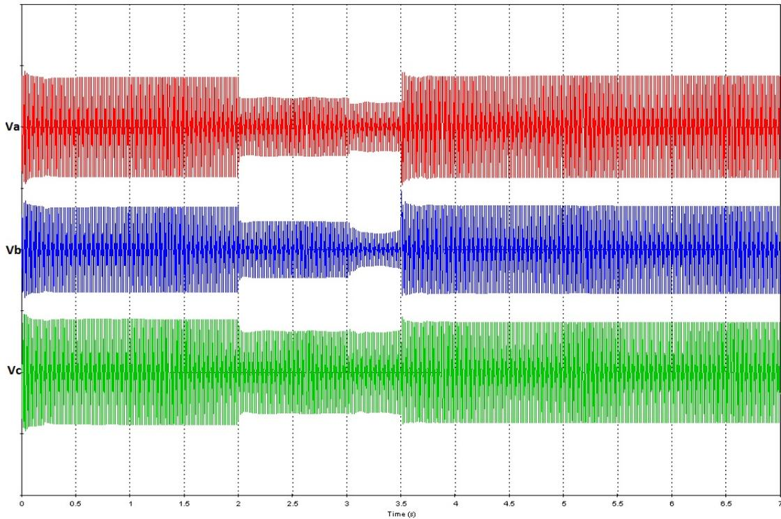
Figure 7.48: Wind Turbine Voltage during Fault
