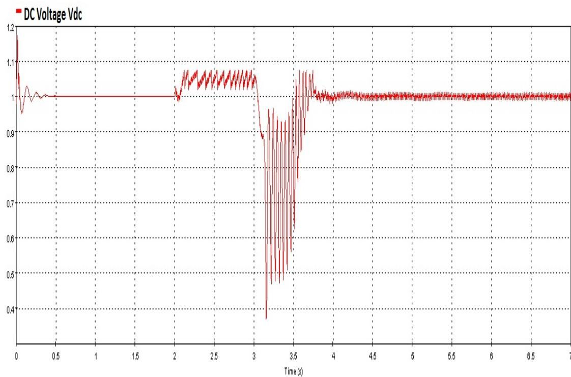
Figure 7.43: DC Link Voltage Deviation due to Fault
