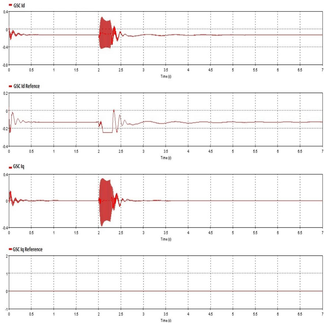
Figure 7.27: Grid Side Converter - Outer Loop Currents
