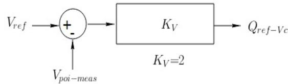
Figure 7.11: Reactive Power Reference for Voltage Control
