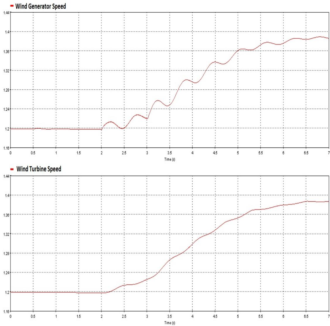
Figure 7.46: Wind Generator and Wind Turbine Speed Deviation during Fault
