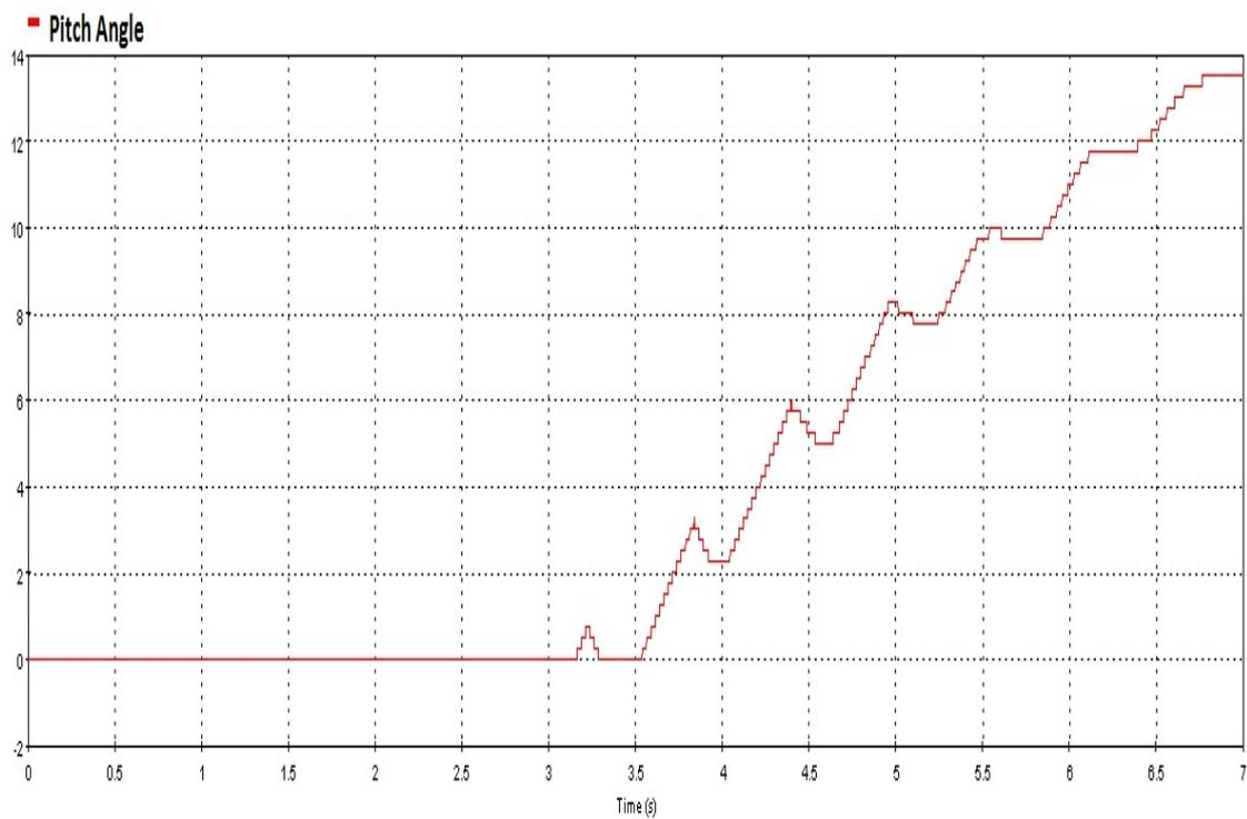
Figure 7.44: Pitch Angle Variation due to Fault
