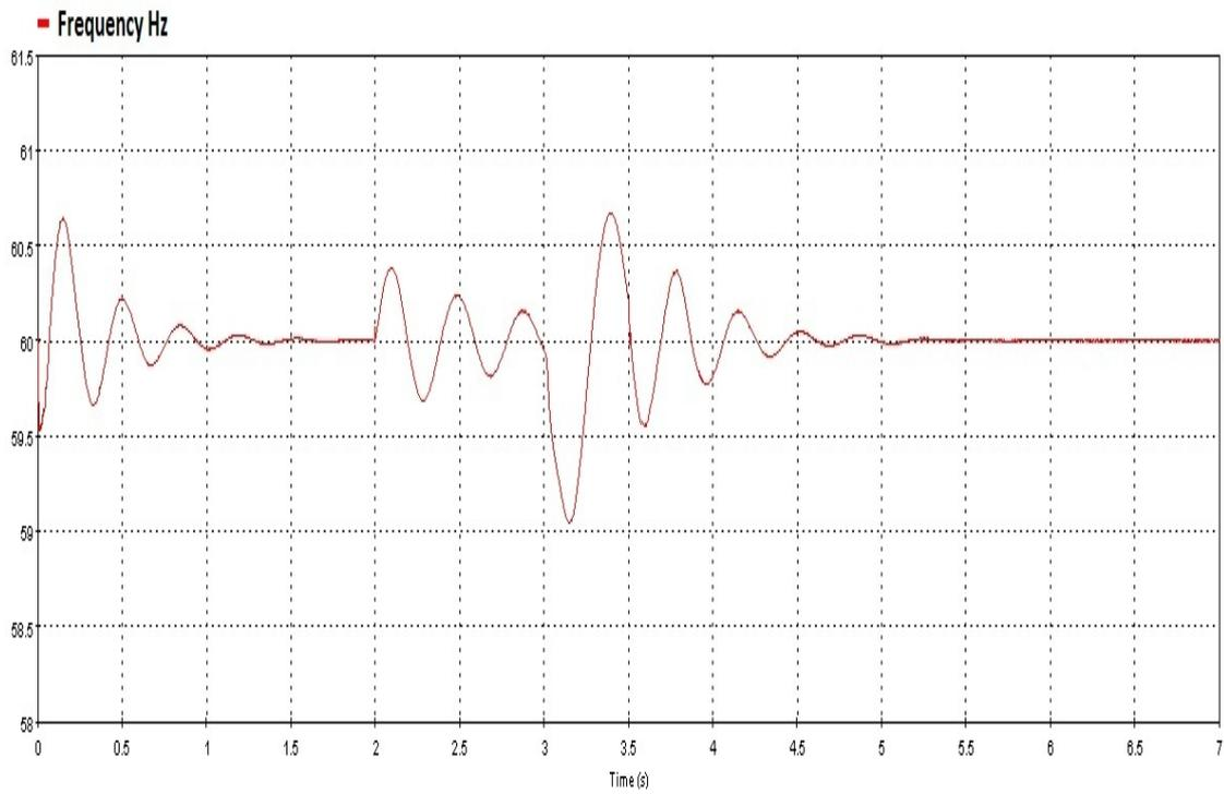
Figure 7.42: Frequency Deviation During Fault
