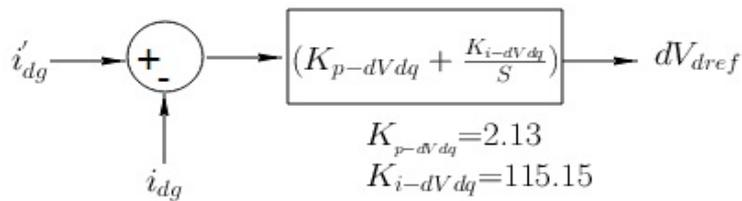
Figure 7.19: PI controller for  $dV_{dRef}$
