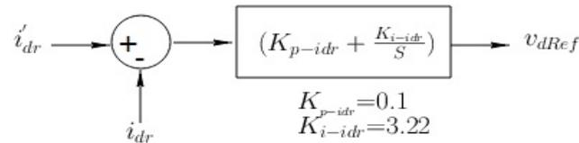
Figure 7.16: PI controller for  $v_{dRef}$
