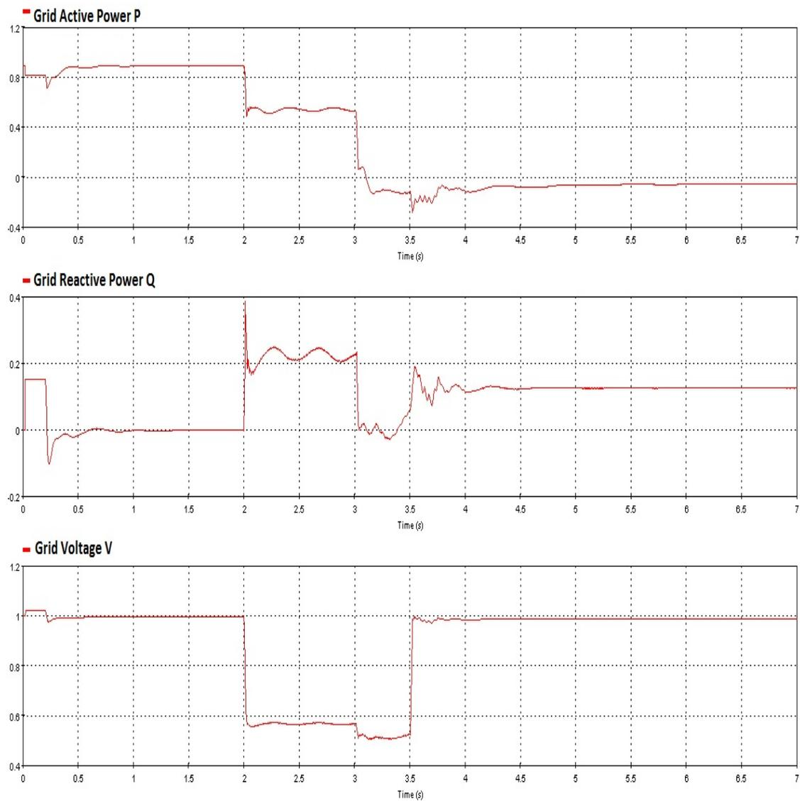
Figure 7.47: Grid Active Power, Reactive Power and Voltage during Fault
