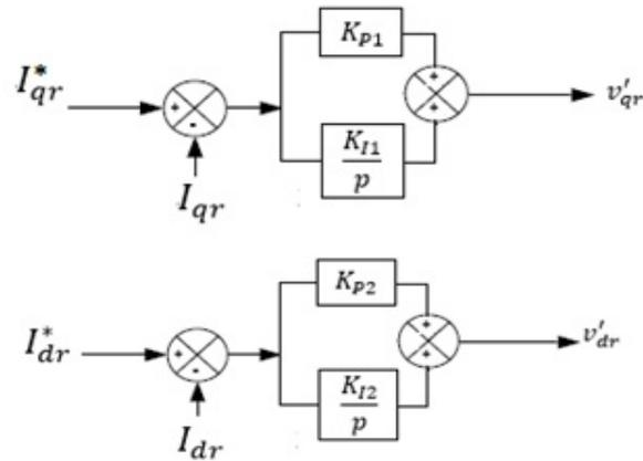
Figure 7.4: PI Controller for  $d$  and  $q$  axis
