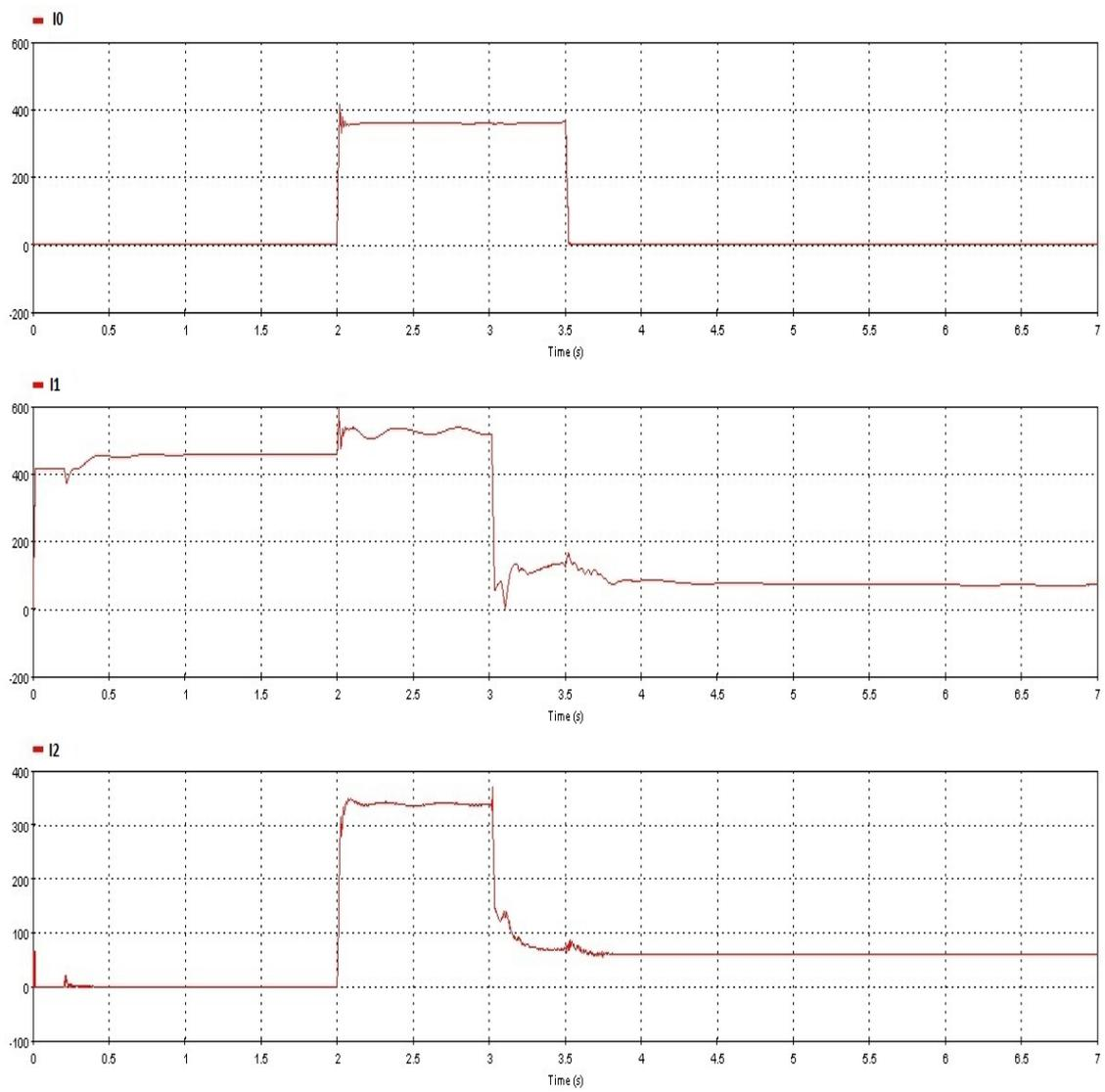
Figure 7.37: Positive, Negative and Zero Sequence Current Under Unbalance Condition
