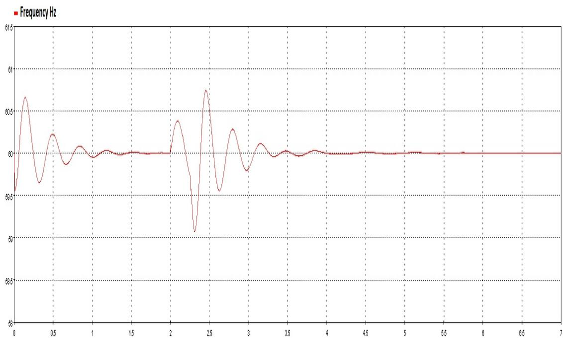
Figure 7.30: Frequency Deviation During Fault
