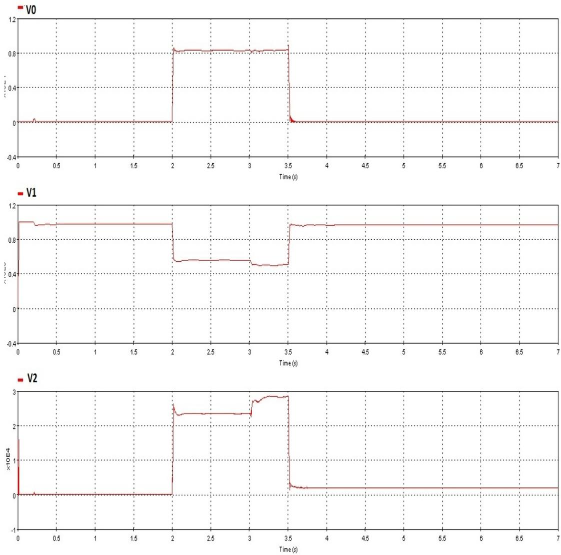
Figure 7.38: Positive, Negative and Zero Sequence Voltage Under Unbalance Condition
