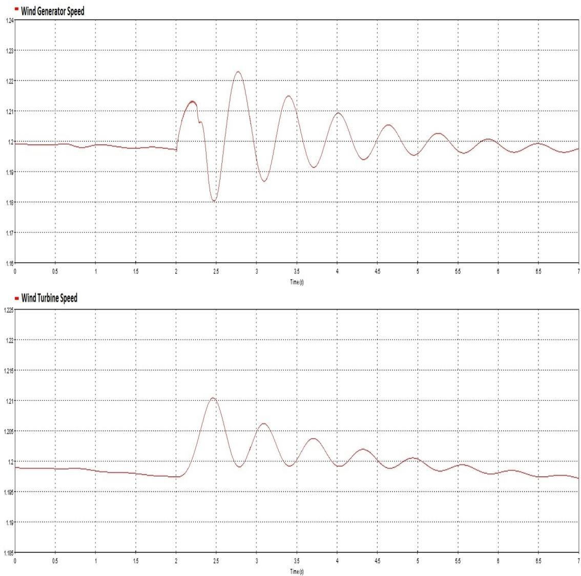
Figure 7.34: Wind Generator and Wind Turbine Speed Deviation during Fault
