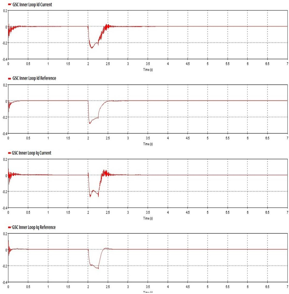
Figure 7.28: Grid Side Converter - Inner Loop Currents
