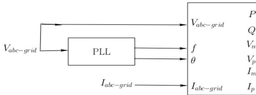
Figure 7.10: Measurement Block
