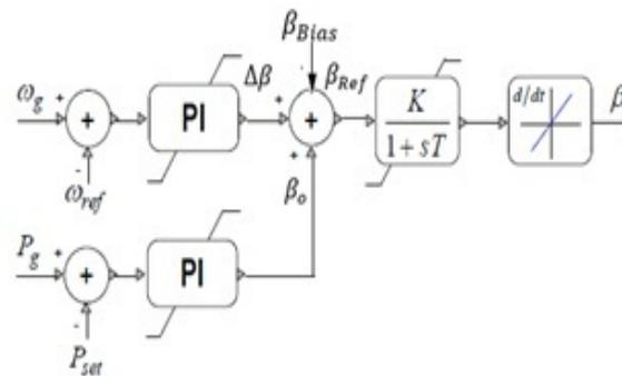
Figure 7.6: Pitch Control Loop
