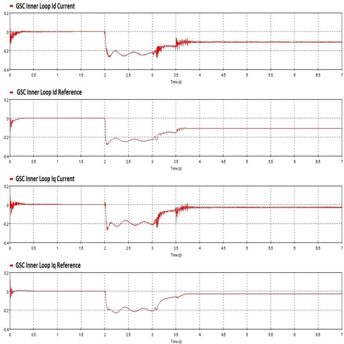
Figure 7.40: Grid Side Converter - Inner Loop Currents
