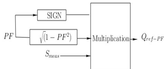
Figure 7.12: Reactive Power Reference for PF Control
