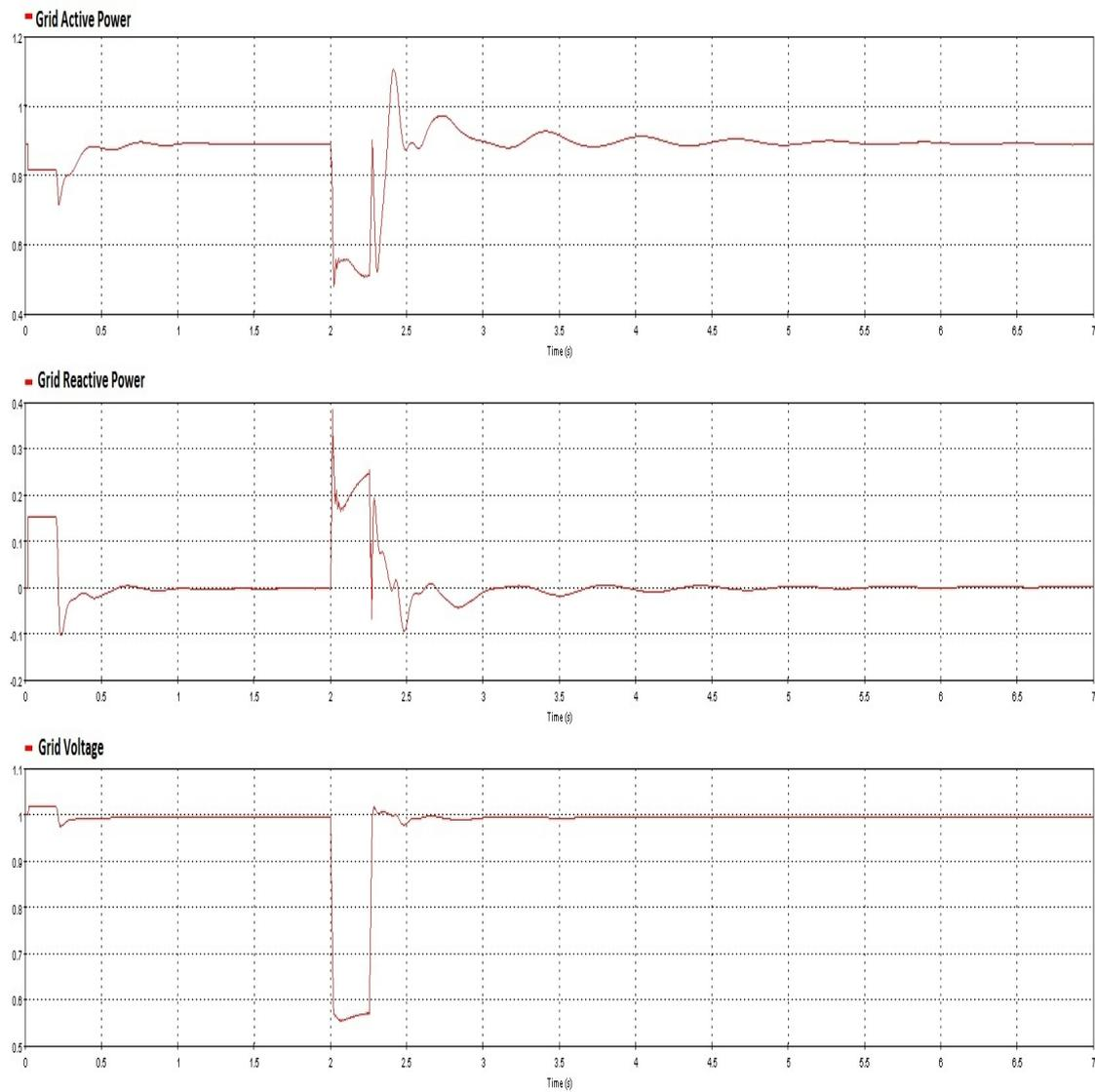
Figure 7.35: Grid Active Power, Reactive Power and Voltage during Fault
