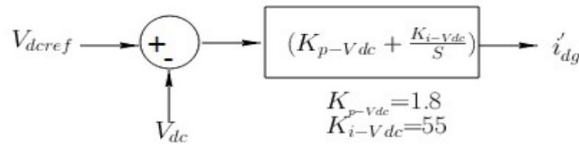
Figure 7.18: PI controller for DC Link Voltage Regulation
