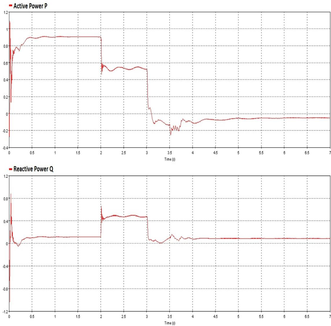
Figure 7.41: Active and Reactive Power of RSC during Fault
