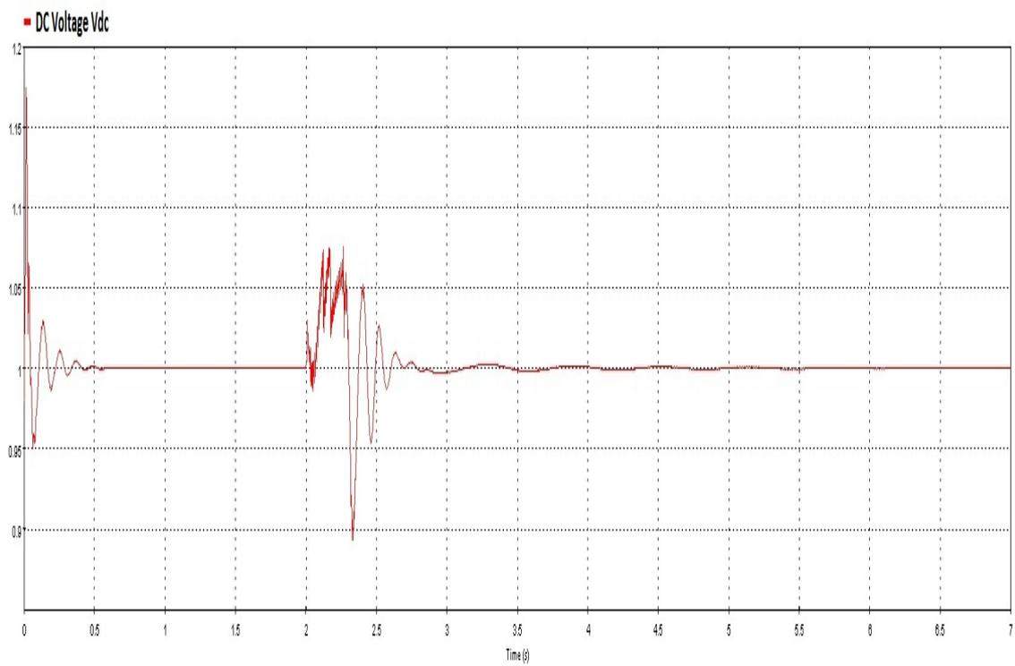
Figure 7.31: DC Link Voltage Deviation due to Fault
