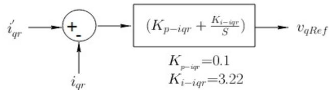
Figure 7.17: PI controller for  $v_{qRef}$
