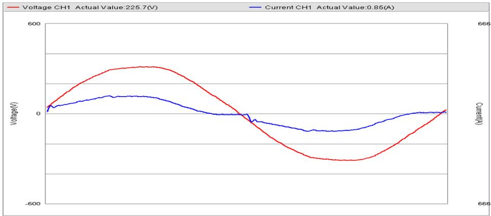
Figure 2.20 Voltage and current waveform (LCD projector)
