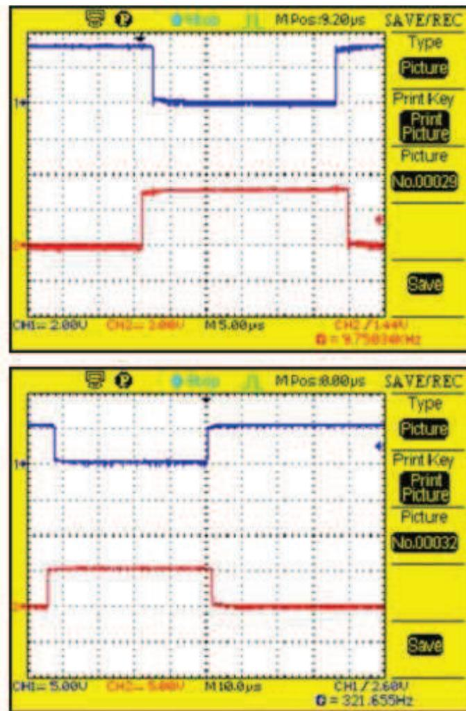
Figure 5.11: Control signals of 3.3 V & 5 V with dead time.
