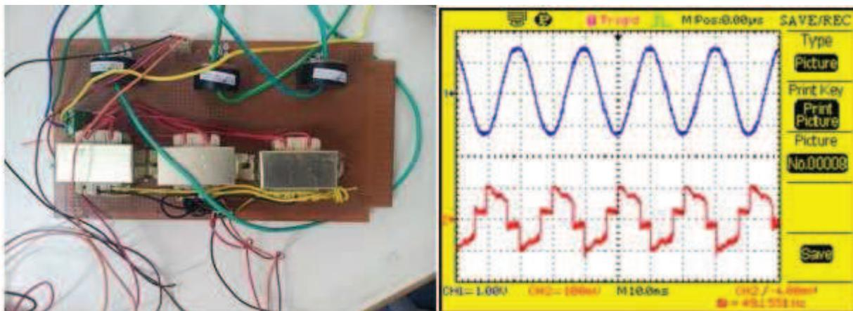
Figure 5.9: Current and voltage sensors CTs & PTs along with waveforms
