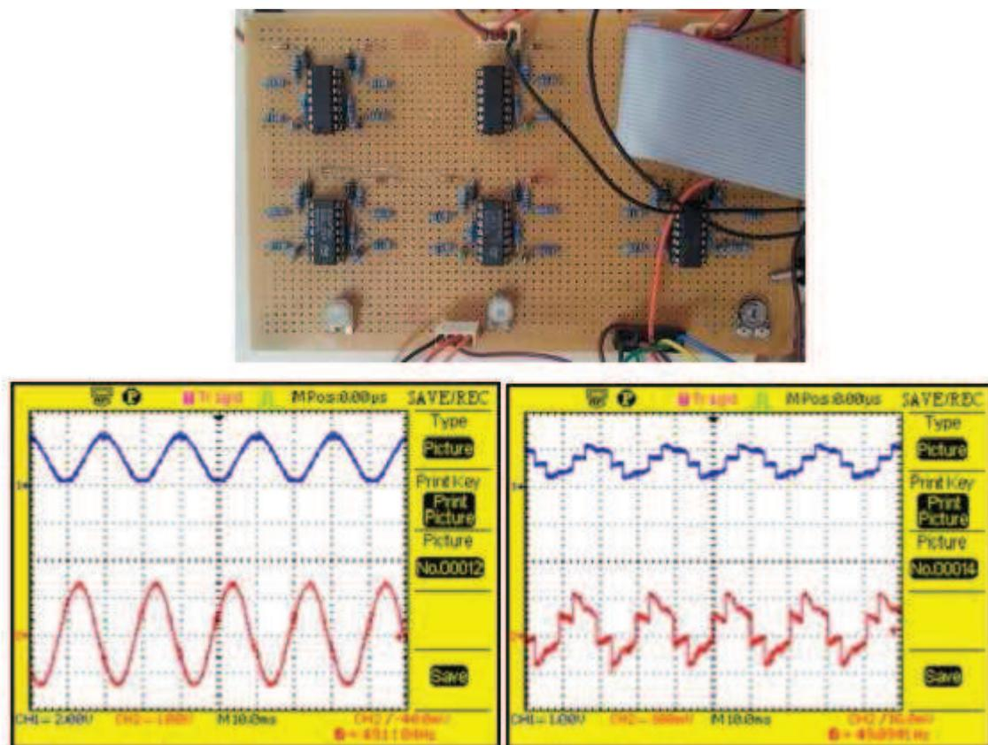
Figure 5.10: Signal conditioning circuit with waveforms
