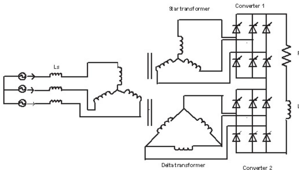
Figure 5.1: Power circuit diagram for 12 pulse converter
