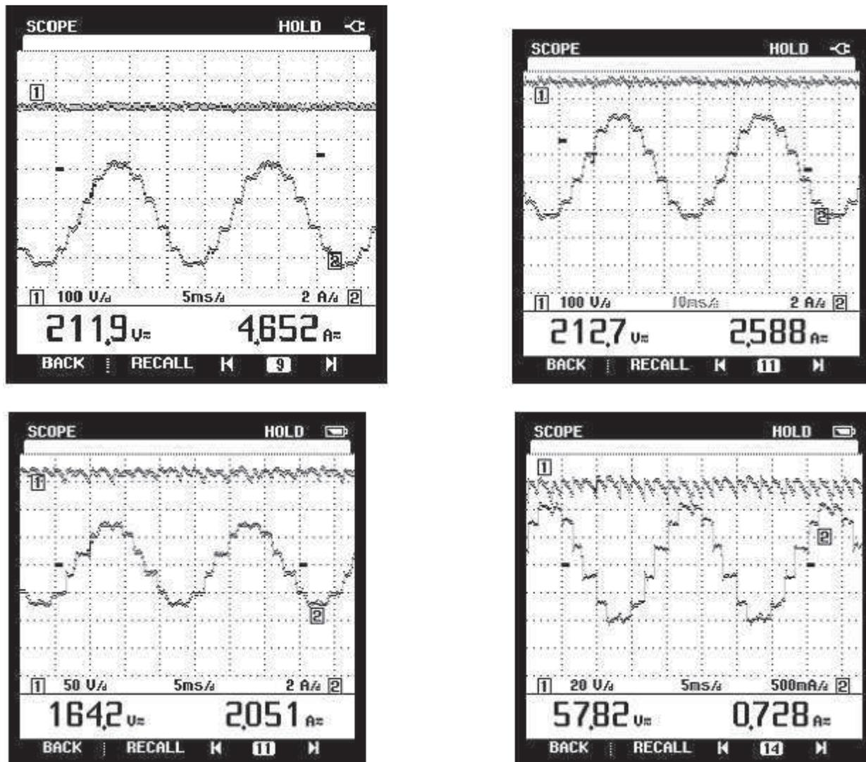
Figure 5.4: Equal firing angle mode
