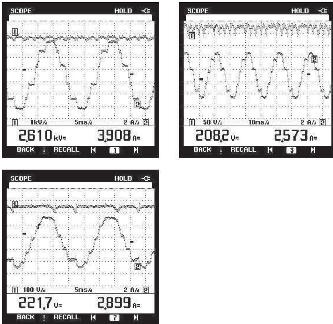
Figure 5.5: Unequal firing angle mode
