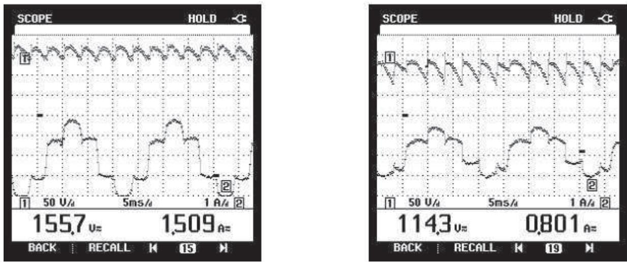
Figure 5.3: Six pulse converter star- delta connected
